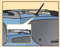
Note: The antenna mast may be laid down flat when carrying over-size objects such as skis or surfboards.
