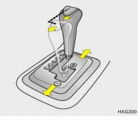
Whether the vehicle is stationary or in motion, sports mode is selected by pushing the selector lever from the "D" position into the manual gate. To return to "D" range operation, push the selector lever back into the main gate. In sports mode, moving the selector lever backwards and forwards can make rapid gearshifts simple. In contrast to a manual transaxle, the sports mode allows gearshifts with the accelerator pedal depressed.
