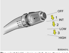
The windshield wiper switch has three positions:
