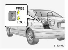
If the rear seatback lock lever (located on the backside of the rear seatback) is in the "LOCK" position when the rear seatbacks are closed, it will not be possible to fold the rear seatback by using the release lock lever. In this instance, move the lock lever to the "FREE" position and fold the rear seatback. The rear seatback lock lever is designed to provide protection from unauthorized entry into the trunk.
