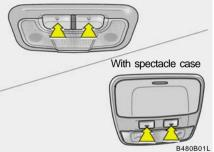
Push in the map light switch to turn the light on or off. This light produces a spot beam for convenient use as a map light at night or as a personal light for the driver and the passenger.
