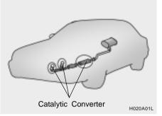
All Hyundai vehicles are equipped with a monolith type three-way catalytic converter to reduce the carbon monoxide, hydrocarbons and nitrogen oxides contained in the exhaust gas. Exhaust gases passing through the catalytic converter cause it to operate at a very high temperature. The introduction of large amounts of unburned gasoline into the exhaust may cause the catalytic converter to overheat and create a fire hazard. This risk may be reduced by observing the following:
