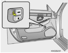
To open the trunk lid without using the key, pull up the lid release lever located on the driver's door panel.
