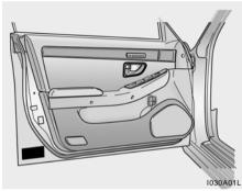
Tire label located on the driver's door edge gives the cold tire pressures recommended for your vehicle with the original tire size, the number of people that can be in your vehicle and vehicle capacity weight.
