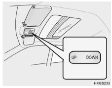
The sunroof can be tilted and closed with the ignition key in the "ON" position. Release the button when the sunroof reaches the desired position.
