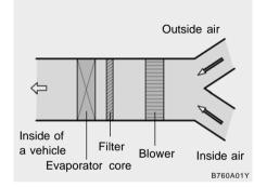
The air conditioner filter is located in front of the evaporator unit behind the glove box.
