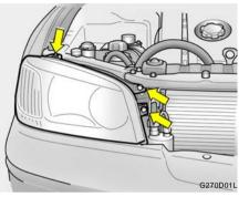
Using a socket wrench of the correct size, remove the headlight assembly mounting bolts.
