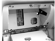
3. Lower the glove box down completely.
