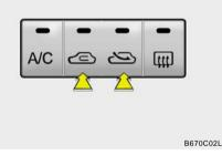
This is used to select fresh outside air or recirculating inside air.
