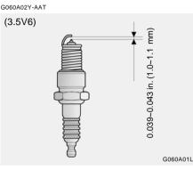
Your engine was originally equipped with platinum-tipped spark plugs.
