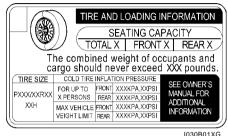
The tire label located on the driver's door edge gives the original tire size, cold tire pressures recommended for your vehicle, the number of people that can be in your vehicle and vehicle capacity weight.
