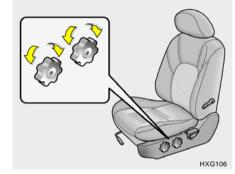
Move the front portion of the control knob up or down to raise or lower the front part of the seat cushion. Move the rear portion of the control knob up or down to raise or lower the rear part of the seat cushion.
