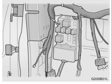
The instrument panel junction box for the lights and other electrical accessories will be found low on the dashboard on the driver's side. Inside instrument panel junction box you will find a list showing the circuits protected by each fuse. If any of your car's lights or other electrical accessories stop working, a blown fuse could be the reason. If the fuse has burned out, you will see that the metal strip inside the fuse has burned through. If you suspect a blown fuse, follow this procedure:
