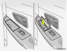
The rear ashtray may be opened by pulling the ashtray lid out. To remove the ashtray to eupty or clean it, lift the metal ash receptacle upward and pull it out.
