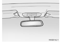
The electric type day/night inside rearview mirror automatically controls the glare of headlights of the car behind you. Adjust the rearview mirror to the desired position.
