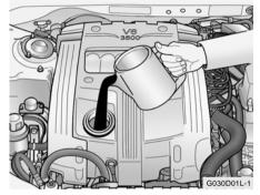
If the oil level is close to or below the "LOW" mark, add oil until it reaches the "FULL" mark.
