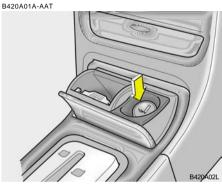
For the cigarette lighter to work, the key must be in the "ACC" position or the "ON" position. To use the cigarette lighter, push it all the way into its socket. When the element has heated, the lighter will pop out to the "ready" position. Do not hold the cigarette lighter pressed in. This can damage the heating element and create a fire hazard.
