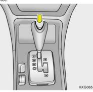
The highly efficient Hyundai automatic transaxle has five forward speeds and one reverse speed. The individual speeds are selected automatically, depending on the position of the speed selector lever. The selector lever has 2 gates; the main gate and the manual gate.
