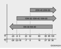
SH, SG or SG/CD (API) multi-grade and fuel efficient oil is recommended.
