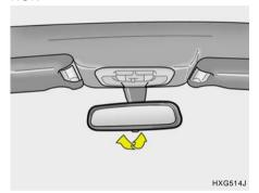
Your Hyundai is equipped with a day/night inside rear view mirror. The "night" position is selected by flipping the tab at the bottom of the mirror toward you. In the "night" position, the glare of headlights of cars behind you is reduced.
