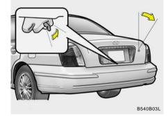
If the trunk lid lock knob (located near the latch) is in the "LOCK" position when the trunk lid is closed, it will not be possible to open the trunk lid by using the remote release. In this instance, use the master key to unlock and open the trunk lid.
