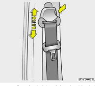
You can adjust the height of the shoulder belt anchor to one of the 4 positions for maximum comfort and safety.
