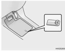
When using a floor mat on the front floor carpet, make sure it attaches to the floor mat anchor in your vehicle. This keeps the floor mat from sliding forward.
