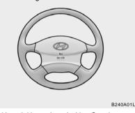
Your Hyundai is equipped with a Supplemental Restraint (Airbag) System. The indications of the system's presence are the letters "SRS AIRBAG" embossed on the airbag pad cover in the steering wheel and the passenger's side front panel pad above the glove box.
