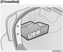
The CD Auto Changer is located in the left side of the trunk. This system can store up to 8 CDs. You may select music without changing disks. First, open the CD Auto Changer door, remove the CD "magazine", and insert up to 8 CDs. Then, push the magazine into the CD Auto Changer. The CD may be operated with the passenger compartment audio system controls.
