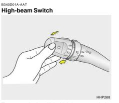
To turn on the headlight high beams, push the lever forward (away from you). The High Beam Indicator Light will come on at the same time. For low beams, pull the lever back toward you. B340E01A-AAT **Headlight Flasher**
