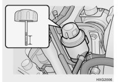
The power steering fluid level should be checked regularly.
