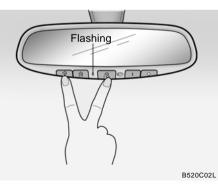
When programming the buttons for the first time, press and hold the two outside HomeLink buttons (介, 介), releasing when the indicator light begins to flash (approximately 20 seconds). This procedure erases the factory-set default codes. Do not perform this step when programming additional transmitters.
