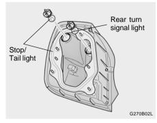
To replace the rear combination light (stop/ tail light and rear turn signal light), remove it from the bulb holder and install the new bulb.
