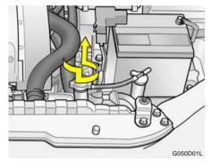
Turn the radiator cap counterclockwise without pressing down on it, until it stops. This relieves any pressure remaining in the cooling system. And remove the radiator cap by pushing down and turning counterclockwise.
