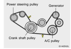
When the air conditioning is being used regularly, the compressor drive belt tension should be checked at least once a month with the engine turned off.
