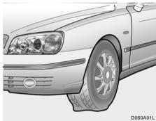
The procedure described on the following pages can be used to rotate tires as well as to change a flat tire. When preparing to change a flat tire, check to be sure the gear selector lever is in "P" and that the parking brake is set, then: Wheel Cap (If Installed)
