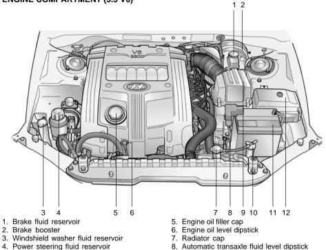
CAUTION: When inspecting or servicing the engine, you should handle tools and other heavy objects carefully so that the plastic cover of the engine is not damaged.
