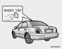
When the radio power switch is turned on while the ignition key is in either the "ON" or "ACC" position, your car will receive both AM and FM broadcast signals through the antenna in the rear window glass.
