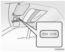
The sunroof can be electrically opened or closed with the ignition key in the "ON" position. To open or to close, press and hold the button located in the front of the roof panel. Release the button when the sunroof reaches the desired position.
