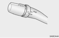
To operate the automatic light feature, turn the barrel on the end of the multi-function switch. If you set the multi-function switch to "AUTO", the tail lights and headlights will be turned automatically on or off according to external illumination.
