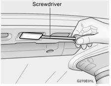
Remove the luggage compartment light cover on the rear package tray panel with a blade screwdriver.
