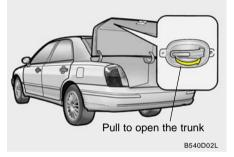
Your vehicle is equipped with a glow-in-the dark emergency trunk release lever located inside the trunk. It will glow after the trunk is closed. When pulled, this lever will release the trunk latch mechanism and open the trunk.
