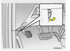
1. Pull the release knob to unlatch the hood.
