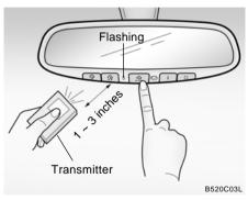
Hold the transmitter of the device you want to program 1 to 3 inches away from the bottom of the mirror. Simultaneously press the handheld transmitter button and the HomeLink button you wish to program. The indicator light will flash slowly at first, then rapidly, indicating successful programming.
