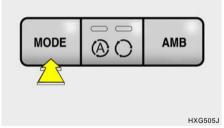
This is used to direct the flow of air. Air can be directed to the floor, dashboard outlets, or windshield. Four symbols are used to represent Face, Bi-Level, Floor and Floor-Defrost air position.
