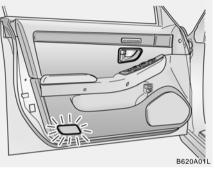
A red light comes on when the door is opened. The purpose of this light is to assist when you get in or out, and also to warn passing vehicles. B610A01Y-AAT
