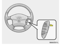
The vehicle will automatically resume the speed set prior to cancellation when you push the control switch "RESUME (ACCEL)" (above 25 mph).
