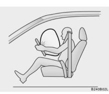
CAUTION: Do not install or place any accessories (drink holder, cassette holder, sticker, etc) on the front passenger's panel above the glove box in a vehicle with a passenger's air bag. Such objects may become dangerous projectiles and cause injury if the passenger's air bag inflates.
