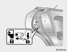
Your Hyundai is equipped with a "child-protector" rear door lock assembly. When the lock mechanism is engaged, the rear door cannot be opened from the inside. Its use is recommended whenever there are small children in the rear seat.
