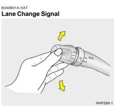
To indicate a lane change, move the lever up or down to a point where it begins flashing. The lever will automatically return to the center position when released. B340C02E-AAT Headlight Switch
