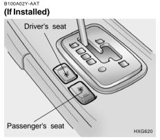
The seat warmer is provided to warm the front seats during cold weather. With the ignition key in the "ON" position, push either of the switches to warm the driver's seat or the passenger's seat.
