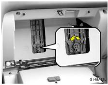
Turn the knob of the air conditioner filter cover counterclockwise and remove the air conditioner filter cover.
