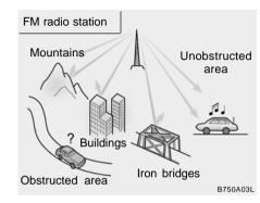
FM broadcasts are transmitted at high frequencies and do not bend to follow the earth's surface. Because of this, FM broadcasts generally begin to fade at short distances from the station. Also, FM signals are easily affected by buildings, mountains, or other obstructions. These can result in certain listening conditions which might lead you to believe a problem exists with your radio. The following conditions are normal and do not indicate radio trouble: 93
