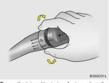
To use the intermittent wiper feature, place the wiper switch in the "INT" position. With the switch in this position, the interval between wipes can be varied from approximately 1 to 18 seconds by turning the interval adjuster barrel. This is also varied automatically depending on your road speed.
