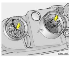
7. Disconnect the power cord from the bulb base in the back of the headlight.
