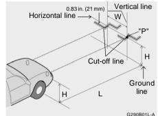
If the vehicle has had front body repair and the headlight assembly has been replaced, the headlight aiming should be checked using an aiming screen as shown in the illustration. Turn on the headlight switch. (Low Beam Position)
