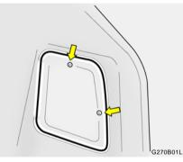
2. Remove the cover on the inside of rear luggage trim by unscrewing the screws.
