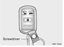
1. Carefully separate the case with a blade screwdriver as shown in the illustration.
