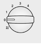
This is used to turn the blower fan on and off and to select the fan speed.
