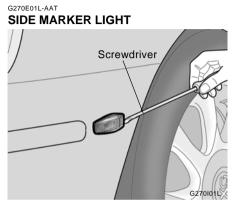
1. Remove the side marker light cover with a blade screwdriver.
