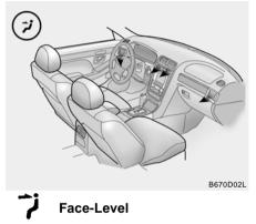
When selecting the "Face" mode, the indicator light will come on, causing air to be discharged through the face level vents.
