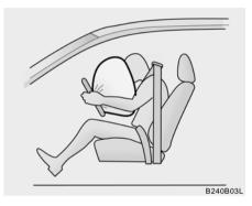
A fully inflated airbag in combination with a properly worn seat belt slows the driver's or the passenger's forward motion, thus reducing the risk of head or chest injury.
