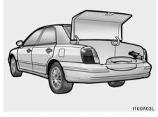
Remove the spare tire and take out the jack and tool bag from the trunk.
