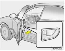
The doors can be locked without a key. To lock the doors, first push the inside lock switch to the "LOCK" position so that the red mark on the switch is not visible, then close the door. The door will not lock if the key is left in the ignition switch when the front doors close. This is normal.
