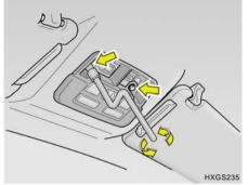
2. Remove the front overhead light and switch panel.
