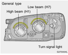
6. Turn the plastic cover counterclockwise and remove it.
