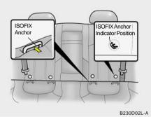
The ISOFIX anchors are located between the seatback and the seat cushion of the rear seat left and right outboard seating positions. Follow the child seat manufacturer's instructions to properly install safety seats with ISOFIX or ISOFIX-compatible attachments.
