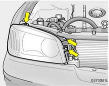
1. Remove the headlight assembly mounting bolts.
