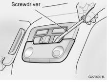
1. Remove the plastic cover with a flat blade screwdriver.
