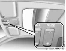
The sunroof can be electrically opened or closed with the ignition key in the "ON" position. The sunroof is moved to its fully open position by pushing the "1" switch, and to stop at the desired position, push in any switches ( $\uparrow$ ,  $\clubsuit$ , Up, Down). To close, press and hold the " I button. Release the button when the sunroof reaches the desired position.
