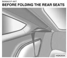
In order to prevent the shoulder belt from being damaged while folding the rear seat, the shoulder belt must be passed through the hanger to keep it out of the way.
