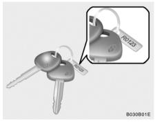
A code number is stamped on the key number plate that came with the keys to your Hyundai. This key number plate should be kept in a safe place, not in the vehicle. The key number should also be recorded in a place where it can be found in an emergency.
