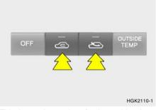
This is used to select fresh outside air or recirculation inside air.
