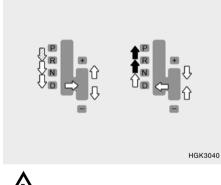
CAUTION: Never shift into "R" or "P" position while the vehicle is moving.
