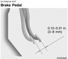
With the engine off, press down on the brake pedal several times to reduce the vacuum in the brake booster.
