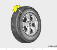
The wheel nuts should be loosened slightly before raising the car. To loosen the nuts, turn the wrench handle counterclockwise. When doing this, be sure that the socket is seated completely over the nut so it cannot slip off. For maximum leverage, position the wrench so the handle is to the left as shown in the drawing. Then, while holding the wrench near the end of the handle, push down on it with steady pressure. Do not remove the nuts at this time. Just loosen them about one-half turn.
