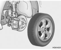
Loosen the wheel nuts and remove them with your fingers. Slide the wheel off the studs and lay it flat so it cannot roll away. To put the wheel on the hub, pick up the spare tire, line up the holes with the studs and slide the wheel onto them. If this is difficult, tip the wheel slightly and get the top hole in the wheel lined up with the top stud. Then jiggle the wheel back and forth until the wheel can be slid over the other studs.
