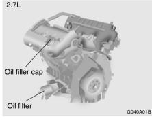
The engine oil and filter should be changed at those intervals specified in the maintenance schedule in Section 5. If the car is being driven in severe conditions, more frequent oil and filter changes are required.
