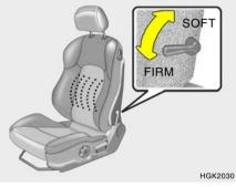
The driver's seat is equipped with adjustable lumbar support.
