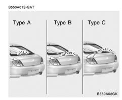
In addition to the lower-mounted rear stoplights on either side of the car, the high mounted rear stoplight in the center of the rear window or inserted in the rear spoiler also lights when the brakes are applied.
