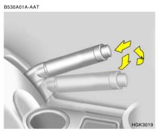
Always engage the parking brake before leaving the car. This also turns on the parking brake indicator light when the key is in the "ON" or "START" position. Before driving away, be sure that the parking brake is fully released and the indicator light is off.
