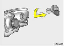
11.To replace the front turn signal light bulb, remove from the bulb holder and install the new bulb.
