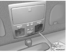
1. Remove the cover with a flat-blade screwdriver.
