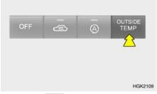
Pressing the  $\begin{bmatrix} OUTSDE\\TEMP \end{bmatrix}$  button displays the ambient temperature on the display.
