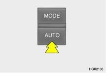
The FATC (Full Automatic Temperature Control) system automatically controls heating and cooling as follows:
