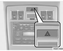
The hazard warning system should be used whenever you find it necessary to stop the car in a hazardous location. When you must make such an emergency stop, always pull off the road as far as possible.
