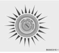
Whenever a door is opened, the ignition switch will be illuminated for your convenience, provided the ignition switch is not in the "ON" position.
