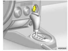
Park the car on level ground with the parking brake engaged. When the transaxle fluid level is checked, the transaxle fluid should be at normal operating temperature and the engine idling.
