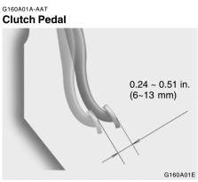
With the engine off, press lightly on the clutch pedal until you feel a change in resistance. This is the clutch pedal free-play. The free-play should be within the limits specified in the illustration. If it is not, have it inspected by your Hyundai dealer and adjusted or repaired if necessary.
