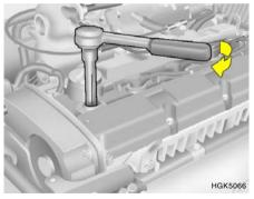
You will find it easier to change spark plugs if the engine is cold. Always change one spark plug at a time. This helps avoid getting the wires mixed up.
