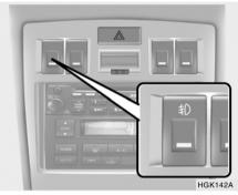
To turn on the front fog lights, push the switch. They will light when the headlight switch is in the second position and the ignition key is in the "ON" position.
