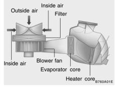
The air conditioner filter is located in front of the blower uniit behind the glove box.
