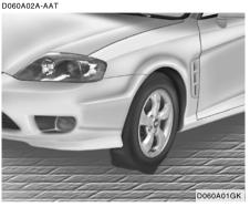
The procedure described on the following pages can be used to rotate tires as well as to change a flat tire. When preparing to change a flat tire, check to be sure the gear selector lever is in "P" (automatic transaxle) or reverse gear (manual transaxle) and that the parking brake is set, then:
