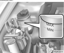
The power steering fluid level should be checked regularly. To check the power steering fluid level, be sure the engine is "OFF", then check to make certain that the power steering fluid level is between the "MAX" and "MIN" level markings on the fluid reservoir.
