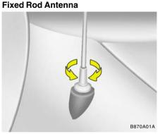
Your car uses a fixed rod antenna to receive both AM and FM broadcast signals. This antenna is a removable type. To remove the antenna, turn it counterclockwise. To install
