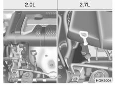
Before checking the oil, warm up the engine to the normal operating temperature and be sure your car is parked on level ground. Turn the enaine off.
