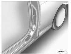
Tire label located on the driver's side of the center pillar outer panel gives the cold tire pressures recommended for your vehicle with the original tire size, the number of people that can be in your vehicle and vehicle capacity weight.
