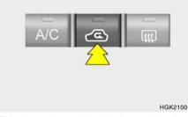
This is used to select fresh outside air or recirculating inside air.
