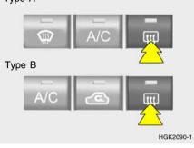
The rear window defroster and heated outside rearview mirrors are turned on by pushing in the switch. To turn the defroster off, push the switch a second time. The rear window defroster automatically turns itself off after about 15 minutes. To restart the defroster cycle, push in the switch again after it has turned itself off.
