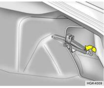
The jack is located behind the right side of luggage trim. Remove the jack cover by unscrewing the bolts. Turn the jack end counterclockwise to lower the jack height by using a screw driver or wrench bar and remove it from the bracket.
