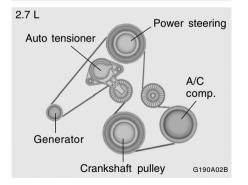
When the air conditioning is being used regularly, the compressor drive belt tension should be checked at least once a month with the engine turned off.
