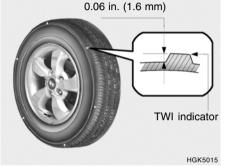
The original tires on your car have tread wear indicators. The location of tread wear indicators is shown by the "TWI" or "  $\triangle$  " marks, etc., The tread wear indicators appear when the tread depth is 0.06 in. (1.6 mm). The tire should be replaced when these appear as a solid bar across two or more grooves of the tread. Always replace your tires with those of the recommended size. If you change wheels, the new wheel's rim width and offset must meet Hyundai specification.
