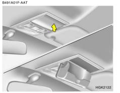
The spectacle case is located on the front overhead console.
