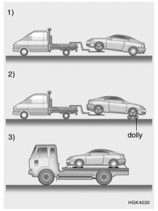
Your vehicle can be towed by wheel lift type truck (1), (2) or flatbed equipment (3).
