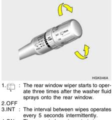
4.ON : The rear window wiper starts to operate continuously.
