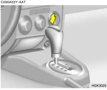
The highly efficient Hyundai automatic transaxle has four forward speeds and one reverse speed. The individual speeds are selected automatically, depending on the position of the speed selector lever. The selector lever has 2 gates; the main gate and the manual gate.
