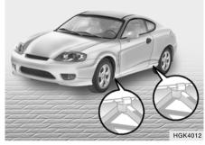
The base of the jack should be placed on firm, level ground. The jack should be positioned as shown in the drawing. **5. Raising the Car**
