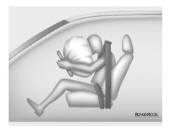
A fully inflated airbag in combination with a properly worn seat belt slows the driver's or the passenger's forward motion, thus reducing the risk of head and chest injury.
