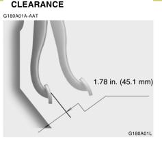
CHECKING BRAKE PEDAL
