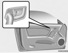
The central door locking is operated by pushing the driver's door lock switch toward the front or
