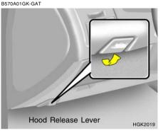
1. Pull the release knob to unlatch the hood.
