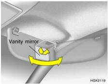
Your Hyundai is equipped with sun visors to give the driver and front passenger either frontal or sideward shade. To reduce glare or to shut out direct rays of the sun, turn the sun visor down. A vanity mirror is provided on the back of the sun visor for the front passenger.
