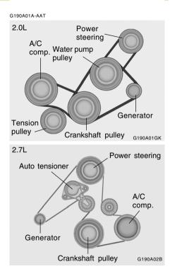
Drive belts should be checked periodically for proper tension and adjusted if necessary. At the same time, belts should be examined for cracks, wear, fraying or other evidence of deterioration and replaced if necessary.
