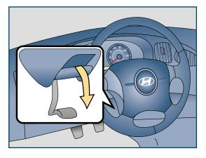
To adjust the steering wheel tilt, lower the lock lever and raise or lower the steering wheel to a comfortable position. Fully raise the lock lever to maintain desired setting.
