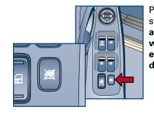
Pressing the lock switch deactivates all of the power window switches except for the driver's window.
