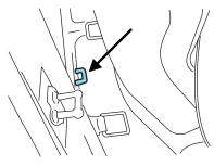
3. Route the child safety seat tether strap through the openings on top of the seatback.
