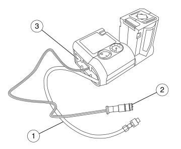
1. Remove the hose (1) and the cable with the electrical plug (2) from the kit's storage compartment (3).
