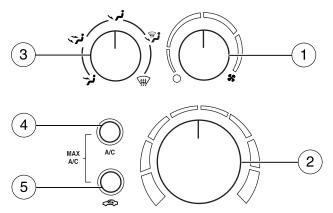
1. **Fan speed adjustment:** Controls the volume of air circulated in the vehicle.
