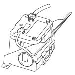
For longer, trouble-free operation, keep the top of the battery clean and dry. Also, make certain the battery cables are always tightly fastened to the battery terminals.
