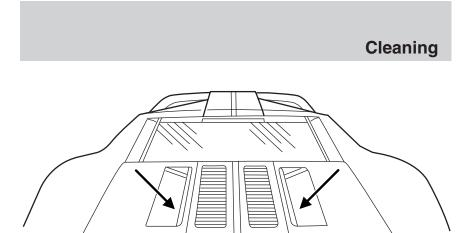
• Do not let excess water drain into the engine air intakes located on the engine cover.
