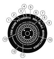
7. **H**: Indicates the tire's speed rating. The speed rating denotes the speed at which a tire is designed to be driven for extended periods of time under a standard condition of load and inflation pressure. The tires on your vehicle may operate at different conditions for load and inflation pressure. These speed ratings may need to be adjusted for the difference in conditions. The ratings range from 81 mph (130 km/h) to 186 mph (299 km/h). These ratings are listed in the following chart.
