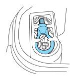
The tow hook should be threaded into the hole provided in the front grill area as shown. **Note: This is a left-handed thread.**
