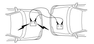
4. Make the final connection of the negative (-) cable to the negative (-) battery terminal of the stalled vehicle.
