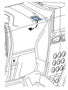
2. Lift up on the decklid at the side air scoop area to provide better access to the auxiliary release.
