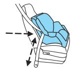
10. Try to pull the belt out of the retractor to make sure the retractor is in the automatic locking mode (you should not be able to pull more belt out). If the retractor is not locked, unbuckle the belt and repeat steps two through nine.
