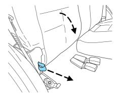
6. Rotate seatback down into load floor position.
