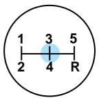
**NOTE:**You can shift into R (Reverse) only by moving the gearshift lever from left of 3 (Third) and 4 (Fourth) gears before you shift into R (Reverse). This is a special lockout feature which prevents you from shifting into R (Reverse) when you downshift from 5 (Fifth).
