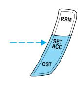
**NOTE:**You can accelerate with the accelerator pedal at any time during speed control usage. Releasing the accelerator pedal will return your vehicle to the previously programmed set speed.
