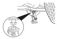
• Rear jacking notches are located under the rear trailing arm.
