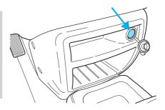
The auxiliary power point is located on the instrument panel below the radio.
