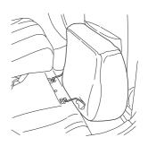
5. Pull the seatback release strap toward the front seat. Make sure the seat belt buckle heads are fully extended towards the front of the vehicle and are away from the seatback.
