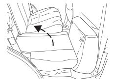
2. Rotate seat cushion down into the seating position making sure that the seat cushion is locked into place and that the seat belt buckles are exposed.
