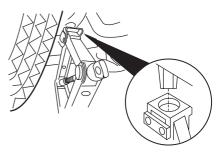
6. Position the jack according to the following guides and turn the jack handle clockwise until the tire is a maximum of 25 mm (1 inch) off the ground.
