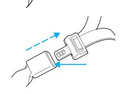
The front and rear outboard safety restraints in the vehicle are combination lap and shoulder belts. The front passenger and rear seat outboard safety belts have two types of locking modes described below:
