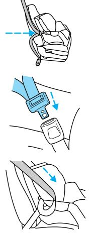
6. Allow the belt to retract. The belt will click as it retracts to indicate it is in the automatic locking mode.
