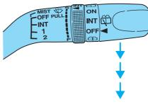
To activate the windshield washer, pull control toward you. Release control to stop washer fluid spray.
