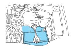
However, for severe usage or in high temperature climates, check the battery electrolyte level. Refer to the service maintenance section for the service interval schedules.
