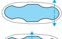
Move the control in the directions shown to move the seat forward, backward, up or down.
