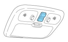
$\bullet\,$  To close, press and hold the front portion of the control.
