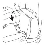
3. Remove the head restraints stored under the front passenger seat and return them to the original position on the seat backs.
