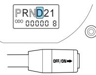
shift into fourth gear. Operating in D (O/D OFF) provides more engine braking than Overdrive for descending hills or city driving.
