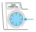
If the volume is set above a certain level and the ignition is turned off, the volume will come back on at a "nominal" listening level when the ignition switch is turned back on.
