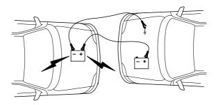
4. Make the final connection of the negative (-) cable to an exposed metal part of the disabled vehicle's engine, away from the battery and the fuel injection system. **NOTE: Do not** use fuel lines, engine rocker covers or the intake manifold as *grounding* points.
