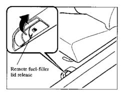
To open, pull up the remote fuel-filler lid release.
