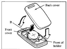
3. Install a new battery (CR2025 or the equivalent) into the front portion of the holder with the positive pole (+) facing up. Press on the B portion of the battery to set the battery.
