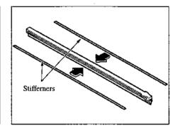
Remove the metal stiffeners from the blade rubber and install them in new blades.
