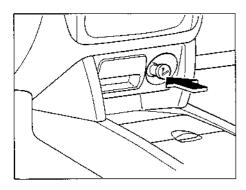
To operate the lighter, press it in and release it. When ready for use, it automatically pops out.
