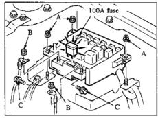
When replacing the 100A fuse:
