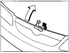
2. Pull the safety catch up and lift the hood.
