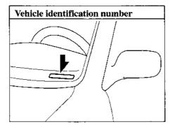
The vehicle identification number legally identifies your vehicle. The number is on a plate attached to the left top side of the dashboard. This plate can easily be seen through the windshield.
