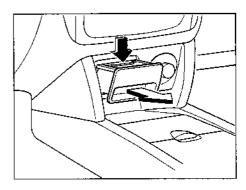
To remove, open and push down on the lock spring.
