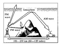
Signals from an FM transmitter are similar to beams of light because they do not bend around corners, but they do reflect. Unlike AM signals, FM signals cannot travel beyond the horizon. Therefore, FM stations cannot be received at the great distances possible with AM reception.
