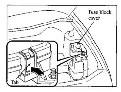
If the headlights or other electrical components don't work and the fuses in the cabin are OK, inspect the fuse block under the hood. If a fuse is blown, it must be replaced. Follow these steps:
