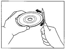
A new CD may have rough edges on its inner and outer perimeters. If a disc with rough edges is used, proper setting will not be possible and the CD player/changer will not play the CD. Remove the rough edges in advance by using a ball-point pen or pencil as shown above. To remove the rough edges, rub the side of the pen or pencil against the inner and outer perimeter of the CD.
