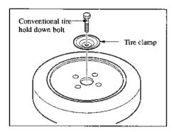
15. Store the damaged tire, using the conventional tire hold-down bolt supplied in the tool bag to hold it in place. Turn the tire clamp upside down from the temporary spare tire position. Repair the damaged tire and replace the spare with it as soon as possible.
