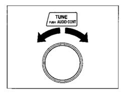
2. Turn the audio control knob to adjust the selected function; bass, mid-range, treble, fade or balance.
