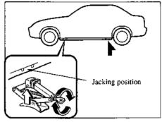
Place the jack under the jacking position closest to the tire being changed.
