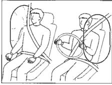
The air bags will function only once. After that, the air bags will not work again and must be replaced.
