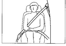
Adjust the height of the shoulder belt if the seat belt touches your neck, if it crosses your arm instead of your shoulder. To raise the shoulder belt adjuster, push the adjuster up. To lower the shoulder belt adjuster, push the button slide it down. Make sure the adjuster is locked.
