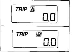
When trip meter A is selected, TRIP A will be displayed. When meter B is selected, TRIP B will be displayed.
