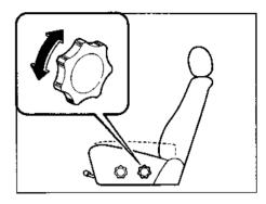
The seat-bottom angle can be adjusted by rotating the dial. The rear dial tilts the rear of the seat bottom upward.
