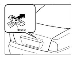
To open the trunk lid from the inside, pull the illuminated "T" shaped handle. The handle is made of material that will glow for hours in the darkness of the trunk following a brief exposure to ambient light.
