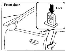
To lock any door with the door-lock button from the outside, push down the door-lock button and close the door.
