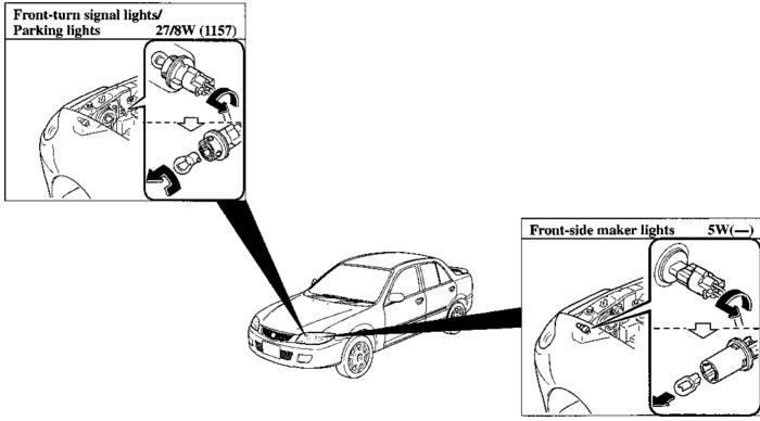
To replace the fog light bulbs, contact an Authorized Mazda Dealer. The number in ( ) shows the bulb number.
