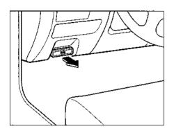
1. With the vehicle parked, pull the release handle to unlock the hood.
