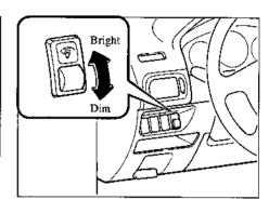
When the parking lights or headlights are on, rotate the thumb-wheel to adjust the brightness of the dashboard lights.
