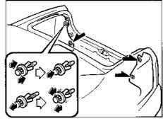
Remove the inside cover's plastic retainers and partially open the inside cover.
