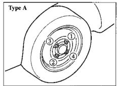
14. Turn the jack handle counterclockwise and lower the vehicle. Use the lug wrench to tighten the nuts in the order shown.
