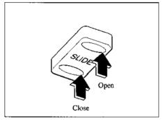
To open to any position, press the rear of the slide switch located on the right side of the overhead console.
