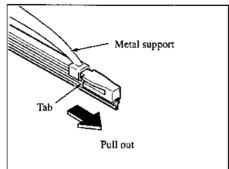
3. Hold the end of the rubber and puil until the tabs are free of the metal support.
