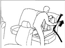
2. To get the retractor into the automatic locking mode, pull the shoulder belt portion of the seat belt until the entire length of the belt is out of the retractor. Push the child-restraint system firmly into the vehicle seat. Be sure the belt retracts as snugly as possible. Clicking from the retractor will be heard during retraction if the system is in the automatic locking mode. If the belt does not lock the seat down tight, repeat this step.
