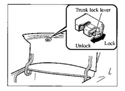
To secure the trunk lid, lock the rear seatbacks (page 2-8), push the trunk lock lever up, and close the trunk.
