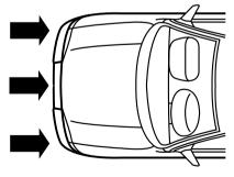
cause activation. Air bags are designed to inflate in frontal and near-frontal collisions, not rollover, side-impact, or rear-impacts unless the collision causes sufficient longitudinal deceleration.
