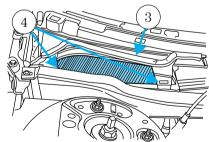
5. Remove the filter. Reverse the procedure to install the new filter.
