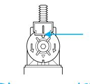
Turning the horizontal adjusting screw in the direction of the arrow changes the horizontal aim as shown.
