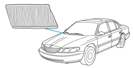
The cabin air filter restricts the entry of airborne dust and pollen particles. The filter is located just in front of the windshield under the cowl vent screen on the passenger side of the vehicle.
