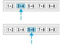
After the factory-set code or personal code has been entered, you can unlock all doors (press 3/4) and release the trunk (press 5/6) as long as the controls are pressed within five seconds of each other.
