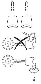
and devices cannot damage the **coded key** ignition key, but can cause a momentary issue if they are too close to the key during engine start. If a problem occurs, turn ignition OFF and restart the engine with all other objects on the key ring held away from the ignition key. Check to make sure the **coded key** ignition key is an approved Ford **coded key** ignition key.
