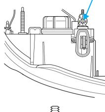
3. Use a 4 mm wrench or socket to turn the horizontal adjusting screw until the "0" mark on the yellow dial lines up with the reference mark on the marker (as shown) when viewed directly from above.
