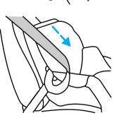
6. Allow the belt to retract. The belt will click as it retracts to indicate it is in the automatic locking mode.
