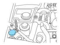
Only use a washer fluid that meets Ford specification. Refer to Lubricant specifications in the Capacities and specifications chapter.
