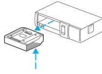
1. Pull the lever to remove a CD tray from the magazine.
