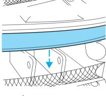
4. Lower the bracket and module tray assembly.
