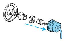
5. Disconnect the electrical connector from the bulb by pulling rearward.
