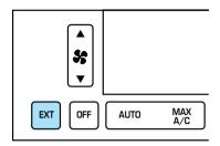
If the selected temperature is changed while the outside temperature is displayed, the new temperature will be displayed for four seconds after it is changed, then the outside temperature will return to the window.
