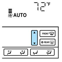
For continuous maximum cooling, push the temperature control until 16°C (60°F) is shown in the display window. The EATC will continue maximum cooling (disregarding the displayed temperature) until a warmer temperature is selected by pressing the temperature control.
