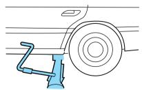
To lessen the risk of personal injury, do not put any part of your body under the vehicle while changing a tire. Do not start the engine when your vehicle is on the jack. The jack is only meant for changing the tire.
