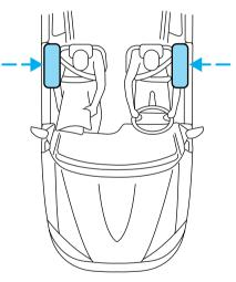
Side air bags, in combination with seat belts, can help reduce the risk of severe injuries in the event of a significant side impact collision.
