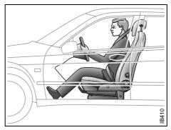
Correctly positioned safety belt
