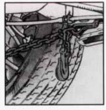
Attach T-hook chains to slots in the bottom of the floor pan directly ahead of rear wheels on both sides.
