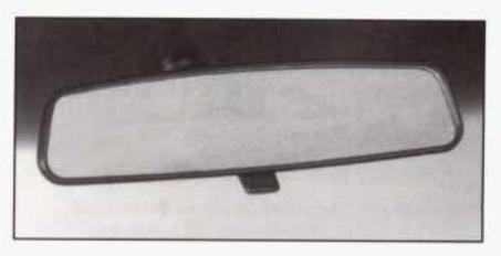
When you are sitting in a comfortable driving position, adjust the mirror so you can see clearly behind your vehicle. Grip the mirror in the center to move it up or down and side to side. The day/night adjustment allows you to adjust the mirror to avoid glare from the lamps behind you. Push the tab forward for daytime use; pull it back for night use.
