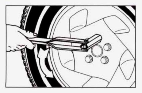
Use the wheel wrench to loosen the wheel nuts, but don't remove them.
