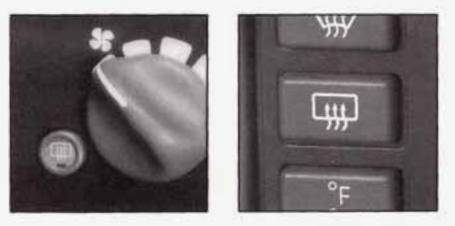
The lines you see on the rear window warm the glass. Press the button to start warming your window. If you have the standard system, a light will glow in the switch while the defogger is working.
