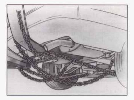
Position the lower sling crossbar directly behind and at lower edge of rear bumper cover.
