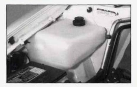
When your engine is cold, the coolant level should be at the FULL COLD mark or a little higher. When your engine is warm, the level should be up to the FULL HOT mark or a little higher.
