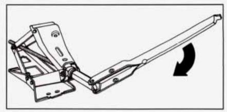
Rotate the wheel wrench to the right (clockwise) to raise the jack lift head until it fits under the vehicle.
