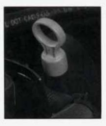
The transaxle fluid dipstick top is a round, red loop and is next to the brake master cylinder behind the engine block. Pull out the dipstick and wipe it with a clean rag or paper towel. Push it back in all the way, wait three seconds and then pull it back out again.
