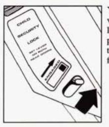
Your vehicle is equipped with rear door security locks that help prevent passengers from opening the rear doors of your car from the inside.
