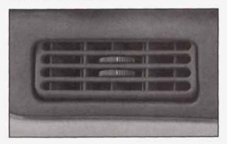
Your vehicle has air outlets that allow you to adjust the direction and amount of airflow inside the vehicle. Push the outlet up or down to direct airflow to your preference. Increase or reduce the amount of airflow by opening and closing the louvers. Opening and closing the louvers will also direct airflow from side-to-side.
