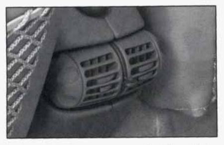
If you have the rear seat passenger outlet, it's attached to the back of the console. You can adjust the airflow toward either seating area, the floor or upward. Turn the end knobs up and down to direct airflow. Increase or reduce the amount of airflow by adjusting the lever between the two rear vents up or down. Open and close the louvers to direct airflow from side-to-side.
