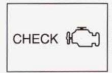
Your vehicle is equipped with a computer which monitors operation of the fuel, ignition and emission control systems.
