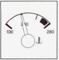
This gage shows the engine coolant temperature.
