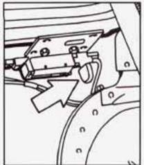
If your vehicle has a fuel door lock, the fuel door can be opened manually in case of an electrical power failure. Open the trunk. The release mechanism is on the driver's side of the vehicle, at the top of the trunk compartment. Pull the tab rearward to release the fuel door.
