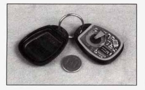
For battery replacement, use one Duracell<sup>®</sup> battery, type DL-2032, or a similar type.
