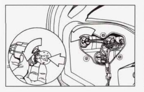
Turn the bulb socket assembly to the left (counterclockwise) to remove it from the lamp assembly.
