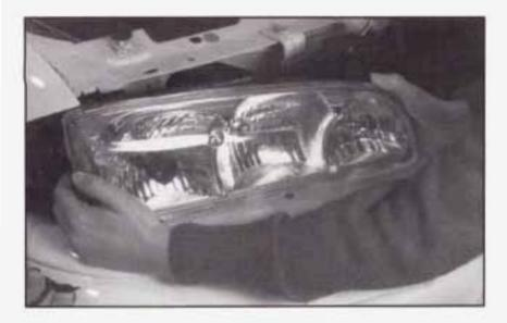
Slide the headlamp assembly outward (to the left) and lift it out.
