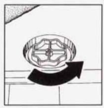
The equipment you'll need is in the trunk. Pull the carpeting from the floor of the trunk. Turn the center retainer bolt on the spare tire cover to the left (counterclockwise) to remove it.
