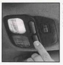
These front reading lamps and the interior courtesy lamps will come on when you open the doors.
