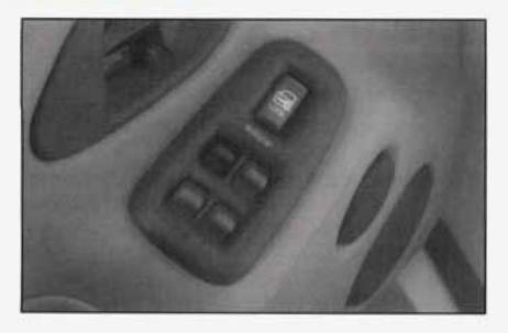
With power door locks, you can lock or unlock all the doors of your vehicle using the driver's or front passenger's door lock switch.
