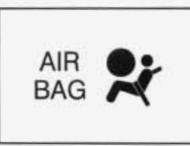
This light will come on when you start your engine, and it will flash for a few seconds. Then the light should go out. This means the system is ready.
