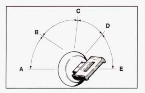
ACCESSORY (A): In this position you can operate your electrical power accessories. Press in the ignition switch as you turn the top of it toward you. LOCK (B): The only position in which you can remove the key. This locks your steering wheel, ignition and transaxle.
