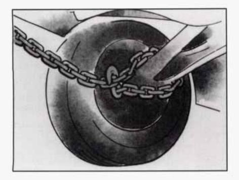
Attach a separate safety chain around the outboard end of each control arm.
