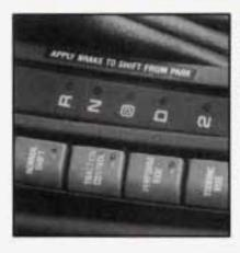
Press PERFORM SHIFT to allow the transaxle to shift at higher engine speeds, increasing acceleration performance. An indicator light on the switch will glow when performance shifting is in operation.
