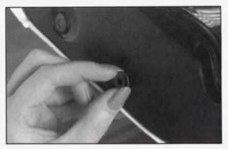
Pull the push pin with your fingers to remove it. (There are four pins altogether -- two on the driver's side and two on the passenger's side.)
