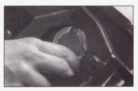
Tip the assembly and turn the bulb assembly to the left (counterclockwise) to remove it.
