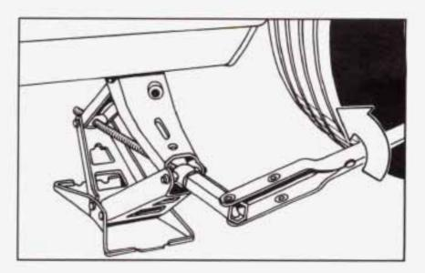
Lower the vehicle by rotating the wheel wrench to the left (counterclockwise). Lower the jack completely.
