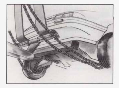
Position a 4" x 4" wood beam across sling chains contacting bottom of the radiator support. Position the lower sling crossbar directly under the front bumper.
