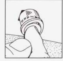
Press the button in to make your front and rear turn signal lamps flash on and off.
