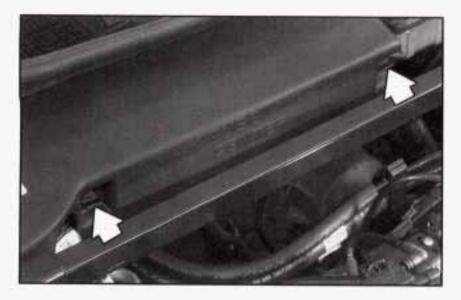
To check the fuses in this underhood fuse center, turn the two knobs one-quarter turn to the left (counterclockwise) and loosen the metal wing nut on the passenger side of the cover. Then remove the cover. The inside of the cover has a chart that explains the features and controls governed by each fuse and relay.
