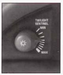
At night, you can turn off all exterior lamps when you are in PARK (P) by moving the twilight sentinel control all the way to MIN.
