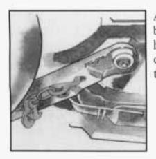
Attach T-hook chains on both sides in the slotted holes in the bottom of the frame, behind the front wheels.
