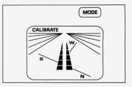
All electronic compasses need to know the magnetic profile of your car. This is called calibration and is done automatically by your compass. But, the feature is available if you would like to manually calibrate. Sometimes, strong magnetic fields can affect the compass. If the CALIBRATE light comes on as shown above, try calibrating the compass as follows:
