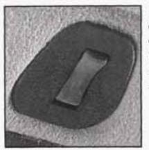
Your vehicle may be equipped with an express-open sunroof. Press the control switch rearward and release it to open the glass panel and sunshade.
