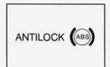
If there's a problem with the anti-lock brake system, this warning light will stay on. See "Anti-Lock Brake System Warning Light" in the Index.
