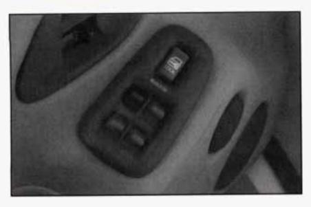
Switches on the driver's door panel control each of the windows when the ignition is on or when retained accessory power is active. In addition, each passenger door has a control switch for its own window.
