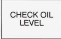
If the CHECK OIL LEVEL light on the instrument panel comes on, it means you need to check your engine oil level right away. For more information, see "Check Oil Level Light" in the Index. You should check your engine oil level regularly; this is an added reminder.
