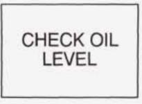
The CHECK OIL LEVEL light turns on for three seconds as a bulb check each time the ignition key is turned to the RUN position. If the light doesn't turn on, have your vehicle serviced.
