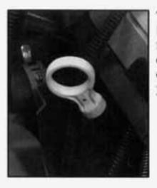
The engine oil dipstick is located behind the engine fans and in front of the engine oil fill cap. The top of the dipstick is a round, yellow loop.
