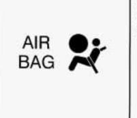
There is an air bag readiness light on the instrument panel, which shows AIR BAG.
