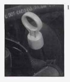
The transaxle fluid dipstick top is a round, red loop and is next to the brake master cylinder behind the engine block. Pull out the dipstick and wipe it with a clean rag or paper towel.
