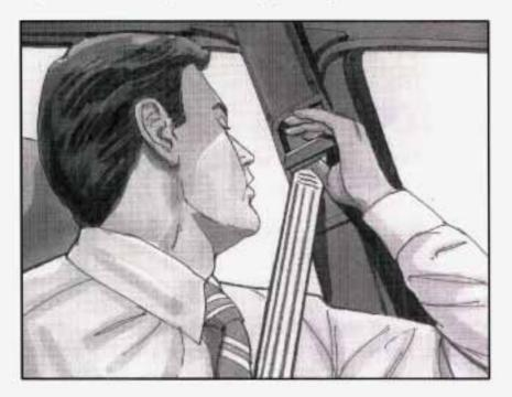
To move it down, squeeze the release handle and move the height adjuster to the desired position. You can move the adjuster up just by pushing up on the bottom of the release handle. After you move the adjuster to where you want it, try to move it down without squeezing the release handle to make sure it has locked into position.
