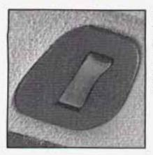
Your Bonneville may be equipped with an express-open sunroof. Press the control switch rearward and release it to open the glass panel and sunshade. If you want to stop the sunroof in a partially open position, lightly press the switch again. To completely open the sunroof, press the switch rearward again. The sunshade can also be opened by hand.
