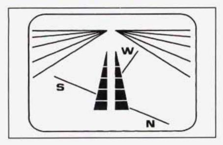
Some vehicles are equipped with an electronic compass. As with all compasses, this unit senses the earth's magnetic field to show the direction the car is pointing. The earth's magnetic field is not always the same direction as true north as we know it. So, you must enter a zone number to tell the compass the difference between magnetic and actual north. This tells the compass where in the country you are driving
