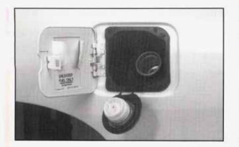
If you have the (L36) 3800 V6 engine, your fuel cap will be tethered and you cannot hang it on the inside fuel door while refueling.
