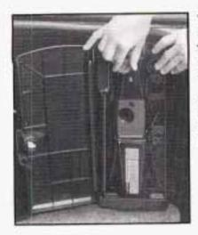
The box that stores the jack and wheel wrench is located on the passenger side trunk wall.
