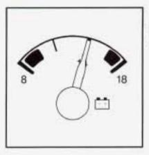
You may have a voltmeter unless you have the supercharged engine.
