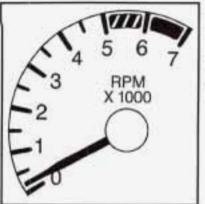
The tachometer shows your engine speed in revolutions per minute (rpm). Do not run your engine at speeds in the red area.
