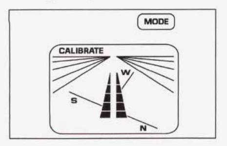
All electronic compasses need to know the magnetic profile of your car. This is called calibration and is done automatically by your compass. But, the feature is available if you would like to manually calibrate. Sometimes, strong magnetic fields can affect the compass. If the CALIBRATE light comes on as shown above, try calibrating the compass as follows:
