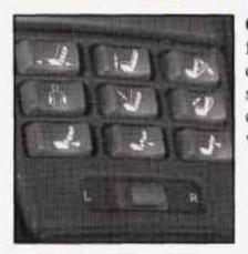
On some models, you'll find the controls on the center console. Slide the selector switch to L or R to choose the front seat you want to adjust.
