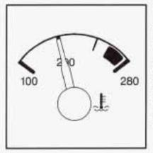
This gage shows the engine coolant temperature.
