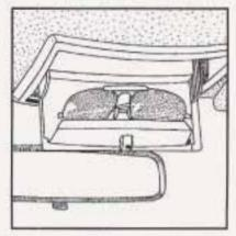
Some models have a storage compartment for glasses in your overhead console. Press the release button to lower the door. Place your glasses inside the door. To close the door, raise it and press it into position.
