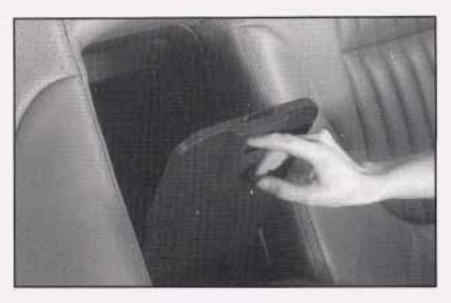
Pull down the interior door to access the trunk.
