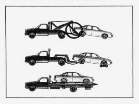
Before hooking up to a tow truck, be sure to read all the information in "Towing Your Vehicle" earlier in this section. Also be sure to use the proper hook-up for your particular vehicle. Attach T-hook chains on both sides in the slotted holes in the bottom of the frame rail just ahead of the rear wheels. These slots are to be used when loading and securing to car carrier equipment.
