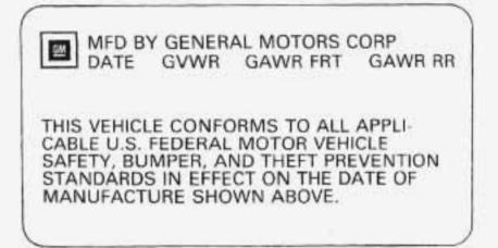
The other label is the Certification label, found on the rear edge of the driver's door. It tells you the gross weight capacity of your vehicle, called the GVWR (Gross Vehicle Weight Rating). The GVWR includes the weight of the vehicle, all occupants, fuel and cargo. Never exceed the GVWR for your vehicle, or the Gross Axle Weight Rating (GAWR) for either the front or rear axle.
