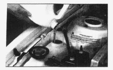
Then fill the coolant surge tank with the proper mix, up to the FULL COLD mark.
