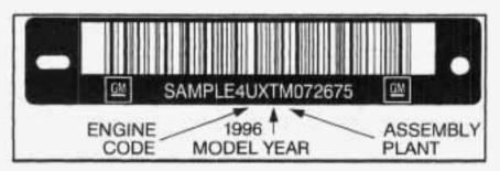
This is the legal identifier for your Pontiac. It appears on a plate in the front corner of the instrument panel, on the driver's side. You can see it if you look through the windshield from outside your vehicle. The VIN also appears on the Vehicle Certification and Service Parts labels and the certificates of title and registration.
