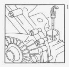
The manual transaxle dipstick is located below the brake master cylinder, near the rear of the transaxle case. Flip the handle up and then pull out the dipstick and clean it with a rag or paper towel.
