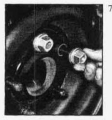
Replace the wheel nuts with the rounded end of the nuts toward the wheel. Tighten each nut by hand until the wheel is held against the hub.
