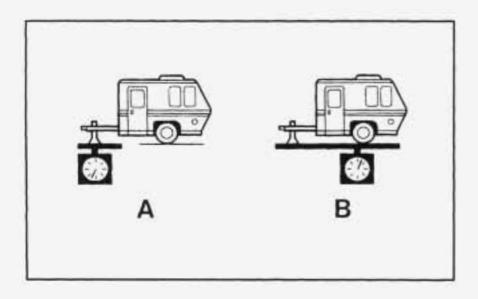
If you're using a weight-carrying hitch, the trailer tongue (A) should weigh 10% of the total loaded trailer weight (B). If you have a weight-distributing hitch, the trailer tongue (A) should weigh 12% of the total loaded trailer weight (B).
