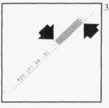
Check both sides of the dipstick, and read the lower level. The fluid level must be in the cross-hatched area.
