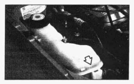
The surge tank is located on the passenger side of the engine compartment.
