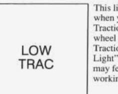
This light will come on when your Enhanced Traction System is limiting wheel spin. See "Enhanced Traction System Active Light" in the Index. You may feel or hear the system working, but this is normal.
