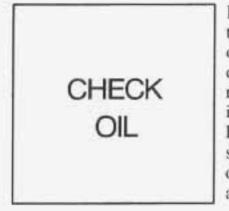
If the CHECK OIL light on the instrument panel comes on, it means you need to check your engine oil level right away. For more information, see "Check Oil Light" in the Index. You should check your engine oil level regularly; this is an added reminder.
