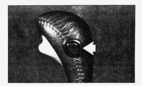
To turn the system on or off, press the button on the shift lever knob.
