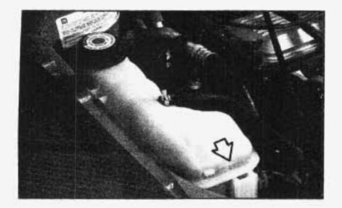
The coolant level should be at the FULL COLD line. If it isn't, you may have a leak in the radiator hoses, heater hoses, radiator, water pump or somewhere else in the cooling system.
