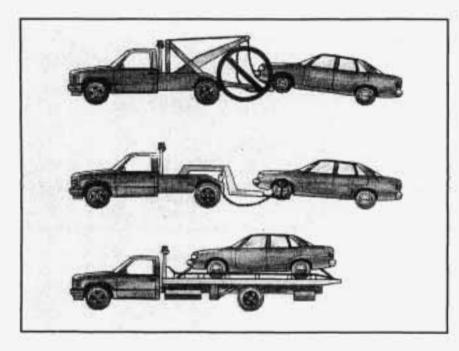
Before hooking up to a tow truck, be sure to read all the information in "Towing Your Vehicle" earlier in this section. Attach T-hook chains into the slots in the bottom of the floor pan, just behind the front wheels, on both sides. These slots are used when loading and securing to car carrier equipment.
