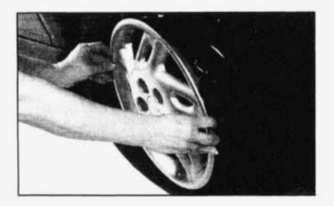
If you have a wheel cover, use your fingers to carefully pry the wheel cover from the wheel. Then remove the flat tire.
