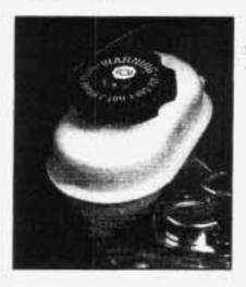
Your brake master cylinder reservoir is here. It is filled with DOT-3 brake fluid.
