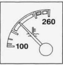
With the ignition in the RUN position, this gage shows the engine coolant temperature.
