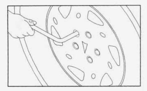
Using the wheel wrench, remove the plastic cap nuts (if your vehicle is so equipped) and *loosen* all the wheel nuts. Don't remove the wheel nuts yet. On some models, a cover plate must be removed to find the wheel nuts. Carefully use the wedge end of the wheel wrench to pry it off.
