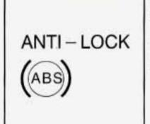
If there's a problem with the anti-lock brake system, this warning light will stay on. See "Anti-Lock Brake System Warning Light" in the Index.
