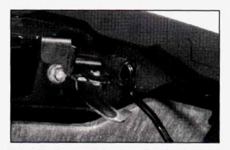
Lift the hood, release the hood prop from its retainer and put the hood prop into the slot in the hood. You may have a lamp that comes on when you lift the hood.
