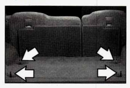
There are four cargo tie downs in the rear that allow you to strap cargo in and keep it from moving inside the vehicle.
