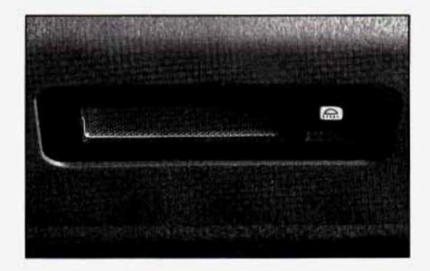
Press the side of the switch with the lamp symbol to turn on the front and rear dome lamps. Pressing the other side of the switch will turn the cargo area dome lamp off, even when the endgate and doors are open.
