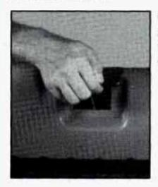
Open the glass and reach inside the endgate to lift the handle and open the endgate.
