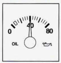
The oil pressure gage shows the engine oil pressure in psi (pounds per square inch) when the engine is running.
