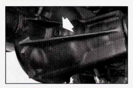
If the level is below the bottom of the filler plug hole, you'll need to add some lubricant. Add enough lubricant to raise the level to the bottom of the filler plug hole.
