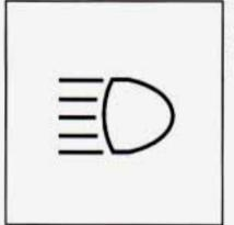
When the high beams are on, this indicator light on the instrument panel also will be on.
