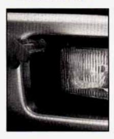
Remove the screws from the headlamp retainer.
