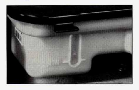
You can check the brake fluid without taking off the cap. Just look at the windows on the brake fluid reservoir. The fluid levels should be above MIN. If they aren't, have your brake system checked to see if there is a leak.
