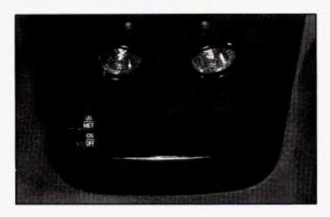
The outside air temperature and the compass are displayed at the front of the overhead console. The control switches are located to the left of the display. Turn the display on or off by pressing the ON/OFF switch. Display the temperature in either degrees Fahrenheit (English) or Celsius (metric) by pressing the US/MET switch.
