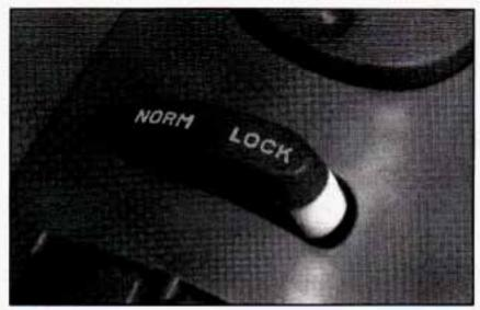
Four-door vehicles have a lockout feature to prevent passengers from operating power windows. It is located on the driver's door. Press LOCK to activate this feature. Press NORM and the windows return to normal operation.
