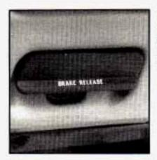
Pull the BRAKE RELEASE lever. It is located on the bottom driver's side of the instrument panel.
