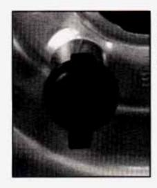
The locking wheel nut can be removed by snapping the rubber weather cover off the face of the lock case.
