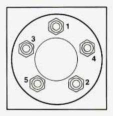
Use the wrench to tighten the wheel nuts firmly in a crisscross sequence as shown.
