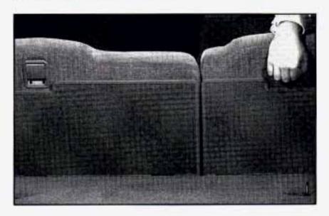
The rear seat release handles are in the upper center of the rear of the seatbacks. Push back on the seatbacks as you pull up on the handles.
