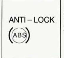
With the anti-lock brake system, this light will come on when you start your engine and may stay on for several seconds. That's normal.
