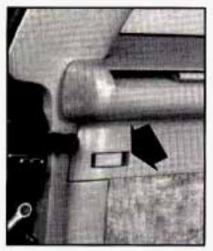
To remove your jack cover, pull up on the latch at the end of the cover, near the endgate and the latch on the top of the cover. Remove the wheel blocks, jack and wheel wrench.
