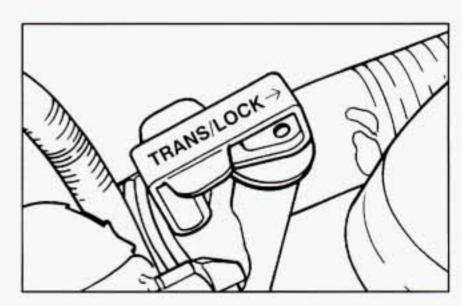
Flip the handle up and then pull out the dipstick and wipe it with a clean rag or paper towel. Push it back in all the way, wait three seconds and then pull it back out again.
