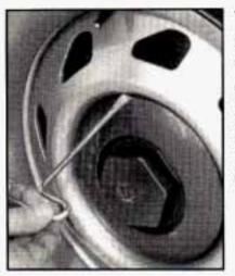
The optional hub cap removal tool is stowed with the jack. Position the hub cap removal tool in the notch and pull straight away from the wheel to avoid potential damage to the hub cap and wheel surface.
