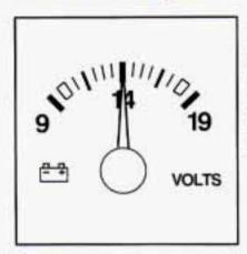
When your engine is not running, but the ignition is on (in the RUN position), this gage shows your battery's state of charge in DC volts.
