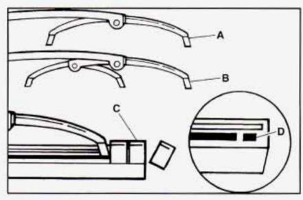
4. To install the new wiper insert, slide the insert (D), notched end last, into the end with two blade claws (A). Slide the insert all the way through the blade claws at the opposite end (B). Plastic caps (C) will be forced off as the insert is fully inserted.
