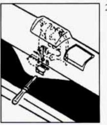
Use a thin screwdriver to reach through the access holes in both the trim panel and the hardware cover.
