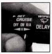
Once you're going about 25 mph (40 km/h) or more, you can move the cruise control switch from ON to R/A for about a 1/2 second.
