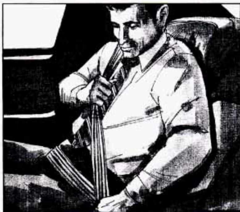
3. To make the lap part tight, pull down on the buckle end of the belt as you pull up on the shoulder part.
