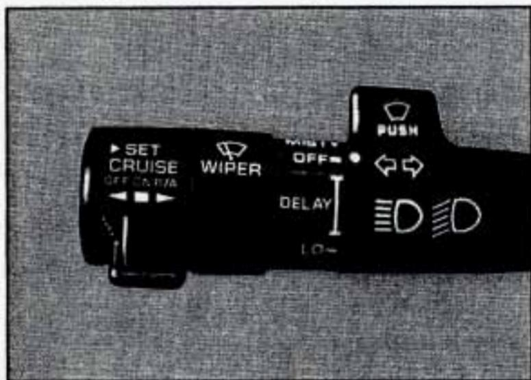
2. Move the CRUISE switch to OFF. (The CRUISE light will go out.)
