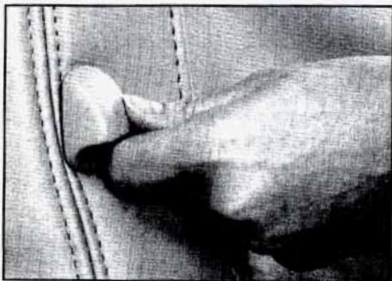
To fold the seatback forward, push the seatback toward the rear as you lift this latch. Then the seatback will fold forward. The latch must be down for the seat to work properly.
