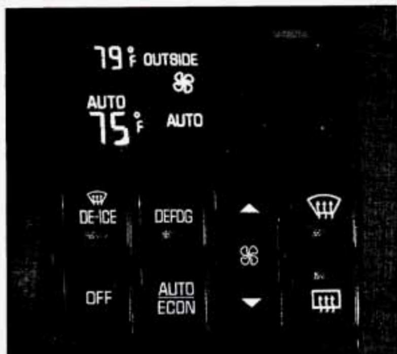
Your vehicle has strategically placed electronic sensors that feed information to the vehicle's computer systems. Your vehicle can control the ventilation, heating and air conditioning automatically year round. The outside temperature, inside temperature setting, fan speeds and the ECC selection are displayed on a digital screen.
