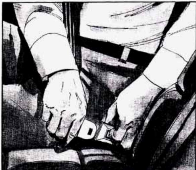
To unlatch the belt, just push the button on the buckle.
