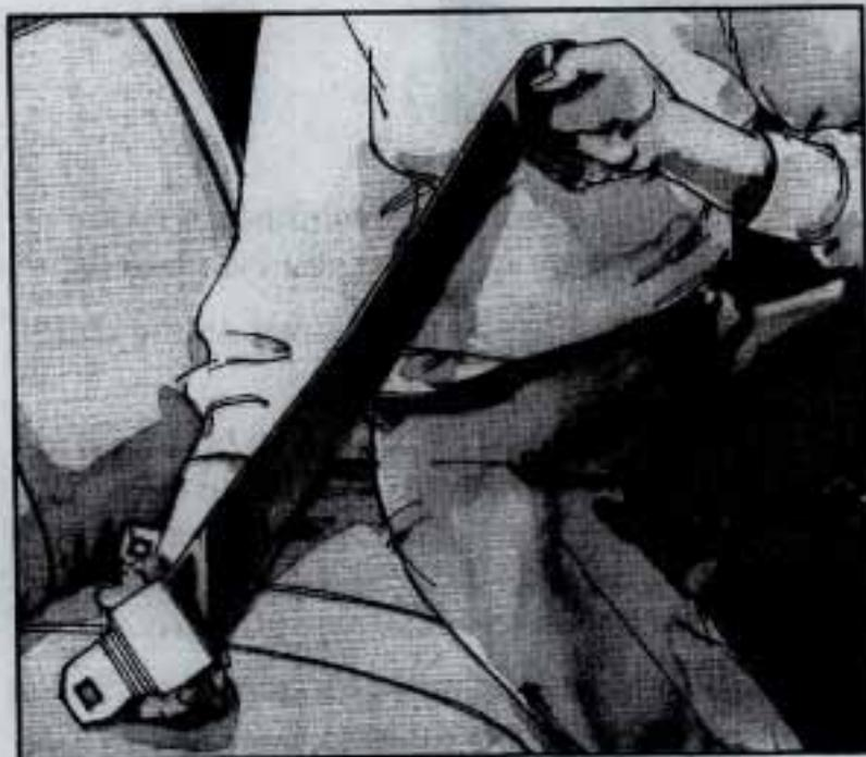
1. Make the belt as long as possible by tilting the latch plate and pulling it along the belt.
