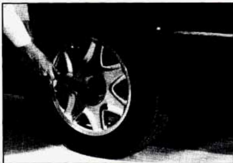
5. Using the wheel wrench loosen all the wheel nuts. Don't remove them yet.
