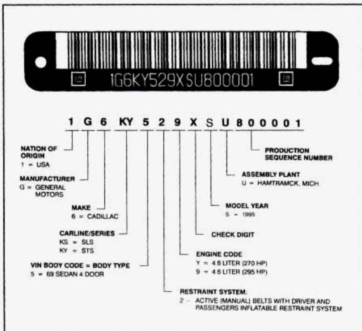
This is the legal identifier for your Cadillac. It appears on a plate in the front corner of the instrument panel, on the driver's side. You can see it if you look through the windshield from outside your vehicle. The VIN also appears on the Vehicle Certification and Service Parts labels and the certificates of title and registration.
