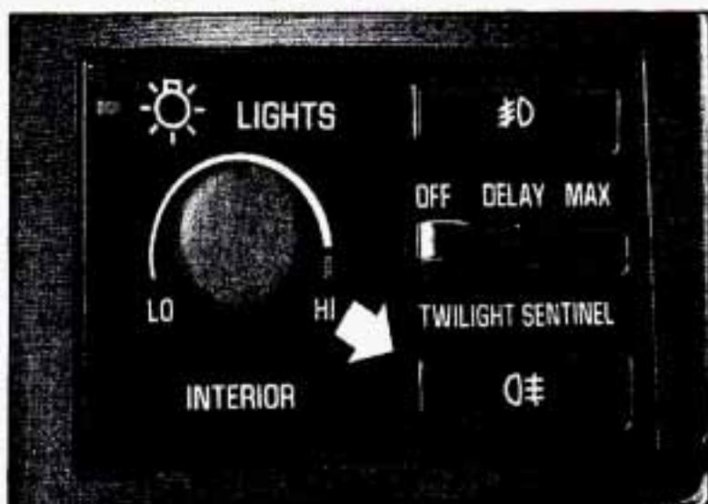
To operate the rear fog lamps, first turn on the front fog lamps, then press the lower switch. A small indicator light will glow to tell you they are on. Press the switch again to turn them off.
