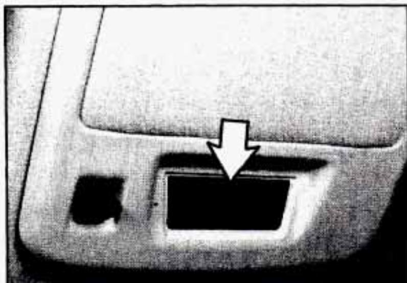
This transmitter allows you to consolidate the functions of up to three individual hand-held transmitters. It will operate garage doors and gates, or with the accessory package, other devices controlled by radio frequency such as home/office lighting systems and security systems.
