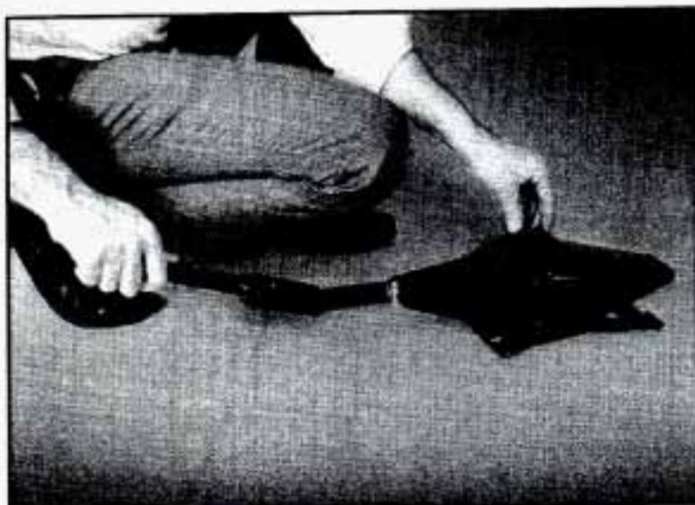
3. Attach the wheel wrench to the jack bolt and rotate it clockwise. That will raise the lift head a little.
