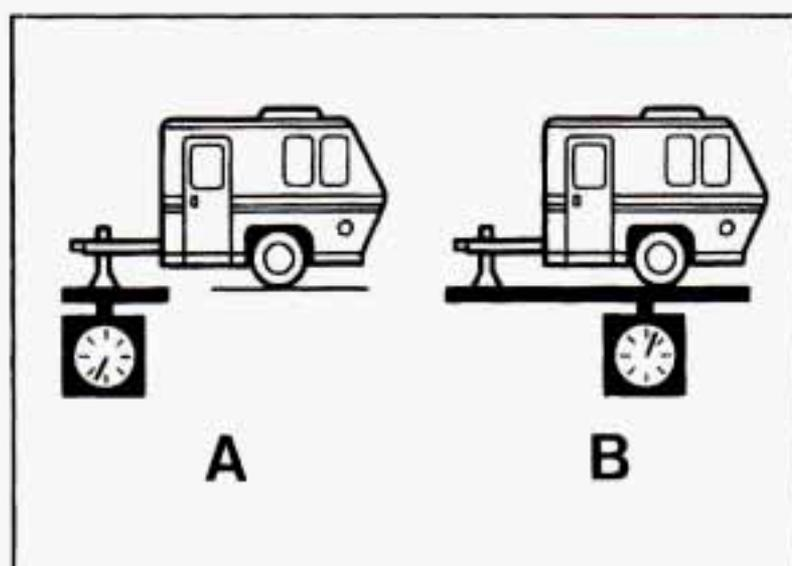
If you're using a "dead-weight" hitch, the trailer tongue (A) should weigh 10% of the total loaded trailer weight (B). If you have a "weight-distributing" hitch, the trailer tongue (A) should weigh 12% of the total loaded trailer weight (B).
