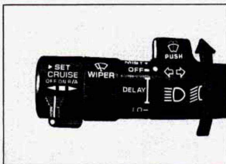
To wash your windshield, press and hold the paddle labeled PUSH. Once you feel you have enough washer fluid on the windshield, release the paddle. The wipers will continue to clear the windshield, then either stop or return to your preset speed.
