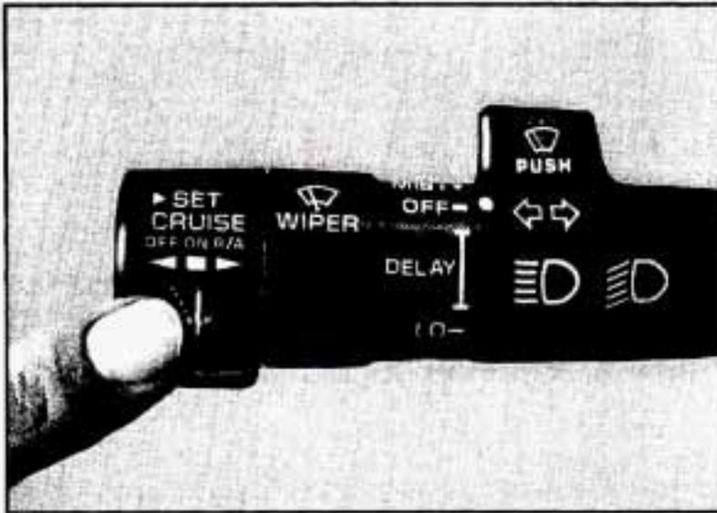
1. Move the cruise control switch to ON.
