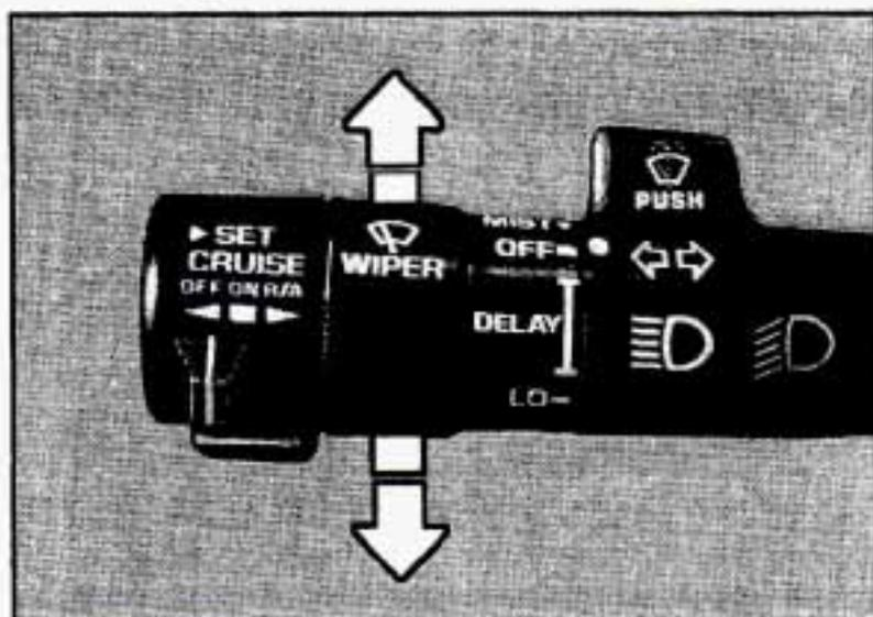
The turn signal has two upward (for right) and two downward (for left) positions. These positions allow you to signal a turn or a lane change.
