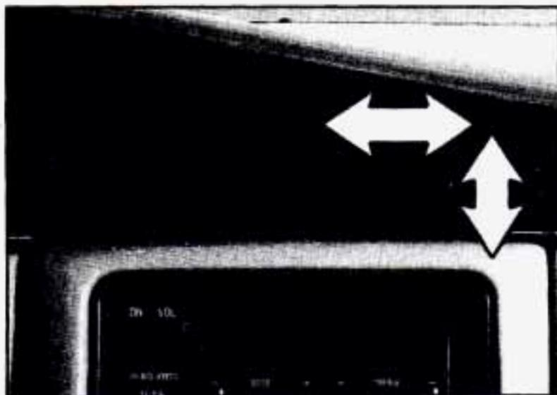
Air outlets are located in the center and at each side of the instrument panel. You can adjust the direction of airflow by moving the center control levers or you can stop the airflow by moving the lever located on each side of the outlets downward.
