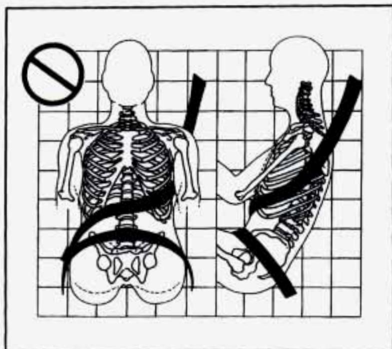
**A:** The shoulder belt is worn under the arm. It should be worn over the shoulder at all times.
