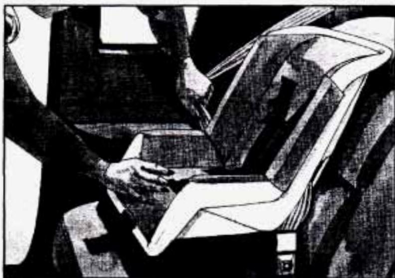
5. To tighten the belt, pull up on the shoulder belt while you push down on the child restraint.
