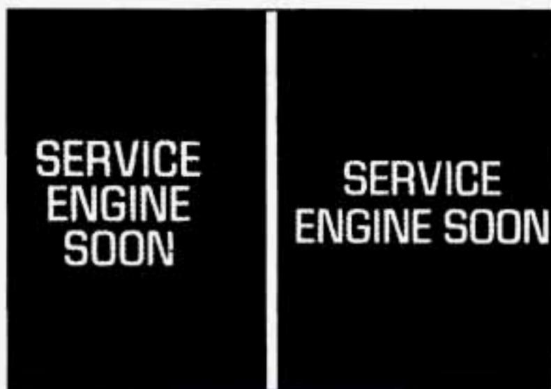
A computer monitors operation of your fuel, ignition and emission control systems. One of these lights should come on when the ignition is on, but the engine is not running, as a check to show you it is working. If one of these lights doesn't come on, have it fixed right away.
