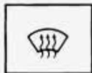
Press this button to remove fog or frost from the windshield.
