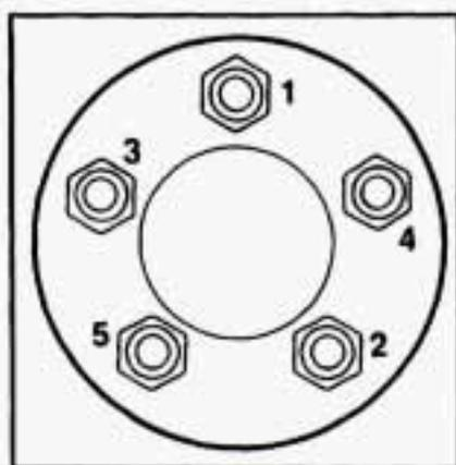
12. Tighten the wheel nuts firmly in a criss-cross sequence as shown.
