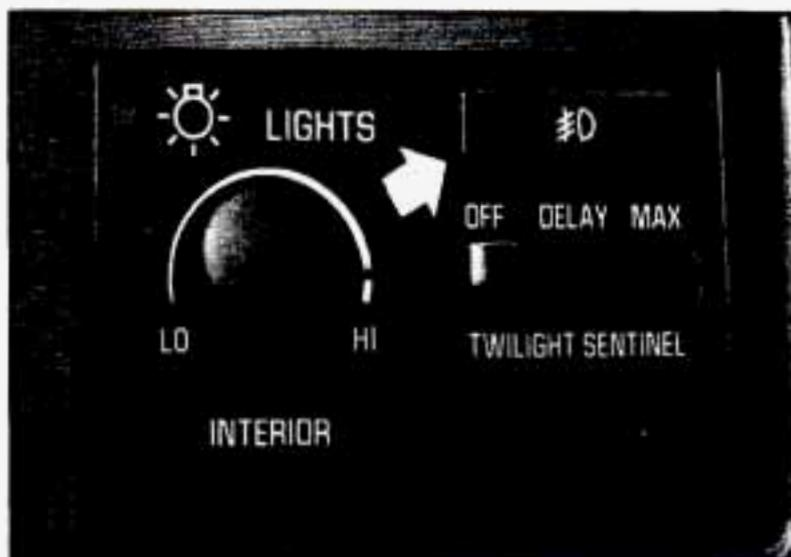
Use your fog lamps for better vision in foggy or misty conditions. When you press the upper fog lamp switch, a small indicator light will glow to tell you the fog lamps are on. Press the switch again to turn them off.
