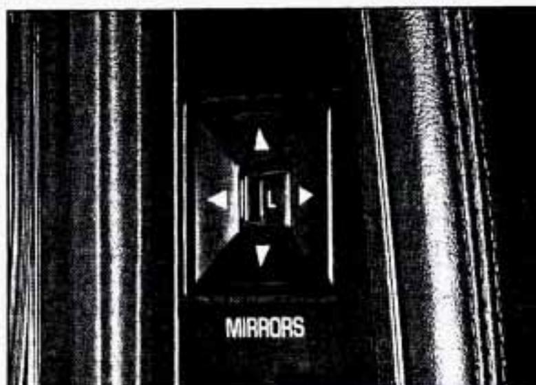
The control on the driver's door armrest operates both outside rearview mirrors. Move the center switch to the left to select the driver side mirror, or to the right to select the passenger side mirror. Then press the control pad in the direction of the desired mirror movement. Adjust each mirror so that you can just see the side of your vehicle.
