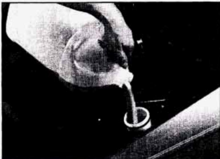
Open the cap labeled **WASHER FLUID ONLY**. Add washer fluid until the tank is full.
