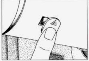
Press the button in to make your front and rear turn signal lights flash on and off.
