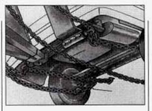
Position the lower sling crossbar directly below and to the rear of the rear bumper.
