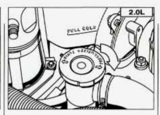
9. Replace the thermostat, making sure it is properly inserted, then replace the pressure cap. At any time during this procedure if coolant begins to flow out of the filler neck, reinstall the pressure cap. Be sure the arrows on the pressure cap line up like this.
