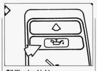
**Oil Warning Light (2.0L L4 ENGINE)** If you have a low engine oil pressure problem, this light will stay on after you start your engine, or come on when you are driving. This indicates that your engine is not receiving enough oil. The engine could be low on oil, or could have some other oil problem. Have it fixed immediately.
