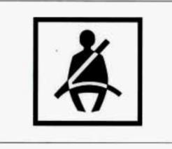
This figure lights up as a reminder to buckle up. (See Safety Belt Warning Light in the Index.)
