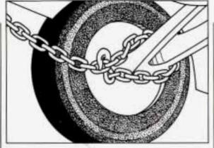
Attach a separate safety chain around the outboard end of each lower control arm.
