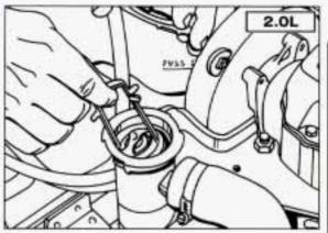
Your engine also has a thermostat housing with a pressure cap. This cap and the thermostat must be taken out to add coolant.
