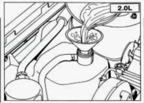
Then fill the coolant recovery tank to FULL COLD.
