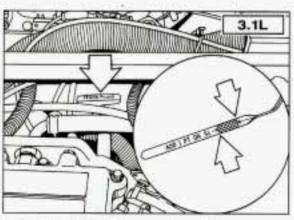
3.1L V6: Checking Automatic Transaxle Fluid
