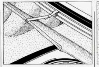
If your vehicle is equipped with a spare tire housing lid hook, pull the front of the lid up and hook it to the rear upper edge of the trunk.
