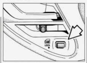
On 2-door models, push the switch down to lock your doors and up to unlock them.
