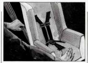
To tighten the belt, pull up on the shoulder belt while you push down on the child restraint.
