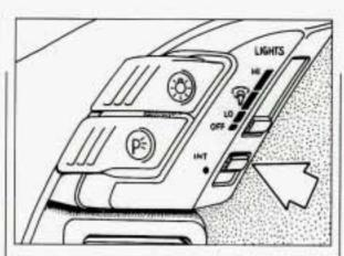
If your vehicle is not equipped with fog lights, you have a switch labeled **INT** (Interior). Slide it up to turn on the interior courtesy lights.
