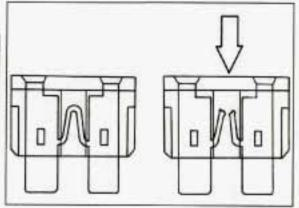
Look at the silver-colored band inside the fuse. If the band is broken or melted, replace the fuse. Be sure you replace a bad fuse with a new one of the identical size and rating.
