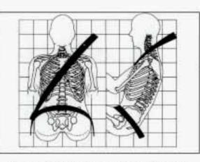
The lap belt should be worn as low on the hips as possible. In a crash, this applies force to the strong pelvic bones. And you'd be less likely to slide under the lap belt. If you slid under it, the belt would apply force at your abdomen. This could cause serious or even fatal injuries. The shoulder belt should go over the shoulder and across the chest. These parts of the body are best able to take belt restraining forces. The safety belt locks if there's a sudden stop or a crash.
