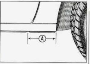
9. Near each wheel well is a notch in the frame which the jack head fits in. The front notch is 9" (23 cm) back from the rear wheel well. The rear notch is 8" (20 cm) forward from the rear wheel well. If your vehicle has flared side moldings, both front and rear notches are 18" (46 cm) from the wheel wells.
