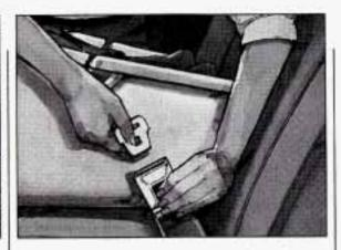
Put the belt's special latch plate into the vehicle's safety belt buckle.
