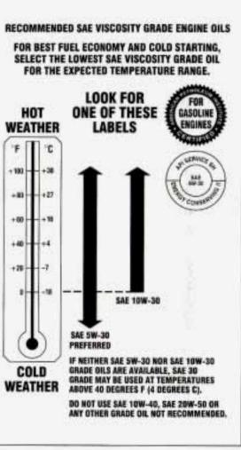
As shown in the chart, SAE 5W-30 is best for your vehicle. However, you can use SAE 10W-30 if it's going to be 0°F (-18°C) or above. These numbers on an oil container show its viscosity, or thickness. Do not use other viscosity oils, such as SAE 10W-40 or SAE 20W-50.
