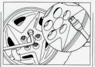
Using the wheel wrench, remove the plastic cap nuts and loosen all the wheel nuts. Don't remove the wheel nuts yet.
