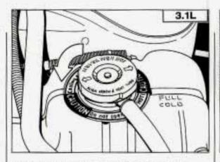
You can remove the coolant surge tank pressure cap when the cooling system, including the coolant surge tank pressure cap and upper radiator hose, is no longer hot. Turn the pressure cap slowly to the left until it first stops. (Don't press down while turning the pressure cap.) If you hear a hiss, wait for that to stop. A hiss means there is still some pressure left.
