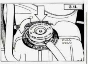
Then keep turning the cap, but now push down as you turn it. Remove the pressure cap.
