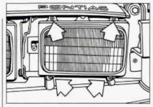
Remove the four Torx<sup>®</sup> screws from the corners of the frame around the headlight.
