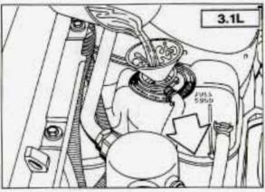
Fill the coolant surge tank with the proper mix, up to FULL COLD.
