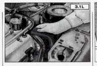
4. With the coolant surge tank pressure cap off, start the engine and let it run until you can feel the upper radiator hose getting hot. Watch out for the engine fan. By this time, the coolant level inside the coolant surge tank may be lower. If the level is lower, add more of the proper mix to the coolant surge tank until the level reaches FULL COLD.
