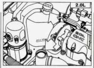
Put the cap back on the coolant recovery tank, but leave the thermostat housing pressure cap off.
