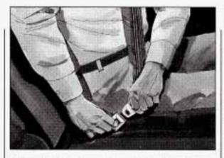
To unbuckle the automatic belt, just push the button on the buckle.
