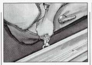
Push the spring on the hook near the door and remove the special belt.
