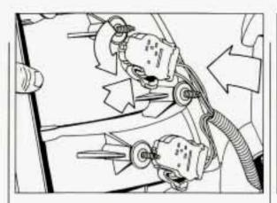
Press the bulb housing release lever and turn the housing % turn counterclockwise to remove it.
