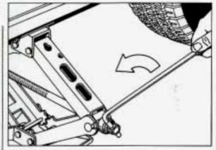
Lower the vehicle by rotating the jack handle counterclockwise. Lower the jack completely.
