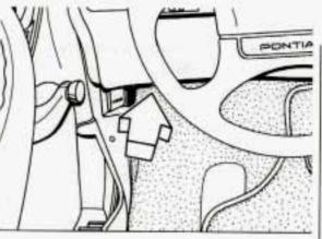
The fuse panel is located on the lower left side of the instrument panel. To open, pull the handle marked FUSE down and forward.
