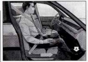
Adjust the seat (to see how, see Seats in the Index) so you can sit up straight. Move your seat far enough forward that your feet touch the part of the vehicle that is called the "toeboard" (A). That way you'd be less likely to slide under the lap belt in a crash.
