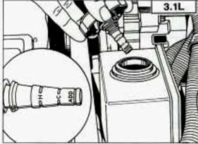
3.1L V6 Engine: Checking Power Steering Fluid
