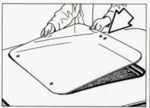
Push forward on the rear edge of the glass while lowering the panel. Do not force a hinge if it binds in a slot. Reposition the glass panel and start again. Finally, push the glass release tab, engage the latch with the striker and close the panel.
