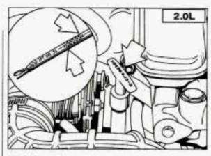
2.0L L4: Checking Automatic Transaxle Fluid
