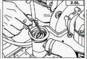
Pull the thermostat out of the housing.
