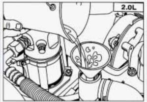
Fill the thermostat housing with the proper mix, up to the base of the filler neck.
