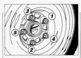
Tighten the wheel nuts firmly in a criss-cross sequence, as shown.
