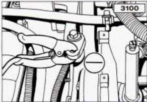
9. Attach the cable at least 18 inches (45 cm) away from the dead battery, but not near engine parts that move. The electrical connection is just as good there, but the chance of sparks getting back to the battery is much less.
