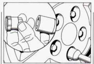
5. Using the wheel wrench, remove the wheel nut caps (if your vehicle has them) and loosen all the wheel nuts. Don't remove them yet. On some models, a cover plate must be removed to find the wheel nuts. Carefully use the wedge end of the wheel wrench to pry it off.
