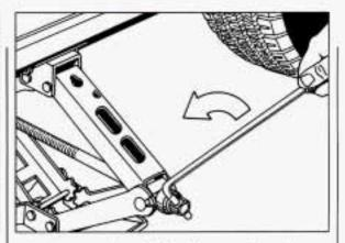
12. Lower the vehicle by rotating the jack handle counterclockwise. Lower the jack completely.
