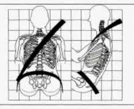
The lap belt should be worn as low on the hips as possible. In a crash, this applies force to the strong pelvic bones. And you'd be less likely to slide under the lap belt. If you slid under it, the belt would apply force at your abdomen. This could cause serious or even fatal injuries. The shoulder belt should go over the shoulder and across the chest. These parts of the body are best able to take belt restraining forces.
