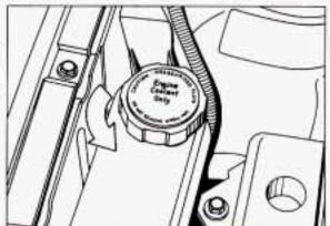
1. You can remove the coolant surge tank pressure cap when the cooling system, including the coolant surge tank pressure cap and upper radiator hose, is no longer hot. Turn the pressure cap slowly about onequarter turn to the left and then stop. If you hear a hiss, wait for that to stop. A hiss means there is still some pressure left.
