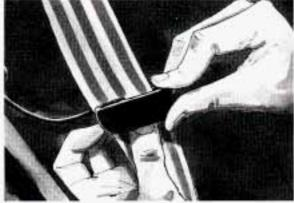
Slide the guide under and past the belt. The elastic cord must be under the belt. Then, place the guide over the belt, and insert the two edges of the belt into the slots of the guide.
