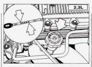
2.3L Quad 4: Checking Engine Oil
