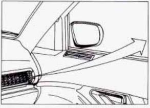
For maximum air flow to the side windows, turn the right knob to **BI-LEV**, turn the fan control to **HIGH**, close the center vents and direct the side vents toward the side windows. This setting does not direct any air to the windshield.
