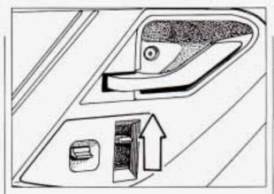
The rear doors of your vehicle cannot be opened from inside when this feature is in use. If you want to open a rear door when the security lock is on:
