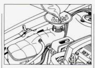
Fill the coolant surge tank with the proper mix, up to FULL COLD, or just above the small cylinder at the base of the opening.
