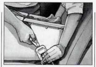
Put the hook on the free end through the slot in the latch plate.
