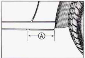
6. Near each wheel well is a notch in the frame which the jack head fits in. The front notch is 9" (23 cm) back from the rear wheel well. The rear notch is 8" (20 cm) forward from the rear wheel well. If your vehicle has flared side moldings, both front and rear notches are 18" (46 cm) from the wheel wells.
