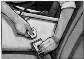
Put the belt's special latch plate into the vehicle's safety belt buckle.
