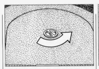
Turn the center retainer nut on the compact spare tire housing counterclockwise to remove it, then lift the tire cover. You will find the jacking instructions label on the underside of the tire cover.
