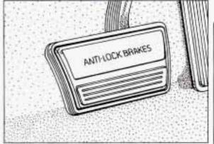
When you start your vehicle, or when you begin to drive away, you may hear a momentary motor or clicking noise. And you may even notice that your brake pedal moves a little while this is going on. This is the ABS system testing itself. If there's a problem with the anti-lock brake system, the anti-lock brake system warning light will stay on or flash.
