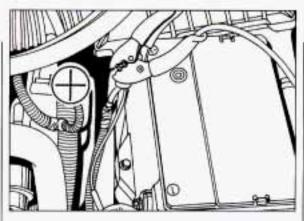
6. Connect the red positive (+) cable to the positive (+) terminal of the vehicle with the dead battery. Use a remote positive (+) terminal if the vehicle has one.
