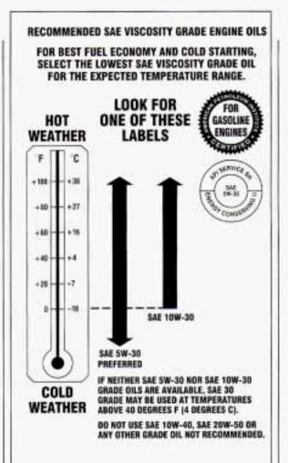
As shown in the chart, SAE 5W-30 is best for your vehicle. However, you can use SAE 10W-30 if it's going to be 0°F (-18°C) or above. These numbers on an oil container show its viscosity, or thickness. Do not use other viscosity oils, such as SAE 10W-40 or SAE 20W-50.
