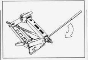
Remove the band around the jack. Turn the jack handle clockwise to raise the jack head a few inches.
