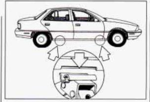
7. Position the jack under the vehicle. Raise the jack head until it fits firmly into the notch in the vehicle's frame nearest the flat tire. Do not raise the vehicle yet. Put the compact spare tire near you.
