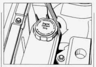
Then replace the pressure cap. Be sure the pressure cap is tight.
