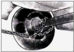
Attach a separate chain to each side of the axle inboard of the spring.
