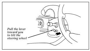
The lever to tilt the steering wheel
