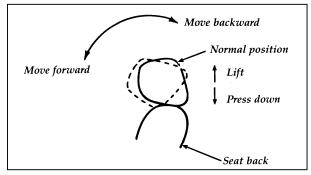
Adjusting the four-way head restraint
