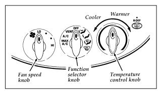
The knobs that control the manual heating and air conditioning system
