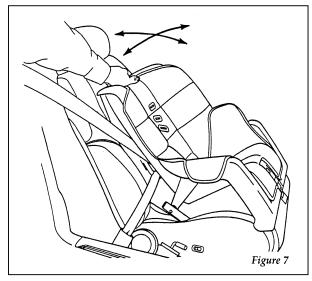
Checking that the seat is secure
