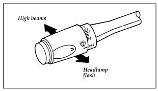
Turning on the high beams
