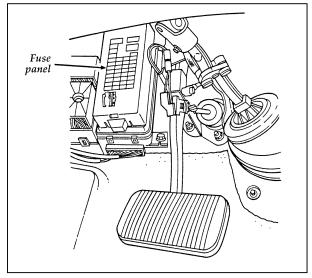
The instrument panel fuses and relays
