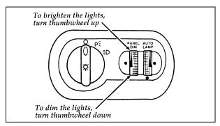
The thumbwheel that controls the light on the instrument panel
