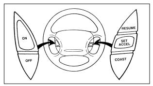
The speed control buttons on the steering wheel
