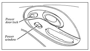
The window controls on the passenger's door
