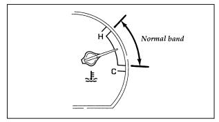
Engine coolant temperature gauge
