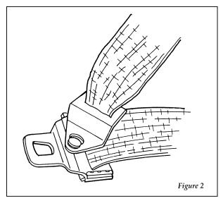
The reverse side of the shoulder belt attached to the lap belt
