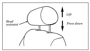
Adjusting the standard head restraint
