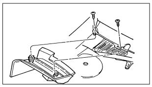
Removing the water shield
