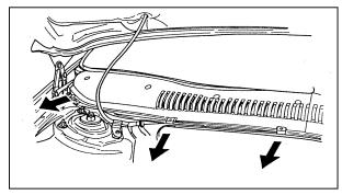
Removing the vacuum hose clips
