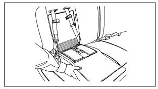
Figure 3: Opening the built-in child seat
