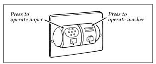
The liftgate window wiper and washer switches
