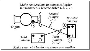
Jumper cable connections
