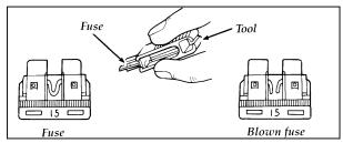
Fuse puller tool and fuse
