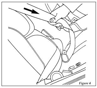
Setting the retractor to automatic locking mode
