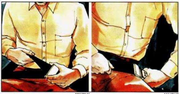
Each jump seat has a lap belt with no retractor. To make the belt longer, tilt the latch plate a little and pull the belt.
