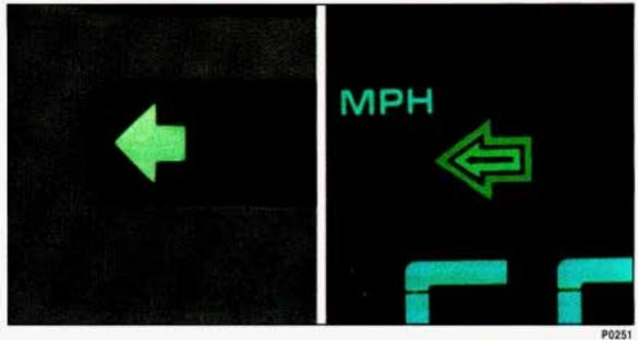
This light with the green arrows is on the instrument cluster. The turn signal indicator will come on whenever you signal a turn or lane change. See "Turn and Lane Change Signal" in this section.
