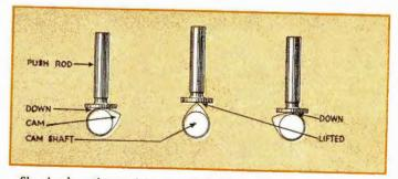
Showing how the revolving cam shaft lifts push rod. (Cut No. 12)
