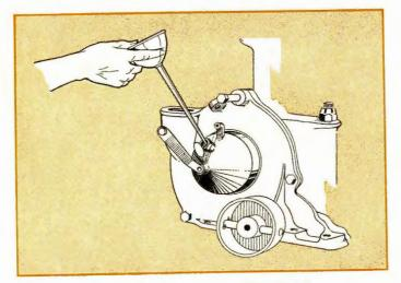
Oiling the Ford commutator. (Cut No. 29)
