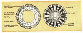
The Ford magneto. The flywheel with magnets revolves with the engine, while magneto coils remain stationary. (Cut No. 19)
