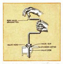
Method of grinding valve. (Cut No. 10)
