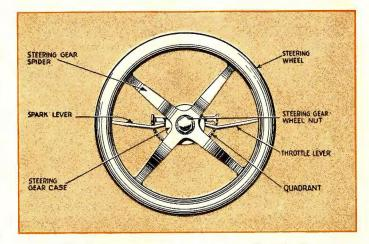
The Ford steering wheel arrangement. (Cut No. 3)
