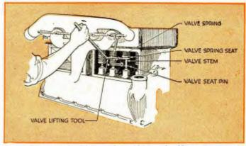
How the valve lifting tool should be used. (Cut No. 9)
