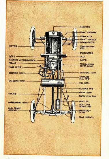
The Ford chassis-top view, which is identical in all Model T's. (Cut No. 2)
