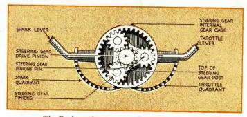
The Ford steering gear assembly. (Cut No. 27)
