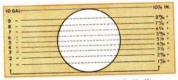
Gasoline measure for 10-gallon tank. (Cut No. 32)
