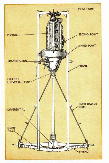
Showing one of the many Ford three point suspensions—also how the engine strengthens the frame. (Cut No. 31)
