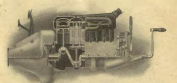
Semi-Sectional View of Model T Engine
