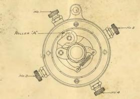
Roller "A" should be on Contact Post No. 1 when Cylinder No. 1 is ready to fire Diagram Showing Proper Method of Setting Commutator
