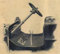
The hand lever when thrown forward engages high speed; when pulled back, operates the emergency brake. The lever is in neutral when almost vertical and clutch is in a released condition. With the hand lever thrown forward in high speed, a light pressure on pedal "C" releases the clutch, while a full pressure on the pedal throws in the slow speed; by gradually
