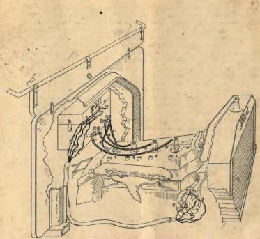
Model T Wiring Diagram
