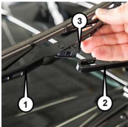
**Wiper Blade Removed From Wiper Arm**
