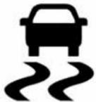
The “ESC Activation/Malfunction Indicator Light” in the instrument cluster will come on when the ignition is turned to the ON mode. It should go out with the engine running. If
