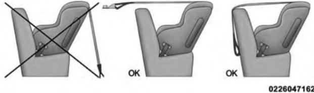
1. Look behind the seating position where you plan to install the child restraint to find the tether anchorage. You may need to move the seat forward to provide better access to the tether anchorage. If there is no top
