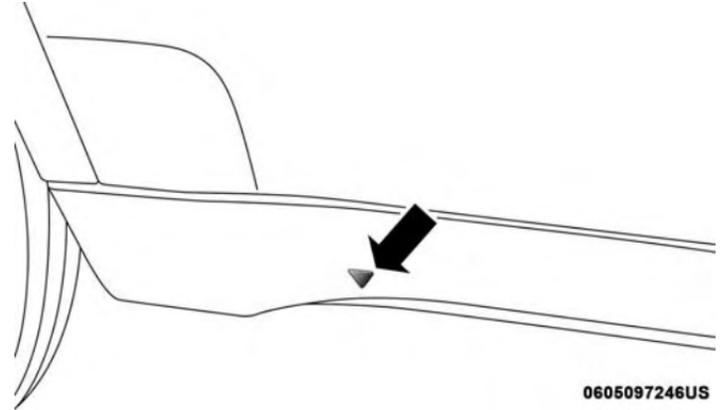
Lift Point Symbol On Sill Molding
