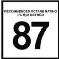
These engines are designed to meet all emissions regulations and provide optimum fuel economy and performance when using high quality unleaded "Regular" gasoline having a posted octane number of 87 as specified by the (R+M)/2 method. The use of higher
