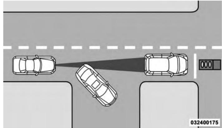
Stationary Object And Stationary Vehicle Example
