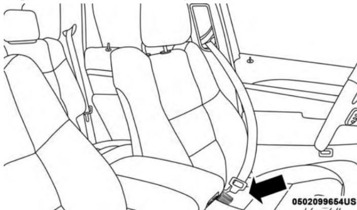
**Inserting Latch Plate Into Buckle**
