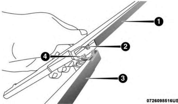
Wiper Blade Removed From Wiper Arm
