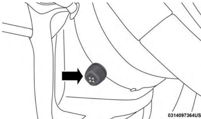
**Power Tilt/Telescoping Steering Column**
