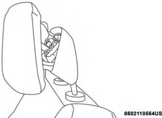
Active Head Restraint (AHR) Triggered
