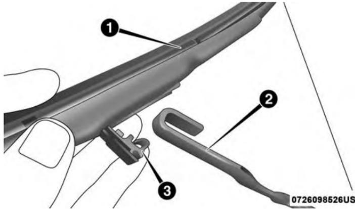
Wiper Blade Removed From Wiper Arm
