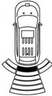
The vehicle is close to the obstacle when the warning display shows one flashing arc and sounds a continuous tone. The following chart shows the warning alert operation when the system is detecting an obstacle:
