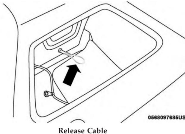
**NOTE:** If the fuel door does not latch after the manual release cable has been activated, the actuator latch should be manually returned to the closed position.
