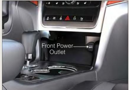
indicate how the outlet is powered. Power outlets labeled with a “key” are powered when the ignition switch is in the ON/RUN or ACC position, while the outlets labeled with a “battery” are connected directly to the battery and powered at all times.
