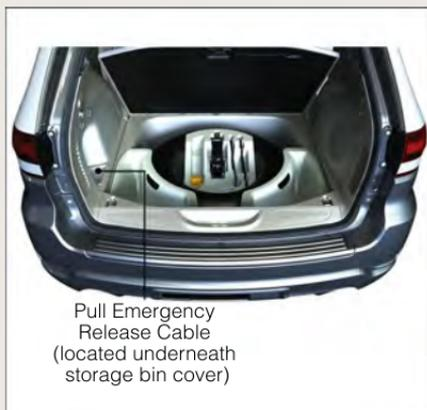
Pull Emergency Release Cable (located underneath storage bin cover)
