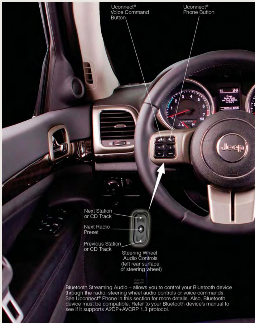
Bluetooth Streaming Audio – allows you to control your Bluetooth device through the radio, steering wheel audio controls or voice commands. See Uconnect® Phone in this section for more details. Also, Bluetooth device must be compatible. Refer to your Bluetooth device's manual to see if it supports A2DP+AVCRP 1.3 protocol.
