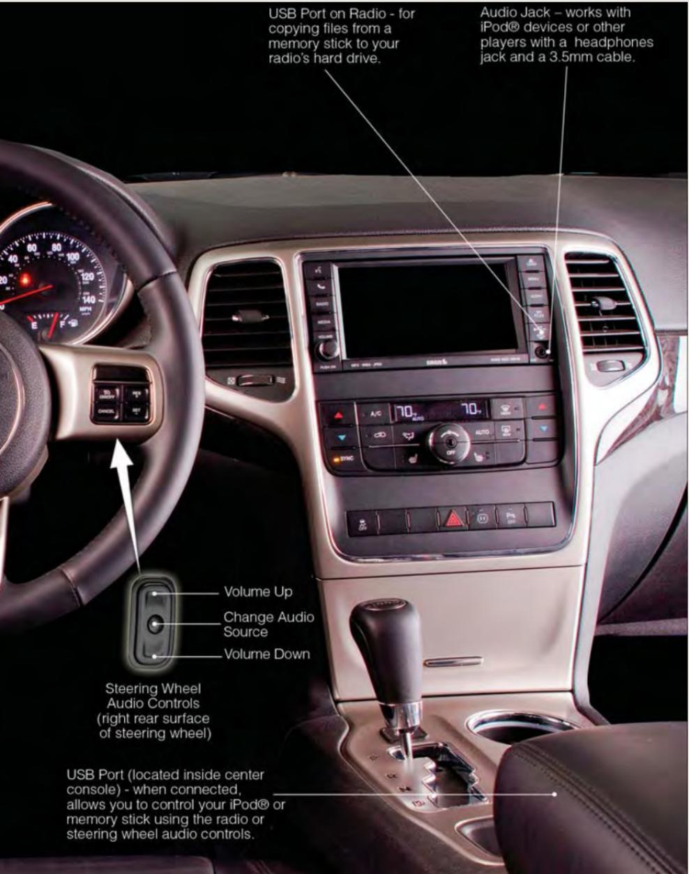
USB Port on Radio - for copying files from a memory stick to your radio's hard drive.
