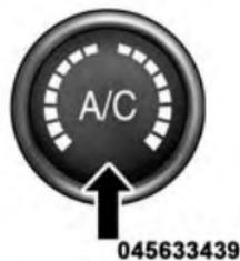
Press this button to engage the Air Conditioning. A light will illuminate when the Air Conditioning system is engaged. Rotating the dial left into the blue area of the scale indicates cooler temperatures, while rotating right into the red area indicates warmer
