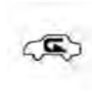
When outside air contains smoke, odors, or high humidity, or if rapid cooling is desired, you may wish to recirculate interior air by pressing the Recirculation control button. Recirculation mode should only be used temporarily. The recirculation LED will illuminate when this button is selected. Push the button a second time to turn off the Recirculation mode LED and allow outside air into the vehicle.
