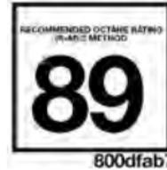
This engine is designed to meet all emissions regulations and provide satisfactory fuel economy and performance when using high-quality unleaded gasoline having an octane range of 87 to 89. The manufacturer recommends the use of 89 octane for optimum performance. The use of premium gasoline is not recommended, as it will not provide any benefit over regular gasoline in these engines.
