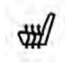
Press the switch once to select HIGH-level heating. Press the switch a second time to select LOW-level heating. Press the switch a third time to shut the heating elements OFF.
