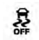
The “ESC OFF Indicator Light” indicates the Electronic Stability Control (ESC) is off.
