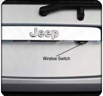
The liftgate flipper glass is unlocked when the liftgate is unlocked. To open the flipper glass, push up on the window switch located on the liftgate.
