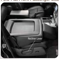
The front passenger seat can be folded flat to allow for extended cargo space. Pull up on the recliner lever to fold down the seathack
