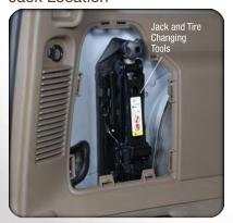
The scissor-type jack and tire changing tools are located in the left rear trim panel behind the second row seat.
