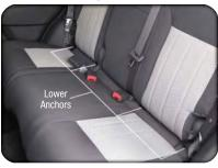
Loosen the child seat adjusters on the lower straps and tether straps so that you can attach the hook or connector to the lower and tether anchorages more easily.
