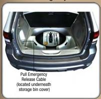
To manually open the fuel door, remove the storage bin and pull the release cable located in the rear cargo area.
