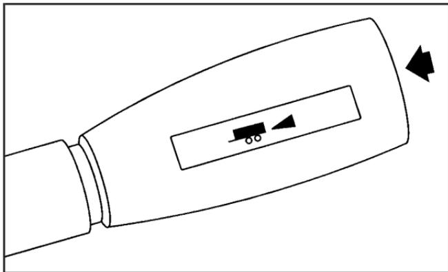
If your vehicle has an automatic transmission, it may have a Tow/Haul mode. If your vehicle has an Allison Transmission<sup>®</sup> see “Tow/Haul Mode (Allison Transmission<sup>®</sup>)” following. Tow/Haul mode adjusts the transmission shift pattern to reduce shift cycling, providing increased performance, vehicle control, and transmission cooling when towing or hauling heavy loads.
