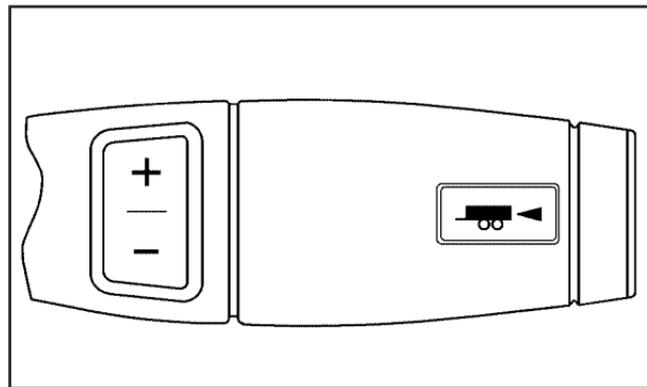
If your vehicle has an Allison Transmission<sup>®</sup>, it may have a Tow/Haul mode. Tow/Haul mode adjusts the transmission shift pattern to reduce shift cycling, providing increased performance, vehicle control, and transmission cooling when towing or hauling heavy loads.
