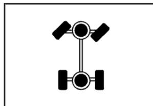
A 4WD indicator light comes on when you shift into four-wheel drive and the front axle engages. See *Four-Wheel-Drive Light* on page 3-49.
