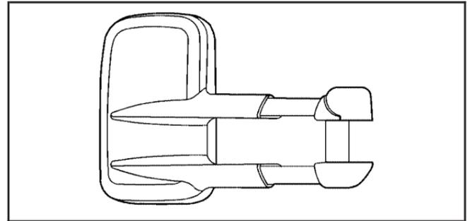
If your vehicle is equipped with this trailer towing type mirror, they can be adjusted so you can have a clear view of the objects behind you. Pull out the mirror head to extend it for better visibility when towing a trailer.
