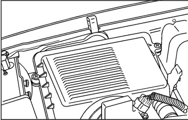
1. Locate the air cleaner/filter assembly on the front corner of the engine compartment on the passenger's side of the vehicle.
