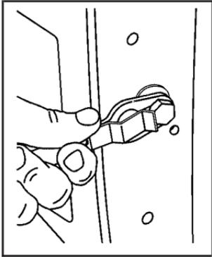
1. Raise the tailgate slightly and release both retaining cable clips. To release the retaining cable clips, lift the cable so it points straight out and push the cable clip forward.
