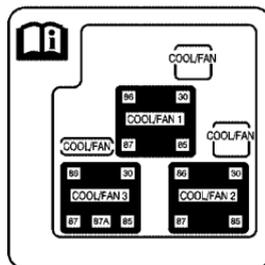
The auxiliary electric cooling fan fuse block is located in the engine compartment on the driver's side of the vehicle next to the underhood fuse block.
