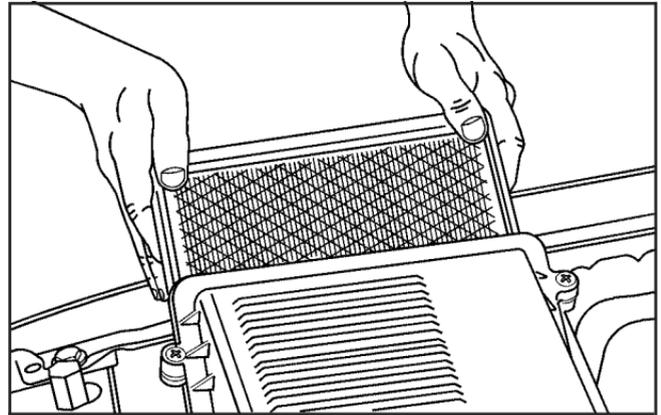
3. Remove the engine air cleaner/filter from the housing. Care should be taken to dislodge as little dirt as possible.
