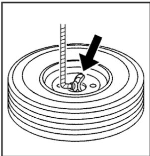
6. Tilt the retainer at the end of the cable when the tire has been lowered, so it can be pulled up through the wheel opening.
