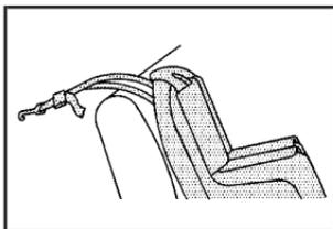
If the position you are using does not have a head restraint and you are using a dual tether, route the tether over the seatback.
