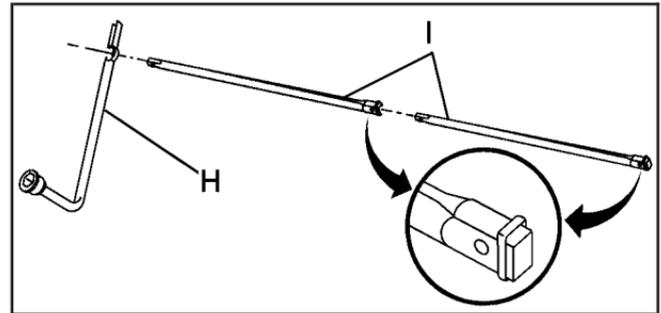
3. Attach the wheel wrench (H) and extensions (I) together.
