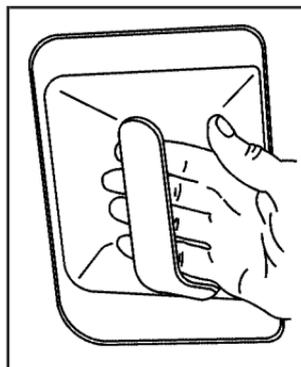
To open a rear access door from the inside, the front door must be opened first. Then, use the handle located on the inside of the rear access door to open it.
