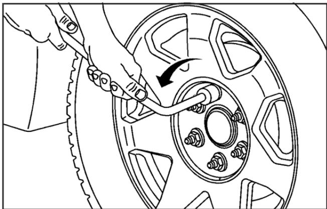
2. Use the wheel wrench and turn it counterclockwise to loosen the wheel nuts. Do not remove the wheel nuts yet.
