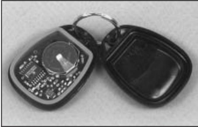
1. Insert a thin object, such as a coin, in the slot between the covers of the transmitter housing near the key ring hole. Remove the bottom by twisting the coin.
