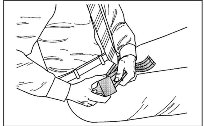
When you sit in the center front seating position, you have a lap safety belt, which has no retractor. To make the belt longer, tilt the latch plate and pull it along the belt.
