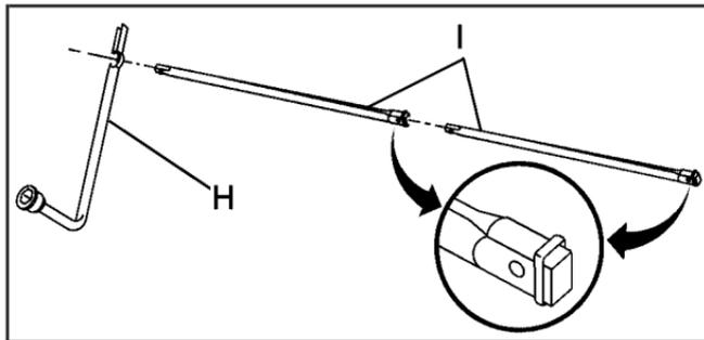
2. Assemble the wheel wrench (H) and the two jack handle extensions (I) as shown.
