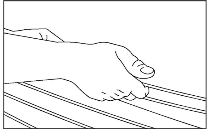
2. Then go to the front of the vehicle and pull up on the secondary hood release located near the center of the grille.
