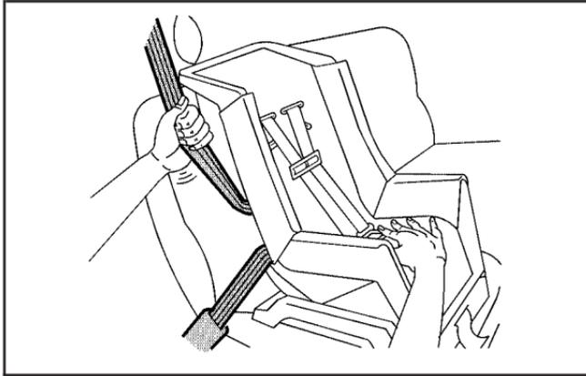
6. To tighten the belt, push down on the child restraint, pull the shoulder portion of the belt to tighten the lap portion of the belt and feed the shoulder belt back into the retractor. If you are using a forward-facing child restraint, you may find it helpful to use your knee to push down on the child restraint as you tighten the belt. You should not be able to pull more of the belt out of the retractor once the lock has been set.
