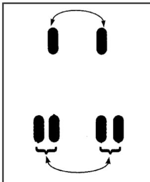
If your vehicle has dual rear wheels and the tread design for the front tires is different from the dual rear tires, always use the correct rotation pattern shown here when rotating your tires.
