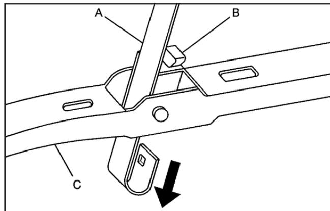
2. Push the release lever (B) to disengage the hook and push the wiper arm (A) out of the blade (C).
