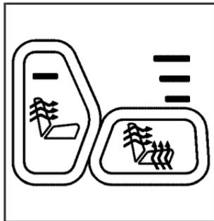
If your vehicle has this feature, the buttons are located on the front doors. The engine must be running for the heated seats to work.
