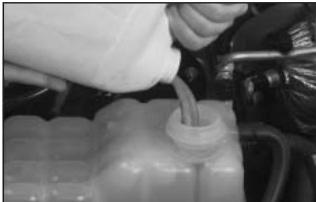
3. Fill the coolant surge tank with the proper mixture, to the FULL COLD mark.
