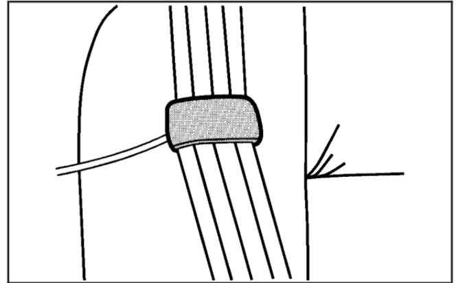
3. Be sure that the belt is not twisted and it lies flat. The guide must be on top of the belt.
