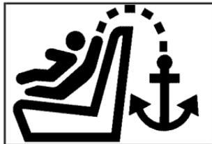
For regular and crew cab models, there is an anchor symbol on the trim covers to assist you in locating the top tether anchors.
