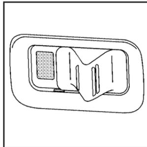
To lock the door from the inside, slide the lever rearward. To unlock the door, slide the lever forward.
