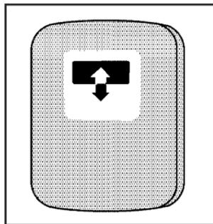
The sunroof control is located on the overhead console. Press the rear of the control to open the sunroof to the vent position, then press the rear of the control again to express-open the sunroof.
