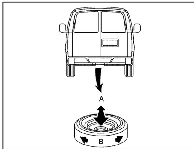
7. Make sure the tire is stored securely. Push, pull (A), and then try to turn (B) the tire. If the tire moves, use the wheel wrench to tighten the cable.
