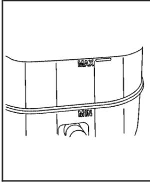
Just look at the brake fluid reservoir. The fluid level should be above MIN. If it is not, have your brake system checked to see if there is a leak.
