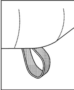
1. Push down on the front of the seat cushion while pulling down on the release strap which is located under the seat cushion.
