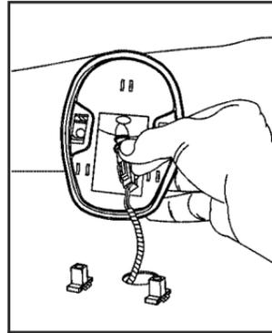
2. Install a new bulb into the socket and turn clockwise until it locks into place.
