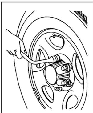
1. If your vehicle has wheel nut caps, loosen them by turning the wheel wrench counterclockwise.
