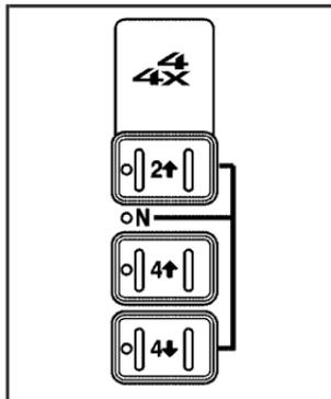
If your four-wheel-drive vehicle has the electronic transfer case, the transfer case switches are located to the left of the instrument panel cluster.
