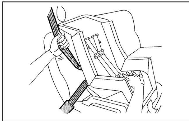
6. To tighten the belt, push down on the child restraint, pull the shoulder belt to tighten the lap belt portion and feed the shoulder belt back into the retractor. If you are using a forward-facing child restraint, you may find it helpful to use your knee to push down on the child restraint as you tighten the belt. You should not be able to pull more of the belt out of the retractor once the lock has been set.
