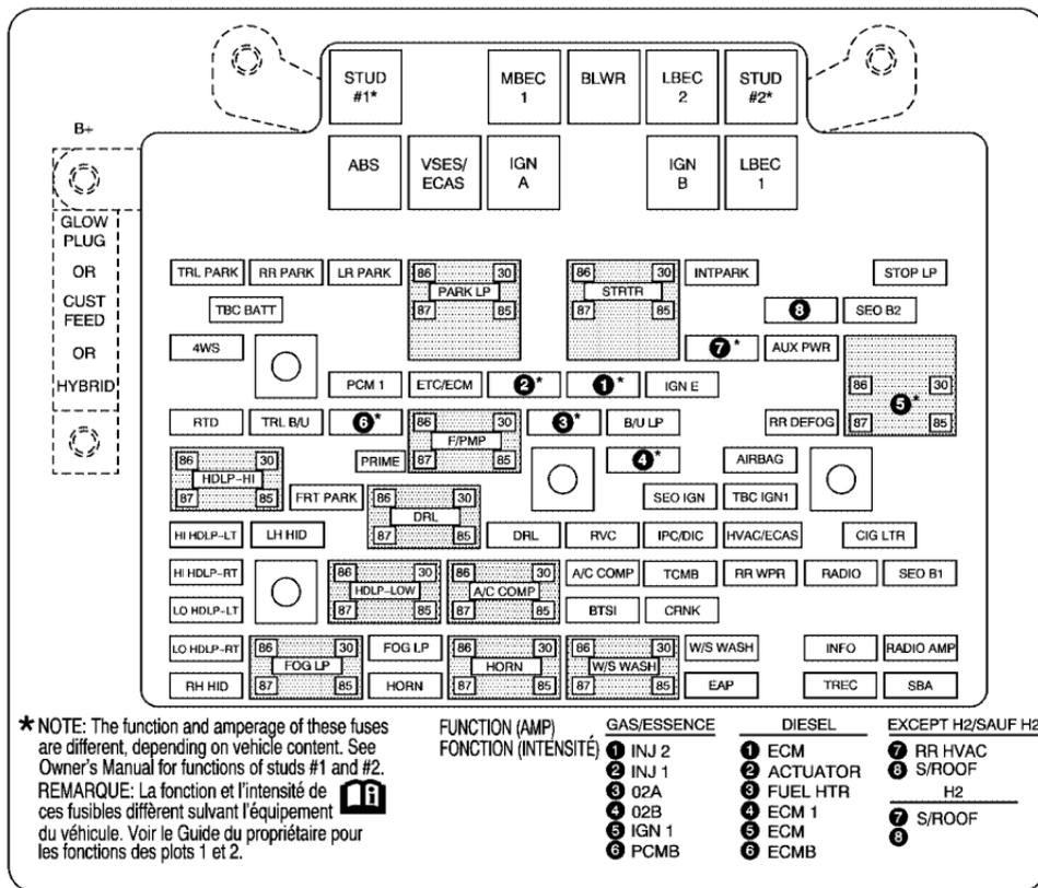
\*1 Fuel Injection Rail #2-Gasoline Engine; Engine Control Module-Diesel Engine.
