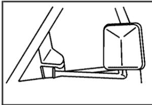
If your vehicle is equipped with this style camper-type mirrors, they can be adjusted so you can have a clear view of the objects behind you.
