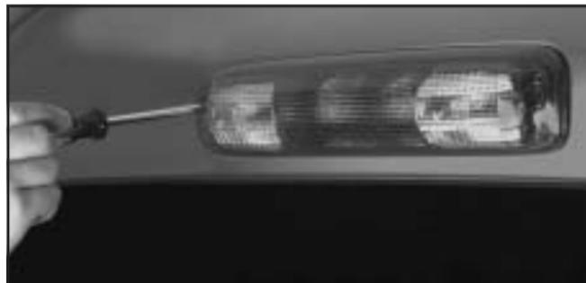
1. Remove the screws and lift off the lamp assembly.
