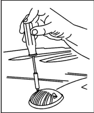
1. Remove the two screws and lift off the lens.
