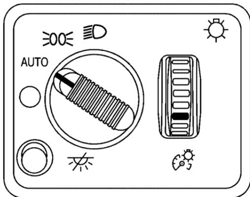
The control on the driver's side of your instrument panel operates the headlamps.
