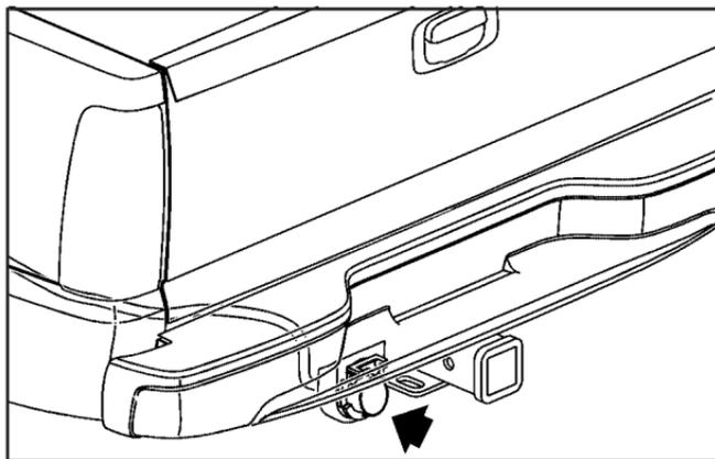
For vehicles equipped with heavy duty trailering, the harness is connected to the trailer mounted to the hitch platform. The eight-wire harness contains the following trailer circuits:
