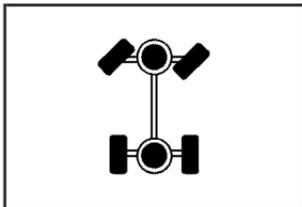
The four-wheel-drive indicator will light up when you shift a manual transfer case into four-wheel drive and the front axle engages.
