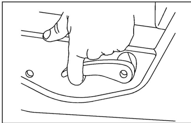
To adjust the seatback, lift the manual lever located on the outboard side of the seat. Release the lever to lock the seatback in the desired position. Lift the lever again without pushing on the seatback and the seatback will go to an upright position.
