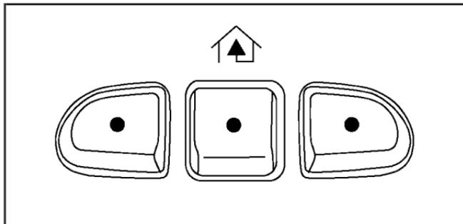
The Universal Home Remote System, a combined universal transmitter and receiver, provides a way to replace up to three hand-held transmitters used to activate devices such as gate operators, garage door openers, entry door locks, security systems, and home lighting.
