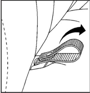
1. Pull up on the strap loop at the rear of the seat cushion. Then, pull the seat cushion up and flip it forward.
