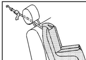
If the position you are using has an adjustable head restraint and you are using a single tether, raise the head restraint and route the tether under the head restraint and in between the head restraint posts.
