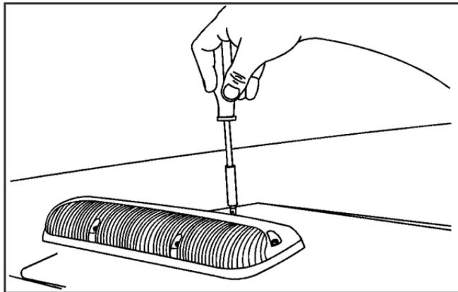
1. Remove the six screws from the center roof marker lamp assembly.
