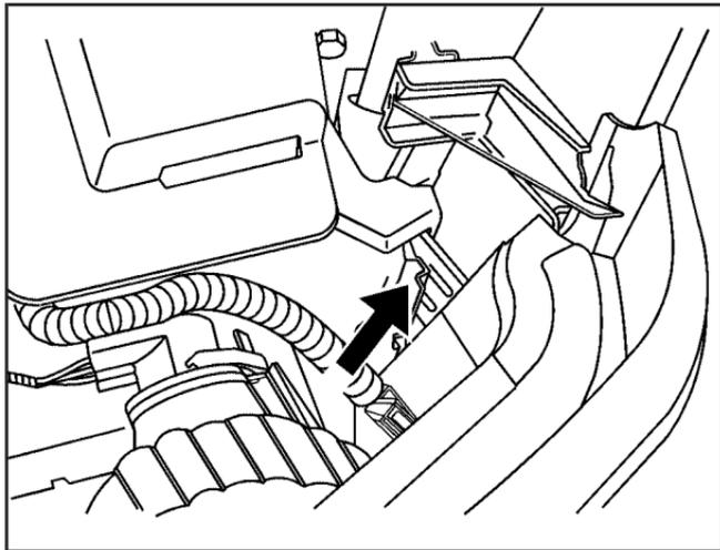
2. Press the retainer clip (arrow), located behind the turn signal assembly, towards the outside of the vehicle.
