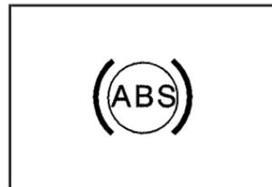
If there is a problem with the anti-lock brake system, this warning light will stay on. See *Anti-Lock Brake System Warning Light* on page 3-42.
