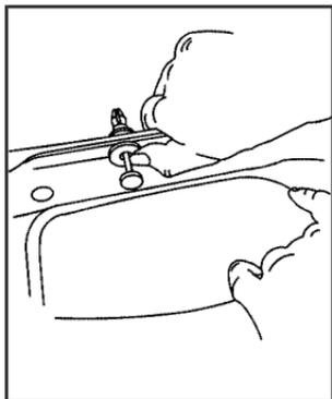
1. Line up each push-pin with its intended retainer and push the washer portion of the push-pin toward the retainer until it locks into place.
