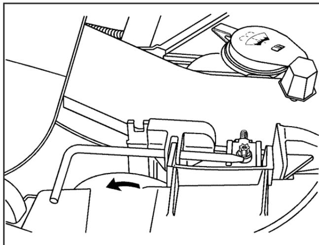
2. Remove the pin on the headlamp assembly by turning the pin up and pulling it straight out.
