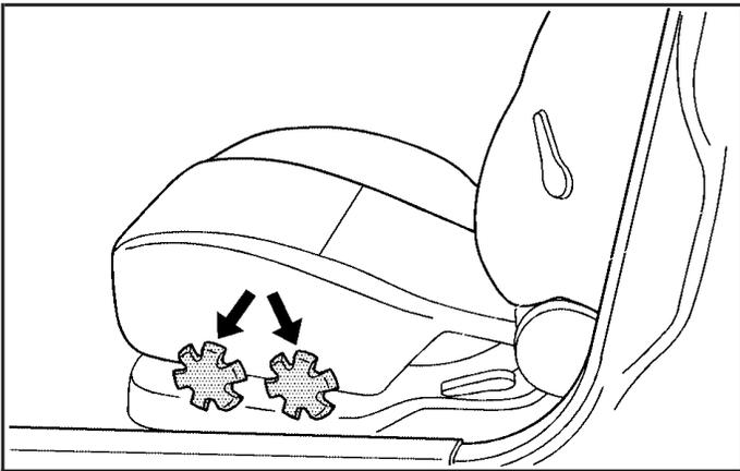
The manual drivers seat tilt adjuster knobs are located on the outboard side of the seat cushion.
