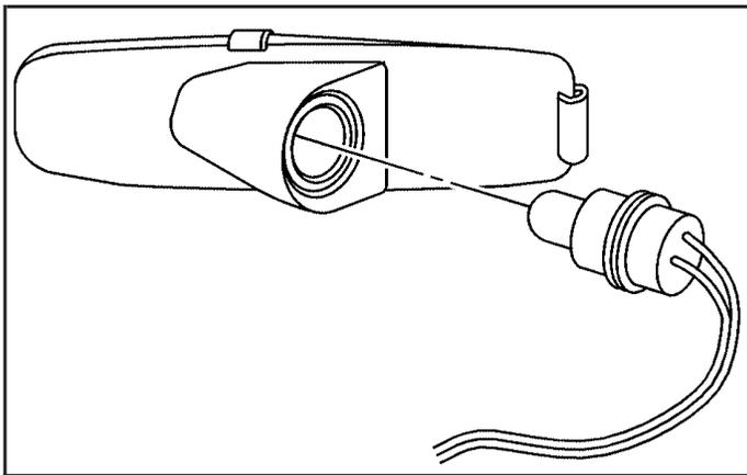
5. Pull the old bulb straight out of the bulb socket.
