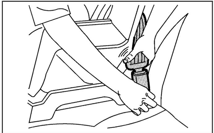
3. Buckle the belt. Be sure the latch plate clicks when you put it into the buckle. This means you are using the correct buckle. Also, make sure the release button is positioned so you would be able to unbuckle the safety belt quickly if you ever had to.
