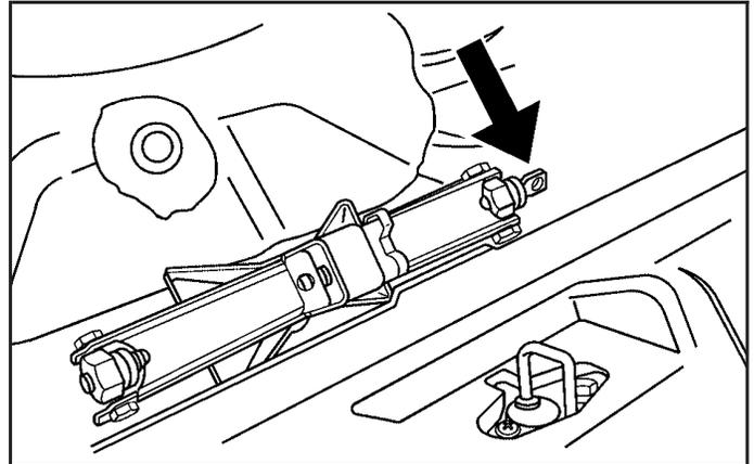
6. Remove the jack by turning the jack retainer, located on the right side of the jack, counterclockwise to release it. The jack is located in the trunk, in front of the compact spare tire.
