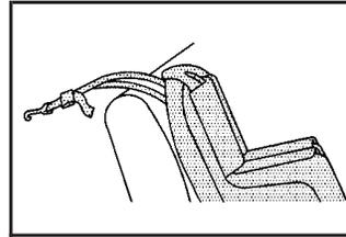
If the position you are using does not have a head restraint and you are using a dual tether, route the tether over the seatback.
