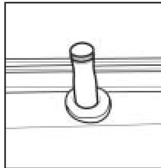
All doors, except for the driver's door, can be locked from the outside by pushing down the manual door lock and then closing the door.
