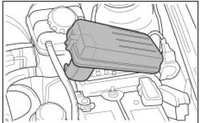
The engine compartment fuse block is located on the driver's side of the vehicle, near the battery. See *Engine Compartment Overview* on page 5-12 for more information on location. To access the fuses, press in the top flap to release the cover.
