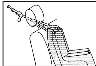
If the position you are using has a head restraint and you are using dual tether, route the tether under the head restraint and in between the head restraint posts.
