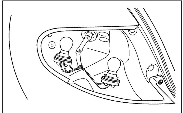
3. Remove the bulb socket by turning it counterclockwise from the taillamp assembly.
