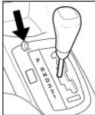
4. Insert the key into the shift-lock release slot and press and hold the key.
