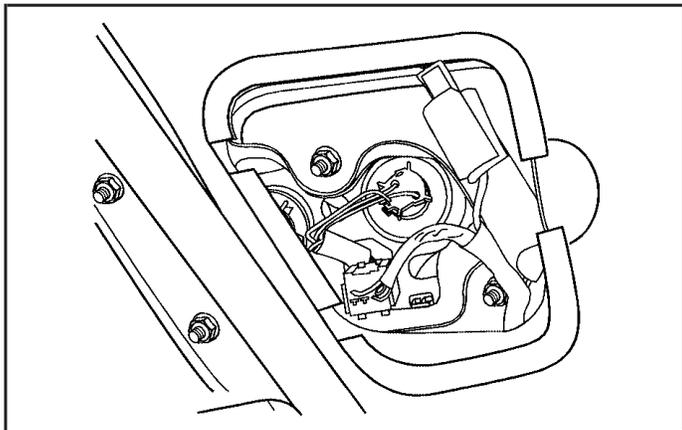
3. Remove the bulb socket by turning it counterclockwise.
