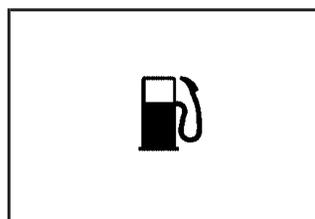
This light comes on when the fuel tank is low on fuel.
