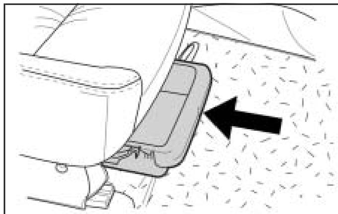
Your vehicle may have a sliding storage tray located under the front passenger seat. To use the tray, pull up on the end of the tray and pull it toward the instrument panel. Push the tray toward the seat to return it to its original position.
