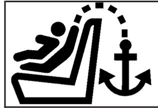
To assist you in locating the top tether anchors, the top tether anchor symbol is located on the trim cover, if equipped.
