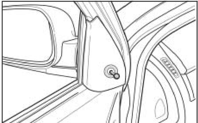
Adjust the outside mirrors with the control levers on the driver's and passenger's doors.
