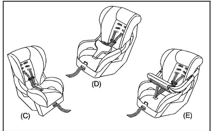
A forward-facing child seat (C-E) provides restraint for the child's body with the harness and also sometimes with surfaces such as T-shaped or shelf-like shields.
