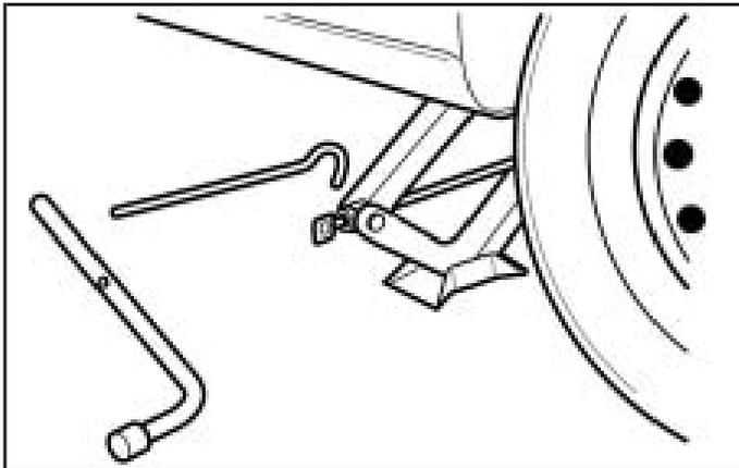
5. Insert the jack handle into the jack and the wheel wrench onto the end of the jack handle.
