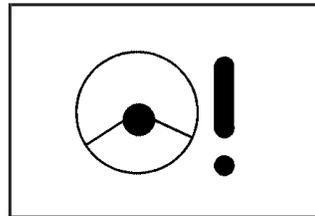
If your vehicle has Speed Sensitive Power Steering, this warning light will come on briefly when you turn the ignition to ON as a check to show you it is working.
