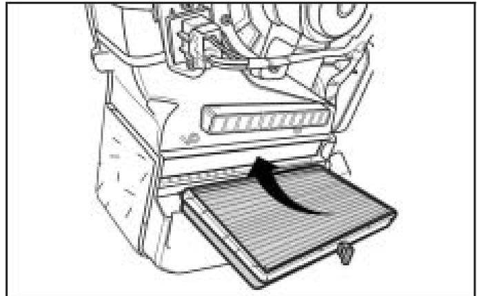
3. Remove the old passenger compartment air filter.
