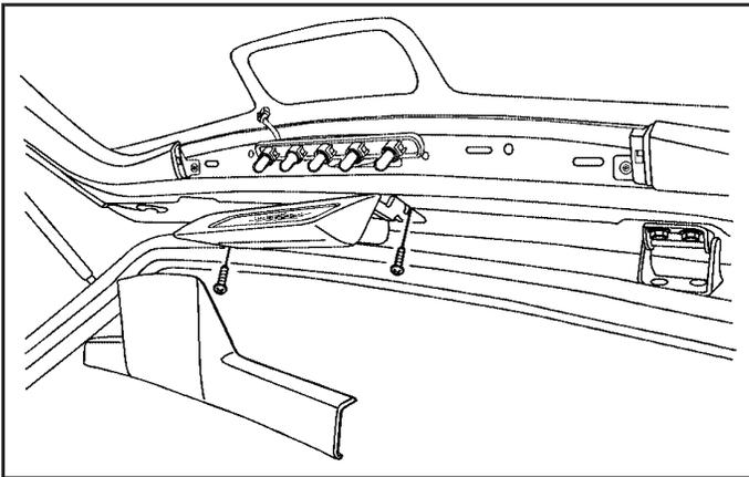
2. Pry off the trim from the liftgate and remove the two screws.
