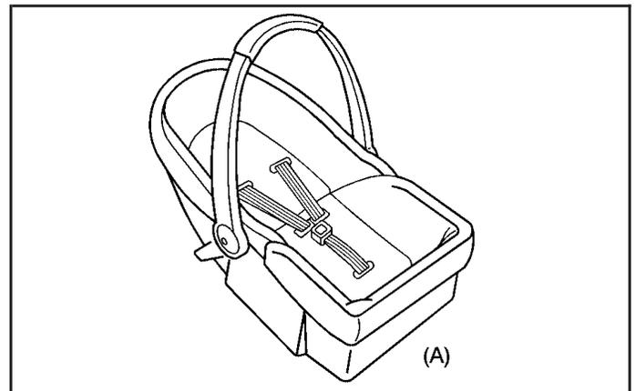
An infant car bed (A), a special bed made for use in a motor vehicle, is an infant restraint system designed to restrain or position a child on a continuous flat surface. Make sure that the infant's head rests toward the center of the vehicle.
