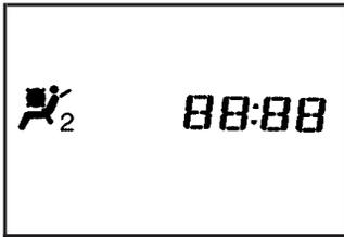
The passenger sensing system will turn off the right front passenger's frontal airbag and side airbag (if equipped) under certain conditions.
