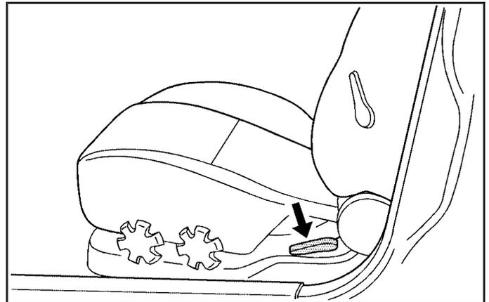
Your seats have manual reclining seatbacks. The lever used to operate them is located on the outboard side of the seats.
