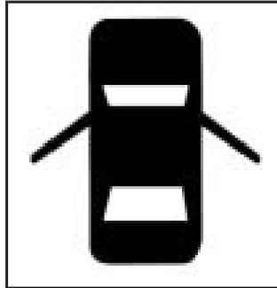
If one of the doors on your vehicle is not closed properly while the ignition is on, the door ajar light on the instrument panel cluster will come on and stay on until the doors are closed. See *Door Ajar Light* on page 3-42 for additional information.
