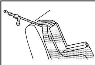
If the position you are using does not have a head restraint and you are using a single tether, route the tether over the seatback.
