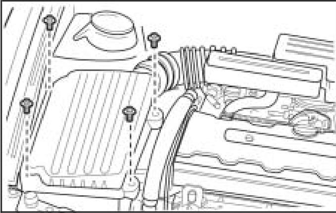
1. Remove the four screws that hold the cover on.
