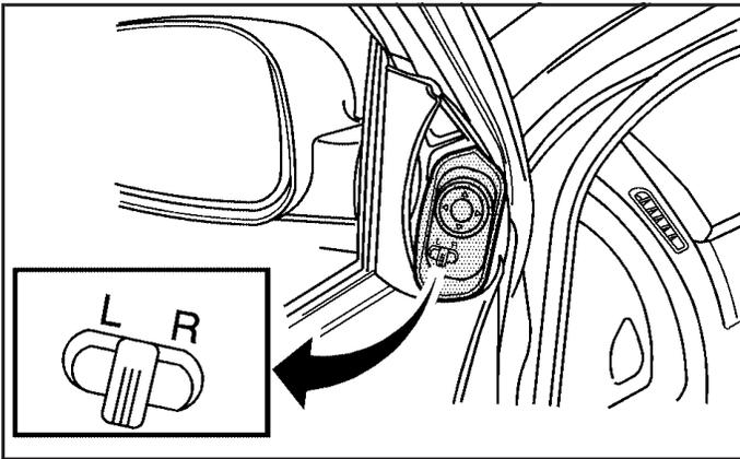
Your vehicle may have outside power mirrors. The control for the power mirrors is located on the driver's side door trim.
