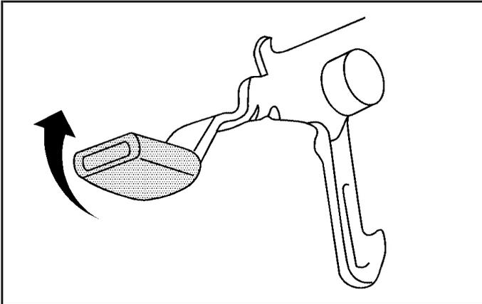
2. Then go to the front of the vehicle and lift up the secondary hood release lever. The secondary hood release lever is located under the front center of the hood.
