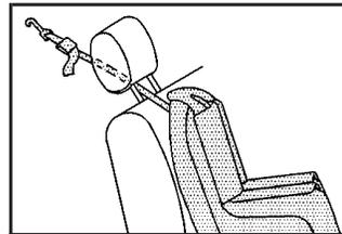
If the position you are using has a head restraint and you are using a single tether, route the tether under the head restraint and in between the head restraint posts.
