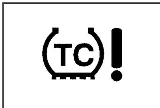
If your vehicle has the Traction Control System (TCS), this light comes on for a few seconds when the ignition is turned to ON.
