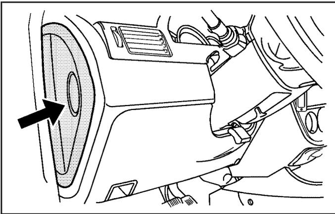
The instrument panel fuse block is located on the end of the instrument panel, on the driver's side of the vehicle. To access the fuses, open the fuse panel door by pulling out.
