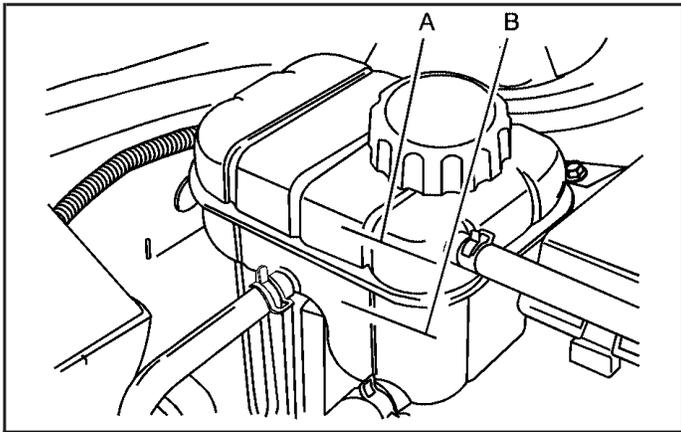
The engine coolant surge tank is located in the rear of the engine compartment on the driver's side. See *Engine Compartment Overview* on page 5-12 for more information on location.
