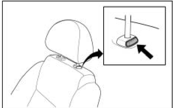
Push in the release button at the base of the head restraint and push the restraint down to lower it.
