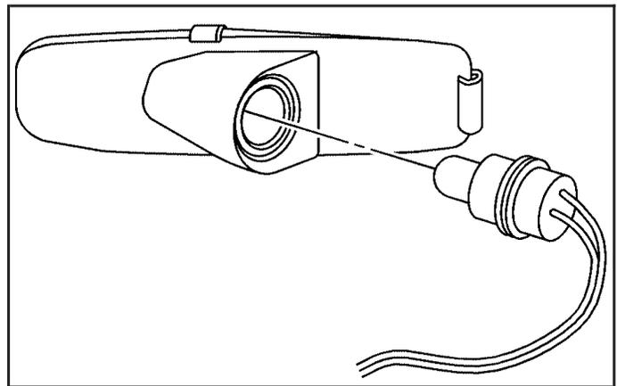
2. Turn the rear sidemarker bulb socket counterclockwise.
