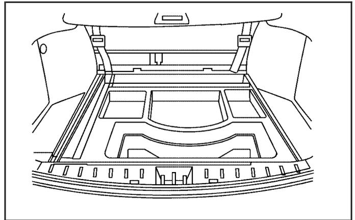
There are various bins under the luggage compartment floor. To access the bins, pull floor mat handle upward.
