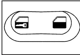
With the power door locks, you can unlock or lock the doors on your vehicle using the driver's door lock switch.
