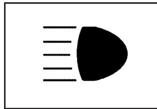
When the high beams are on, a light on the instrument panel cluster also will be on if the ignition is turned to ON.
