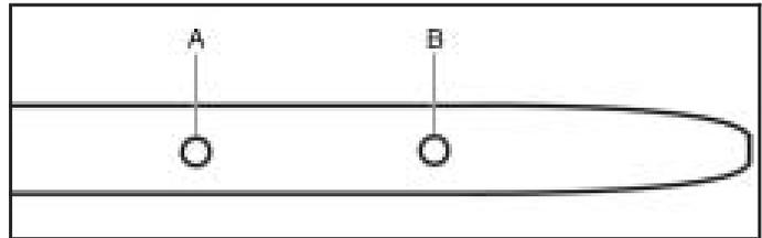
If the oil is below the lower hole at the tip of the dipstick (B), you will need to add at least one quart/liter of oil. But you must use the right kind. This section explains what kind of oil to use. For engine oil crankcase capacity, see *Capacities and Specifications on page 5-88*.
