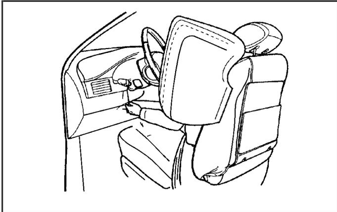
If your vehicle has one, the driver's side impact airbag is in the side of the driver's seatback closest to the door.
