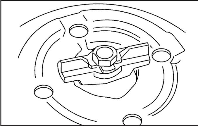
5. Turn the retainer on the compact spare tire counterclockwise and remove the retainer.
