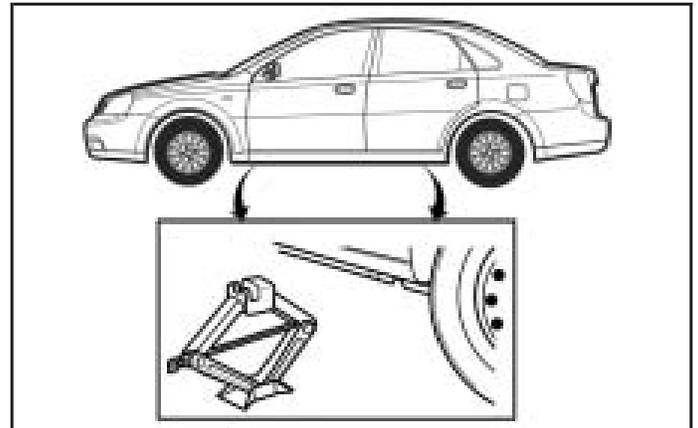
3. Locate the notch near each wheel in the frame which the jack head fits in.
