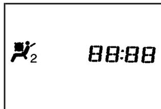
When the ignition key is turned to ON or START, the passenger airbag status indicator will light for several seconds as a system check.
