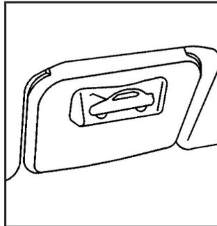
1. Pull the hood release handle inside the vehicle. It is located on the lower left side of the instrument panel.
