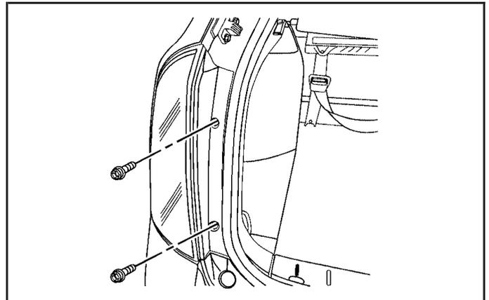
2. Remove the two screws from the taillamp assembly.
