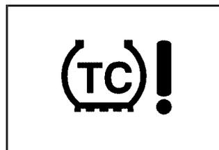
This light will come on briefly when the ignition is turned to ON along with the anti-lock brake system warning light.
