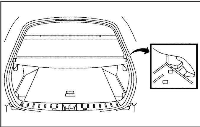
Your vehicle is equipped with a cargo shade. Pull the handle of the shade toward you and insert the retainer into the slot located on both sides of the tailgate openings. To remove the shade, release the handle after pulling it toward you a little. The shade will retract automatically.
