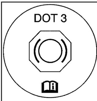
Your master cylinder reservoir is filled with DOT-3 brake fluid. See *Engine Compartment Overview on page 5-12* for the location of the reservoir.
