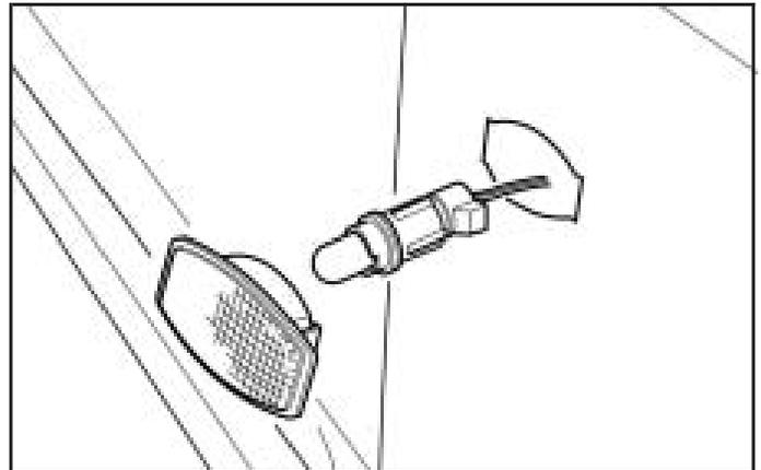
4. Remove the bulb from the lamp housing by pulling the bulb straight out of the socket.
