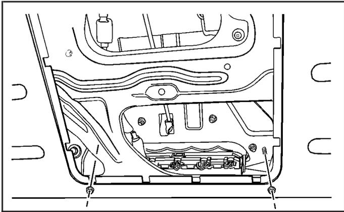
2. Remove the two screws and the liftgate trim cover.
