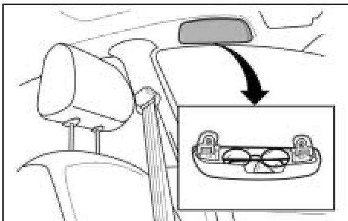
The sunglasses storage compartment is located above the driver's door. To open the sunglasses storage compartment, pull down and hold the upper part of the cover. To close the compartment, let go of the cover and the compartment will automatically close.
