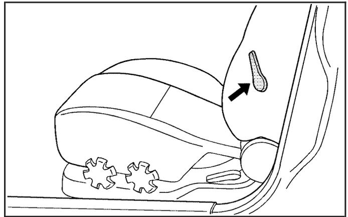
To adjust the front seat lumbar support, use the lever located on the outboard side of the seatback.
