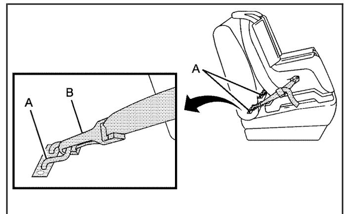
Lower anchors (A) are metal bars built into the vehicle. There are two lower anchors for each LATCH seating position that will accommodate a child restraint with lower attachments (B).
