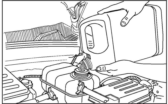
3. Fill the coolant surge tank with the proper mixture to the Maximum mark on the coolant surge tank. Wait about five minutes, then check to see if the level is below the mark. If the level is below the Maximum mark, add additional coolant to bring the level up to the mark. Repeat this procedure until the level remains constant at the Maximum mark for at least five minutes.
