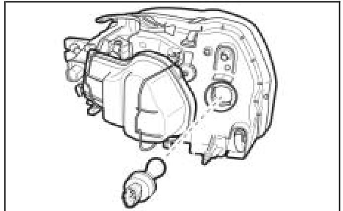
5. Turn the front turn signal bulb socket counterclockwise. Pull the front turn signal bulb socket out of the lamp housing.
