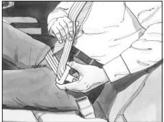
If the belt stops before it reaches the buckle, tilt the latch plate and keep pulling until you can buckle it. Pull up on the latch plate to make sure it is secure. Make sure the release button on the buckle is positioned so you would be able to unbuckle the safety belt quickly if you ever had to.
