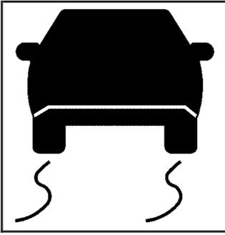
If your vehicle has the Traction Control System (TCS), the TCS active light comes on for a few seconds when the ignition is turned to ON.
