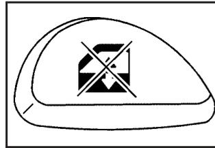
The driver's power window controls also include a lockout button.
