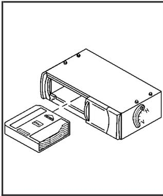
To eject the magazine from the player, press the eject button. The magazine will automatically eject.
