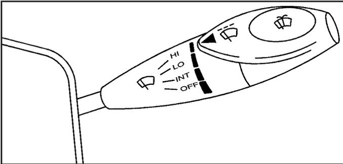
Use this lever located on the right side of the steering wheel to operate the windshield wipers. The ignition must be turned to ON to operate the windshield wipers.
