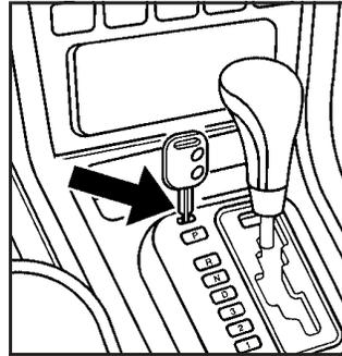
4. Insert the key into the shift-lock release slot and press and hold the key.
