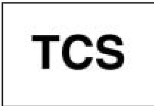
This light will come on briefly when the ignition is turned to ON along with the anti-lock brake system warning light.
