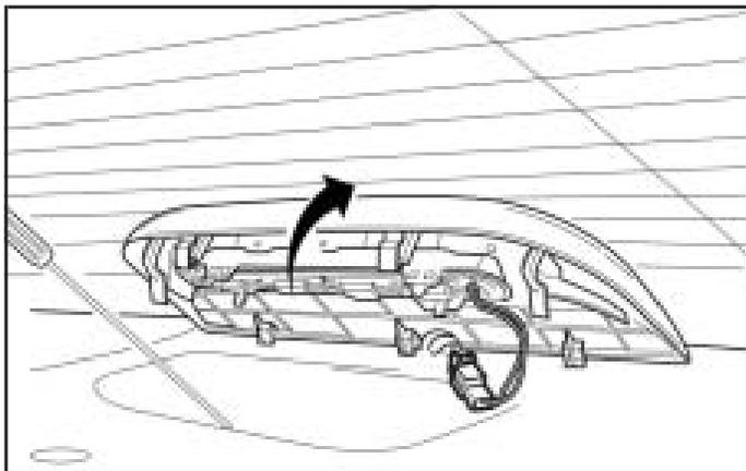
2. Pry off the lamp housing with a flat tool.
