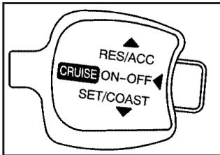
The cruise control lever is located on the right side of the steering wheel.
