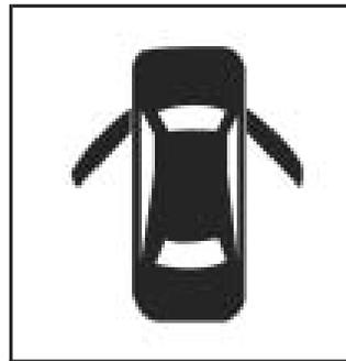
If one of the doors on your vehicle is not closed properly, the door ajar light on the secondary information center will come on and stay on until the doors are closed.
