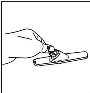
1. Reach in the underside of the front bumper and turn the bulb socket counterclockwise.
