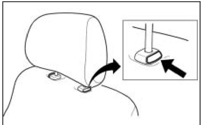
Push in the release button on the head restraint in order to adjust the position downward.
