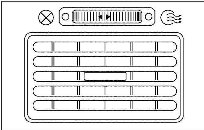
Use the lever located in the center of each outlet to change the direction of the airflow. Use the thumbwheel located above the side outlets to turn them on and off.
