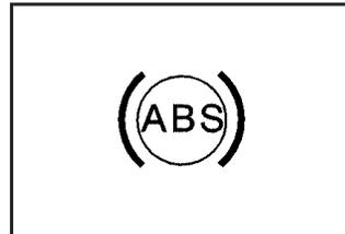
If there is a problem with the anti-lock brake system, this warning light will stay on. See *Anti-Lock Brake System Warning Light* on page 3-36.
