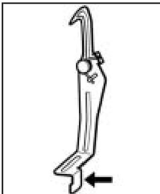
2. Then go to the front of the vehicle and locate the secondary hood release lever under the front center of the hood.
