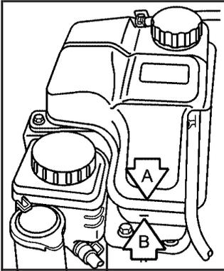
The coolant level should be between the MIN (B) and MAX (A) marks on the coolant surge tank when the engine is cool.
