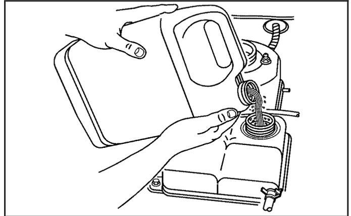
3. Fill the coolant surge tank with the proper mixture to the MAX (A) mark on the coolant surge tank. Wait about five minutes, then check to see if the level is below the MAX (A) mark. If the level is below the MAX (A) mark, add additional coolant to bring the level up to the MAX (A) mark. Repeat this procedure until the level remains constant at the MAX (A) mark for at least five minutes.
