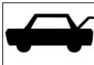
This light will come on when the trunk is not completely closed.
