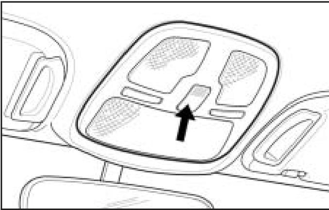
To open the sunroof to the vent position, first manually open the sunroof shade and then push the front part of the sunroof switch. To return the sunroof to its original position, push the rear part of the switch and hold it until the sunroof reaches the desired position.
