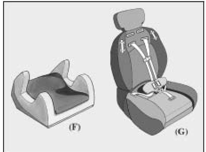
A booster seat (F-G) is a child restraint designed to improve the fit of the vehicle's safety belt system. Some booster seats have a shoulder belt positioner, and some high-back booster seats have a five-point harness. A booster seat can also help a child to see out the window.
