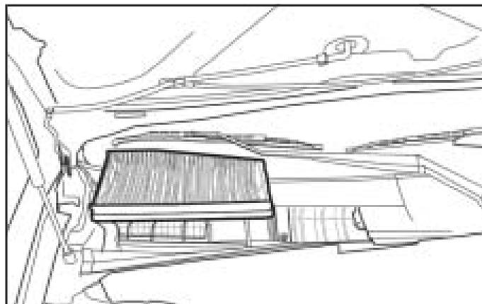
3. Remove the old passenger compartment air filter.
