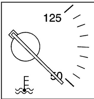
Your vehicle has an engine coolant temperature gage. With the ignition turned to ON, this gage shows the engine coolant temperature.
