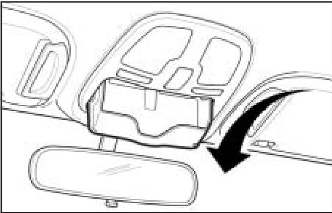
The sunglasses storage compartment is located on the headliner. To open the sunglasses storage compartment, press the rear part of the cover. To close the compartment, pull up and push it until it latches.
