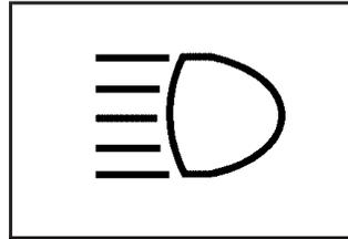
When the high beams are on, this light on the instrument panel cluster also will be on if the ignition is turned to ON.
