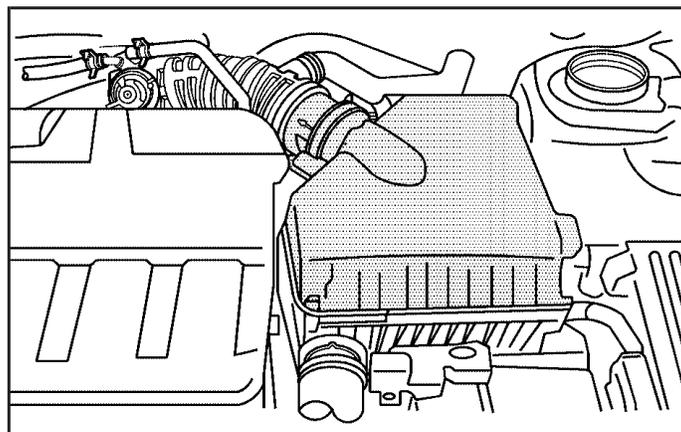
The engine air cleaner/filter is located in the engine compartment on the driver's side of the vehicle, near the battery. See *Engine Compartment Overview* on page 5-12 for more information on location.
