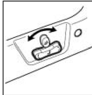
Adjust the angle of the seatback by pushing the upper switch forward or rearward.
