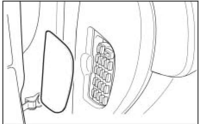
The instrument panel fuse block is located on the driver's side end of the instrument panel. To access the fuses, grip the back end of the fuse panel door and open by pulling the cover out.
