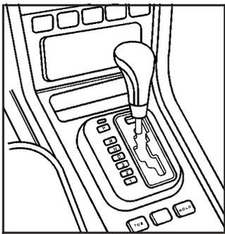
The automatic transaxle has a shift lever located on the console between the seats.
