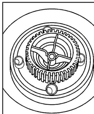
2. Turn the retainer on the spare tire counterclockwise and remove the retainer.
