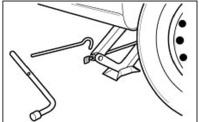
4. Insert the jack handle into the jack and the wheel wrench onto the end of the jack handle.
