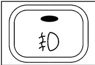
The button for the fog lamps is located on the center of the instrument panel, above the front ashtray.
