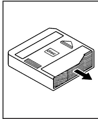
To remove the CD trays, press the CD tray button of the tray that you want to load, and carefully pull the tray out.
