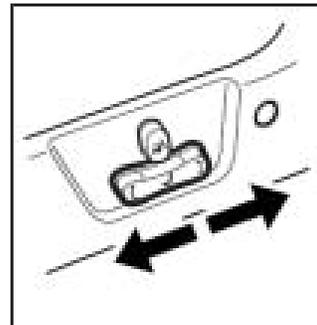
Move the seat forward or rearward by pushing and holding the switch toward the front or rear of the vehicle.
