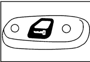
With the power door locks, you can unlock or lock the doors on your vehicle using either the driver's or front passenger's door lock switch.
