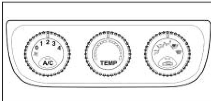
**Fan:** Turn the left knob clockwise or counterclockwise to increase or decrease the fan speed. In any setting other than off, the fan will run continuously with the ignition on. The fan must be on in order for the air conditioning compressor to run.
