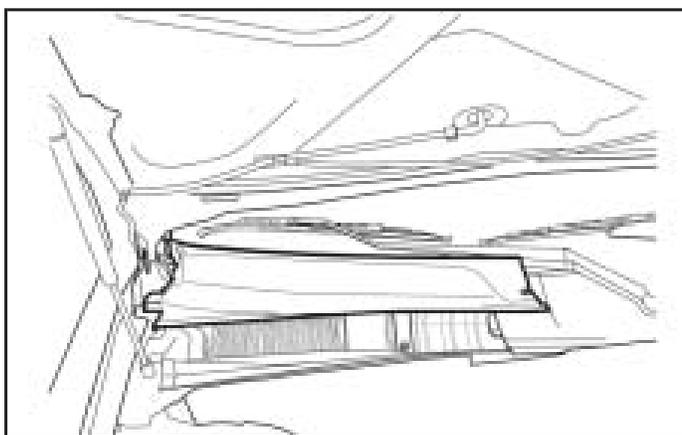
2. Unscrew and remove the three clips and the access panel.
