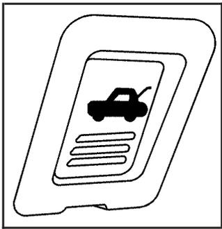
Press the remote trunk release button, located on the driver's door trim, to release the trunk lid.
