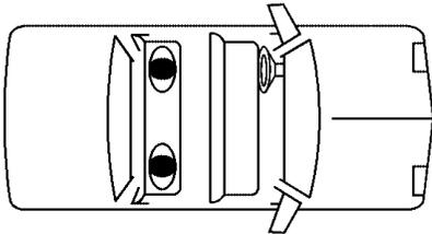
Your vehicle has the LATCH system. You will find anchors (A) for the rear outside seating positions.
