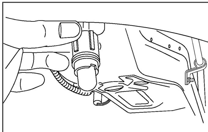
3. Pull the old bulb straight out of the socket.
