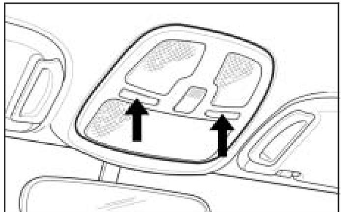
The map lamps are located on the headliner. To turn on a lamp, press the button next to it. Press the button again to turn the lamp off.
