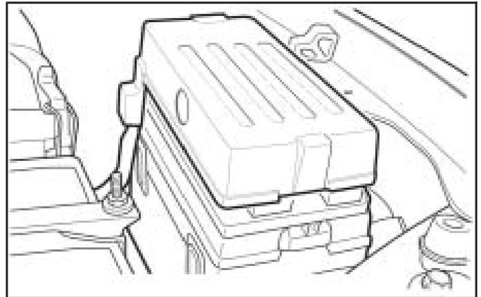
The engine compartment fuse block is located on the driver's side of the vehicle, near the battery. See *Engine Compartment Overview* on page 5-12 for more information on location. To access the fuses, press the top and bottom flaps to release the cover.
