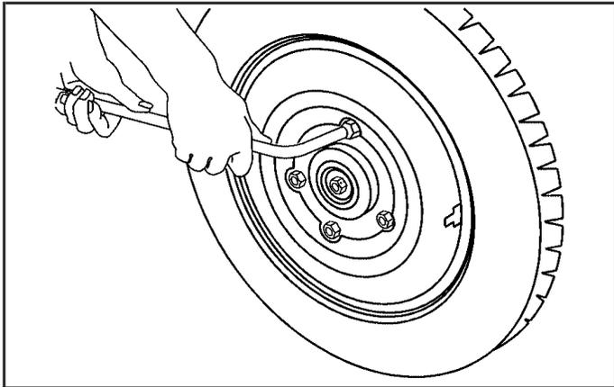
2. Then use the wheel wrench to loosen all the wheel nuts. Do not remove them yet.
