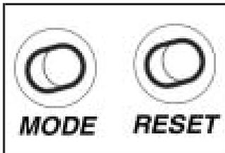
The trip odometer buttons are located to the right of the steering wheel above the ignition switch.
