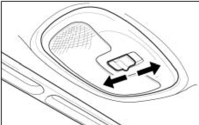
The switch on the dome lamp has three positions. The ON position will turn on the lamp. The lamp will stay on until it is manually turned off. The door, or middle, position will turn on the lamp whenever a door is opened.
