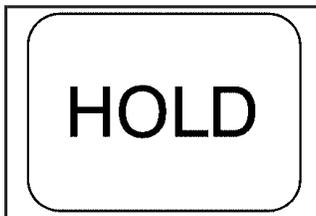
Press the HOLD button on the console below the shift lever to turn on hold mode.
