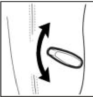
To adjust the driver's front seat lumbar support, use the lever located on the outboard side of the driver's seatback.
