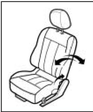
To adjust the seatback, lift the lever located on the outboard side of the seat cushion and move the seatback to where you want it.
