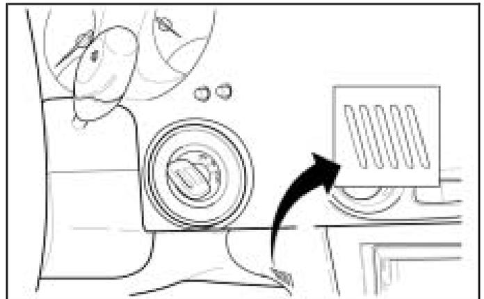
There is also a temperature sensor located beside the audio system on the driver's side of the vehicle. This sensor reads the inside air temperature and helps to establish ventilation system requirements while operating in AUTO mode. Do not cover the temperature sensor or the system will not work properly.
