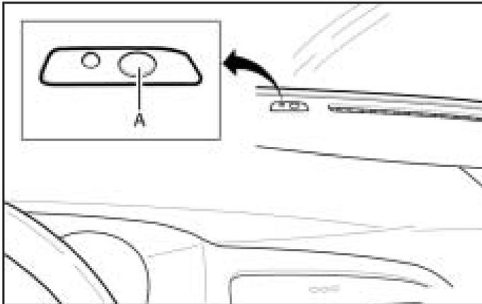
The solar sensor (A) on your vehicle monitors solar radiation and uses the information to maintain the selected temperature by initiating needed adjustments to the temperature, the fan speed and the air delivery system. Do not cover the solar sensor located in the center of the instrument panel, near the windshield, or the system will not work properly.
