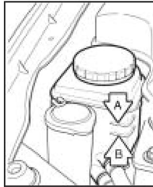
The level should be between the MIN (B) and MAX (A) marks.
