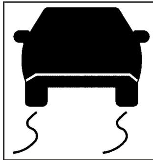
This light will come on briefly when the ignition is turned to ON along with the anti-lock brake system warning light. This light will blink when your Traction Control System is limiting wheel spin.
