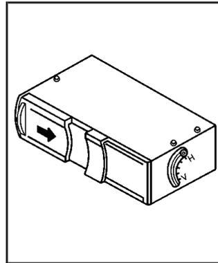
Slide the door open, in the direction of the arrow, of the CD changer.
