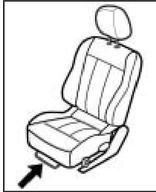
Pull up and hold the bar located under the front of the seat to unlock it.
