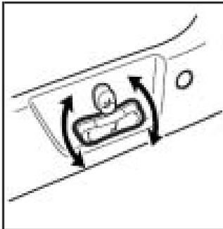
Raise or lower the front of the seat cushion by pushing the front part of the switch up or down.
