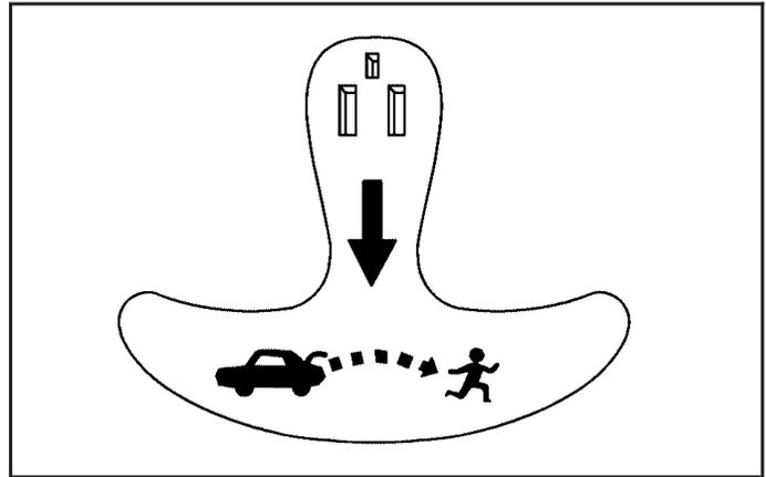
There is a glow-in-the-dark emergency trunk release handle located on the underside of the trunk lid. This handle will glow following exposure to light. Pull the release handle down to open the trunk from the inside.
