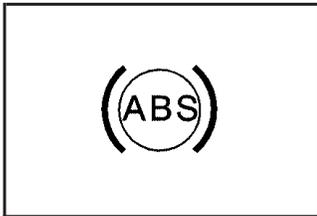
If your vehicle has an anti-lock brake system, this light will come on when the ignition is turned to ON and may stay on for several seconds. That is normal.
