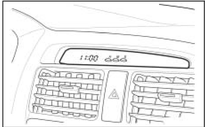
**H (Hour):** To go forward one hour, press the H button once. To go forward more than one hour, press and hold the button until the correct hour is reached.
