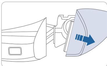
a) Use the manual key from the FOB to push up the under the driver's side handle as shown. Make sure the tab stays up. If it does not you will need to keep it pressed up while performing the next step.
