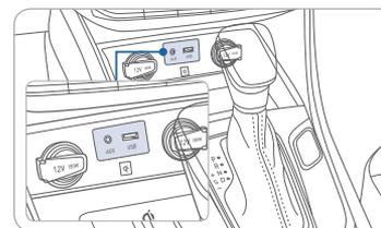
Use the input jack to connect an external audio device and listen to it through the audio system in your vehicle.
