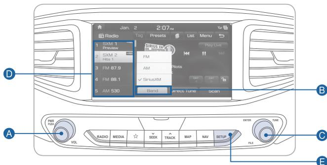
Press POWER button **A** to turn radio on.
