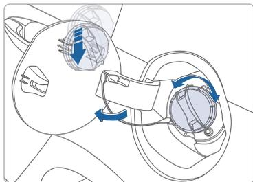
2. Remove the fuel tank cap.
