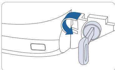
b) While holding the handle out, pull off the access cover to expose the manual lock cylinder.
