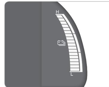
This gauge indicates the remaining hybrid battery power. If the SOC is near the "L (Low)" level, the vehicle automatically operates the engine to charge the battery.
