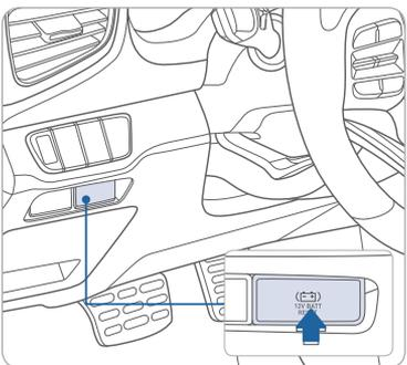
This vehicle does not have a replaceable 12V flooded lead acid battery. The 12V battery is integrated into the lithium high voltage battery assembly. Is it automatically protected against vehicle current draw when a minimum level of 12.8V 10% SOC level is reached. The 12V Battery Reset Switch has to be activated in order to start the vehicle. This should negate the need to jump start the car.
