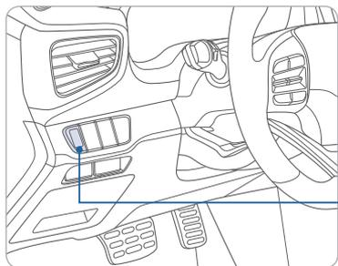
Press the illumination control button to adjust the instrument cluster illumination brightness.
