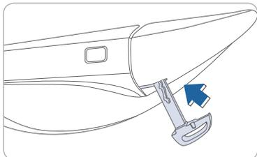
If the door is locked you will need to use the manual key to enter the vehicle after removing the lock access cover.
