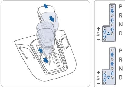
(↔): Depress the brake pedal and press the shift button while moving the shift lever.
