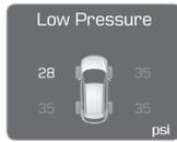
Low Tire Pressure Monitor with Location Indicator (Shown on the LCD display)
