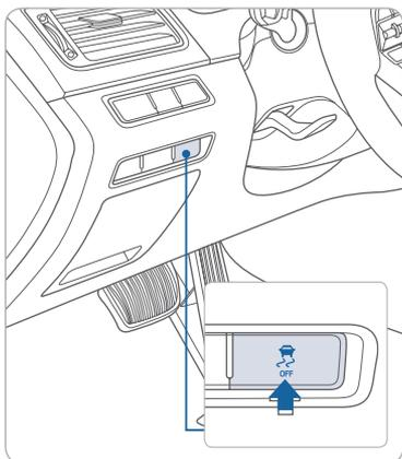
The ESC system is an electronic system designed to help the driver maintain vehicle control under adverse conditions.
