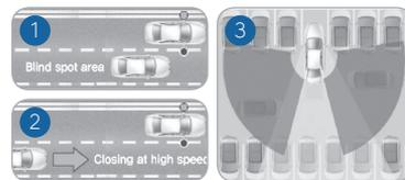
The BSD (Blind Spot Detection) system uses a radar sensor to alert the driver while driving. It senses the rear side territory of the vehicle and provides information to the driver.
