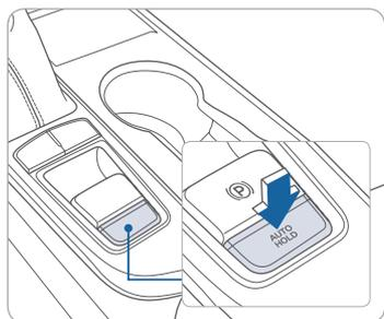
When the vehicle reaches a stop, Auto Hold keeps the vehicle stopped even when the brake pedal is released. The brakes are released automatically when the accelerator pedal is pressed.
