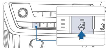
Pressing the heated steering wheel button warms the steering wheel. The indicator on the button is illuminated.
