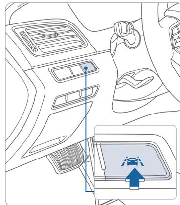
The Lane Departure Warning System detects the lane on the road and warns the driver if the vehicle leaves the lane when the vehicle speed is over 37mph.
