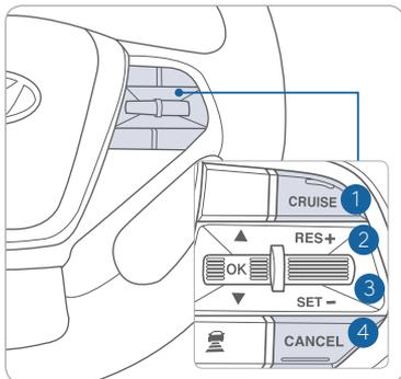
The Cruise Control system allows you to program the vehicle to maintain a constant speed without holding the accelerator pedal.
