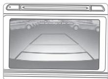
When transmission is shifted into R (Reverse), rearview camera displays the area behind the vehicle.
