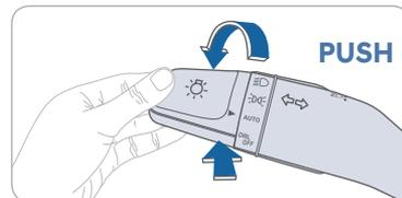
**NOTE:** To turn off high beam, pull the lever towards you.
