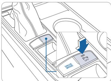
The rear parking assist system assists the driver during reverse movement of the vehicle by chiming if any object is sensed within the distance of 47 inch behind the vehicle.
