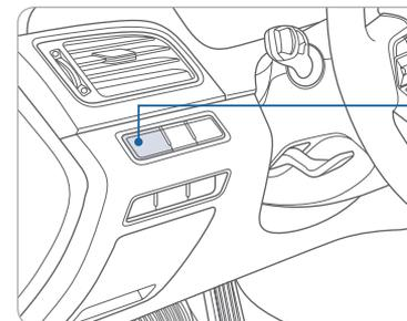
Press - or + to adjust the instrument cluster illumination brightness.
