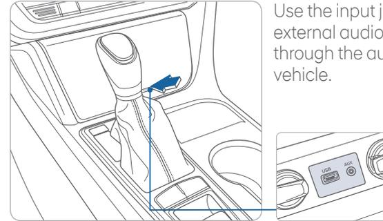
Use the input jack to connect an external audio device and listen to it through the audio system in your vehicle.
