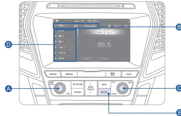
Press POWER button **A** to turn radio on.
