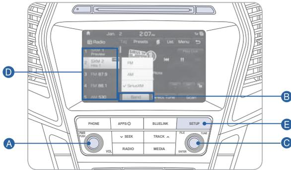
Press POWER button **A** to turn radio on.
