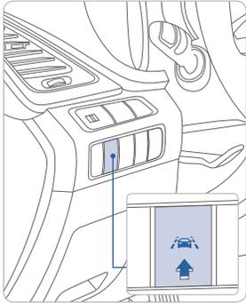
The Lane Departure Warning System detects the lane on the road and warns the driver if the vehicle leaves the lane when the vehicle speed is over 37mph.
