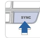
Press the SYNC button to operate the driver and passenger side temperature individually.
