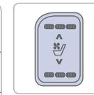
Push the upper portion of the switch to warm or the lower portion to cool.
