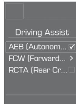
The Autonomous Emergency Braking (AEB) system is designed to detect and monitor the vehicle ahead or detect a pedestrian in the roadway and warn the driver if a collision is imminent.
