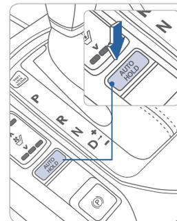
The Auto Hold feature assists in steep hill areas. It holds the brake until the accelerator pedal is pressed.
