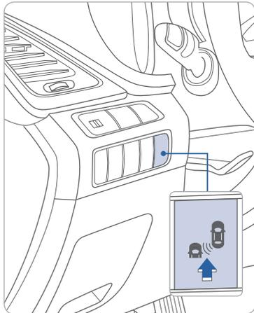
The BSD system sensor senses the rear side territory of the vehicle and provides information to the driver. Press the BSD switch. The indicator will illuminate on the button. If vehicle speed exceeds 9mph the system will activate. Press the switch again to deactivate the system.
