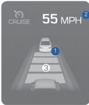
The vehicle to vehicle distance 1 will automatically activate when you set the cruise speed 2.
