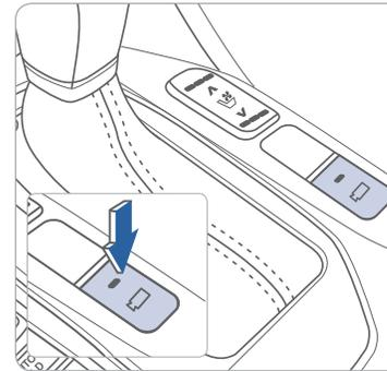
This parking support system displays an all-around view of the vehicle when parking. Press the switch to activate/deactivate the system.
