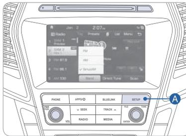
Press SETUP button **A** and press the on-screen CLOCK button. Press on-screen arrows to adjust the time and date.
