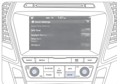
Press SETUP button **A** and press the on-screen CLOCK button. Enable GPS Time and the time and date will automatically set
