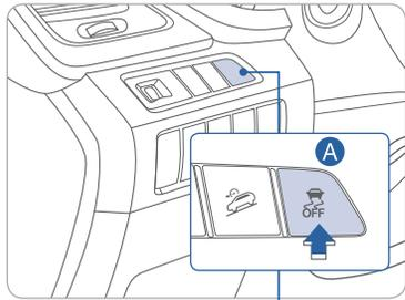
The ESC system is an electronic system designed to help the driver maintain vehicle control under adverse conditions.
