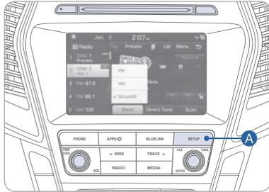
Press SETUP button **A** and press the on-screen CLOCK button. Press on-screen arrows to adjust the time and date.
