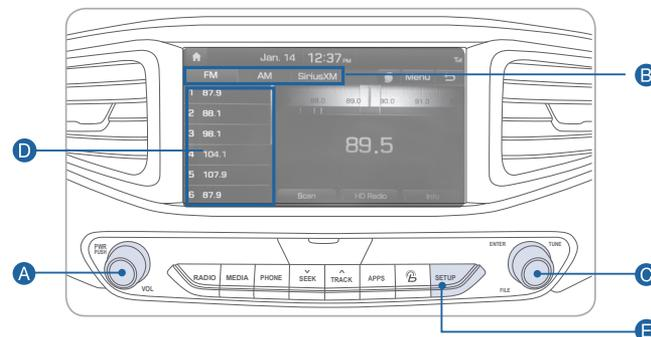
Press POWER button **A** to turn radio on.
