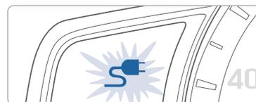
5. Check if the charging cable indicator light of the high voltage battery on the instrument cluster is turned ON.
