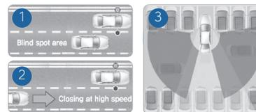
The BSD (Blind Spot Detection) system uses a radar sensor to alert the driver while driving. It monitors the rear area of the vehicle and provides information to the driver.
