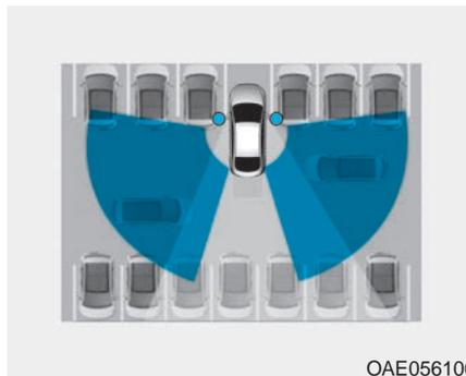
The Rear Cross Traffic Alert function monitors approaching cross traffic from the left and right side of the vehicle when your vehicle is in reverse.
