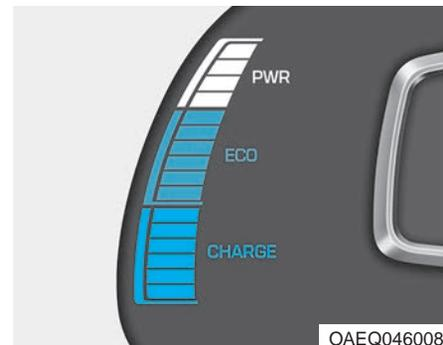
The power gauge indicates whether the current driving condition is fuel efficient or not.
