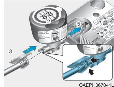
2. Screw the filling hose (3) onto the connector of the sealant bottle (2).
