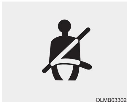
As a reminder to the driver, the seat belt warning light will illuminate and warning chime will sound for approximately 6 seconds each time you place the Engine Start/Stop button to the ON position if the seat belt is unfastened.
