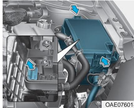
5. Pull the suspected fuse straight out. Use the removal tool provided in the engine compartment fuse panel.
