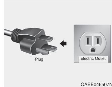
3. Disconnect the plug from the household electric outlet. Do not pull the cable when disconnecting the plug.
