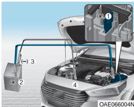
4. Connect the jumper cables in the exact sequence shown in the illustration. First connect one jumper cable to the red, positive (+) jumper terminal of your vehicle (1).
