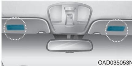
Air bag warning labels, required by the U.S. National Highway Traffic Safety Administration (NHTSA), are attached to alert the driver and passengers of potential risks of the air bag system. Be sure to read all of the information about the air bags that are installed on your vehicle in this Owners Manual.
