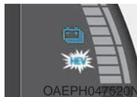
: The high-voltage (hybrid) battery and gasoline engine is used to drive the vehicle.
