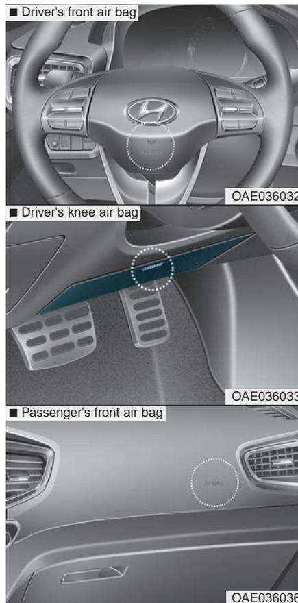
The purpose of the SRS is to provide the vehicle's driver and front passengers with additional protection than that offered by the seat belt system alone. The advanced SRS offers the ability to control the air bag inflation within two levels. A first stage level is provided for moderate-severity impacts. A second stage level is provided for more severe impacts.
