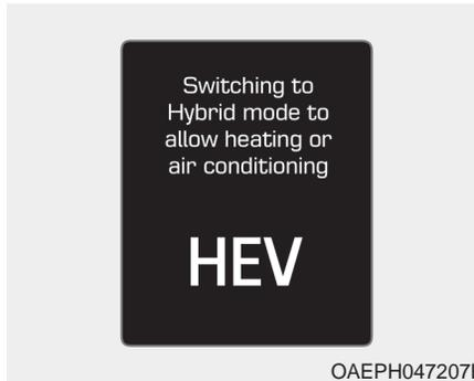
This message is displayed when the vehicle automatically switches to HEV mode to allow heating or air conditioning. It is when the coolant temperature is low (below 7 °F (-14 °C)) and the driver turns on the heating or cooling system.
