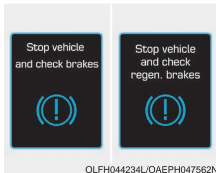
Either message is displayed when a failure occurs in the brake system. In this case, park the vehicle in a safe location and tow your vehicle to the nearest authorized HYUNDAI dealer and have the vehicle inspected.
