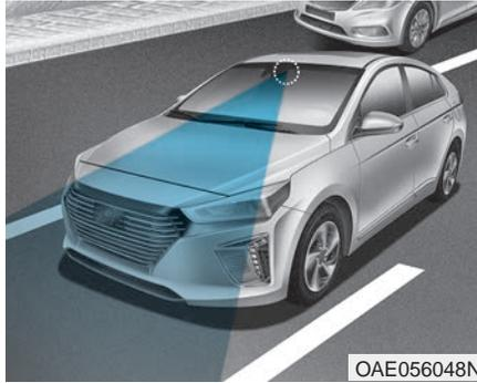
The Lane Keeping Assist System helps detect lane markers on the road with a camera at the front windshield, and assists the driver's steering to help keep the vehicle between lanes.
