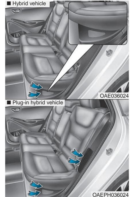
The high-voltage battery cooling duct is located on the left side of the rear seats.
