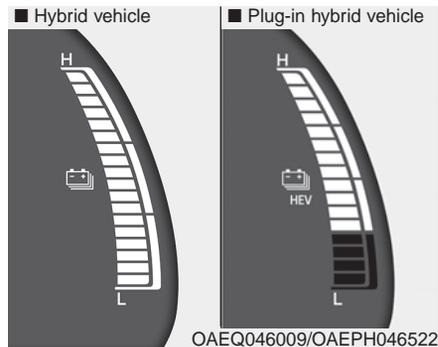
This gauge indicates the remaining hybrid battery power. If the SOC is near the "L (Low)" level, the vehicle automatically operates the engine to charge the battery. However, if the Service Indicator (⚠️) and Malfunction Indicator Lamp (MIL) (🔧) turn on when the SOC gauge is near the "L (Low)" level, have the vehicle be checked by an authorized HYUNDAI dealer.
