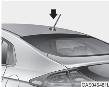
The roof antenna receives both AM and FM broadcast signals. Rotate the roof antenna in a counterclockwise direction to remove it. Rotate it in a clockwise direction to reinstall it.
