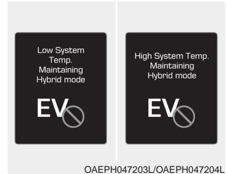
This message is displayed when the temperature of the high-voltage (hybrid) battery is too low or too high. This warning message is to protect the battery and the hybrid system.
