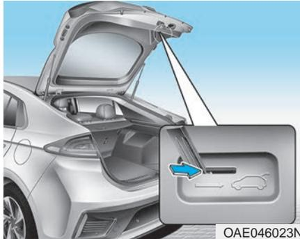
Your vehicle is equipped with an Emergency Liftgate Safety Release lever located inside the liftgate. When someone is inadvertently locked in the luggage compartment, the liftgate can be opened manually from inside the luggage compartment by performing the following steps :
