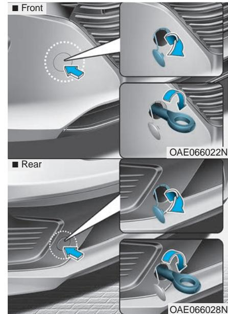
2. Remove the hole cover pressing the lower part of the cover on the front or rear bumper.
