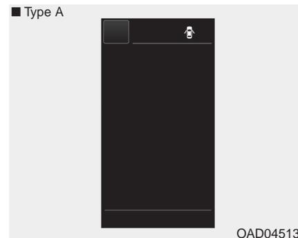
If the door/liftgate open warning is blocked with another warning message, an icon will appear on the top of the LCD display.
