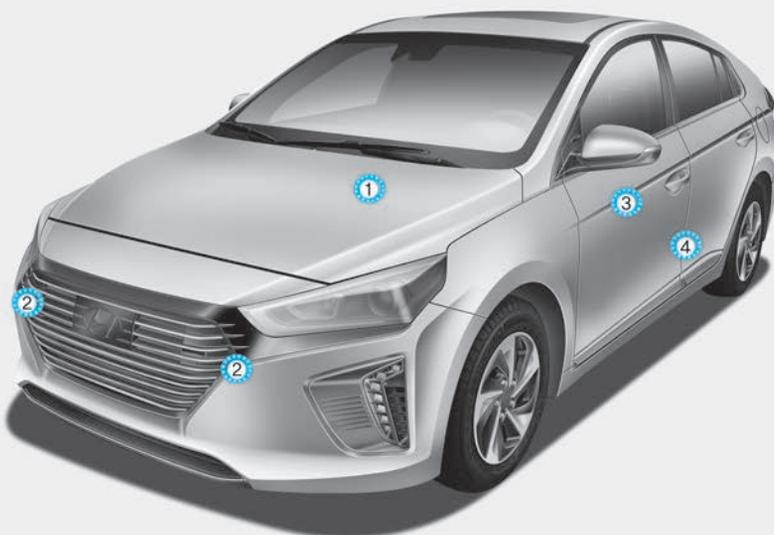
1. SRS control module/Rollover sensor
