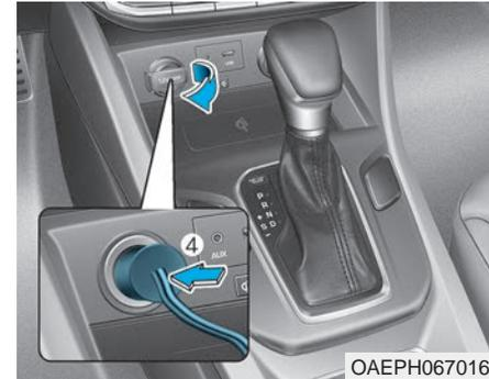
7. Plug the compressor power cord (4) into the vehicle power outlet.
