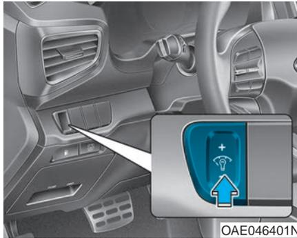
When the vehicle's position lights or headlights are on, press the illumination control button to adjust the brightness of the instrument panel illumination.
