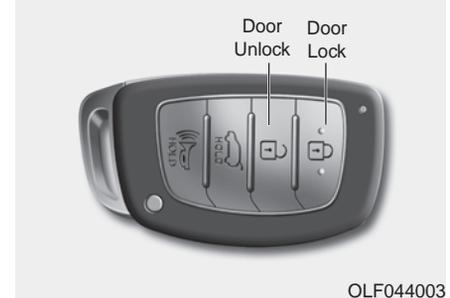
Press the button on the driver's outside door handle while carrying the Smart Key with you or press the Door Unlock button on the Smart Key, the driver's door will unlock. If you press the button on the front passenger's outside door, all doors will unlock.
