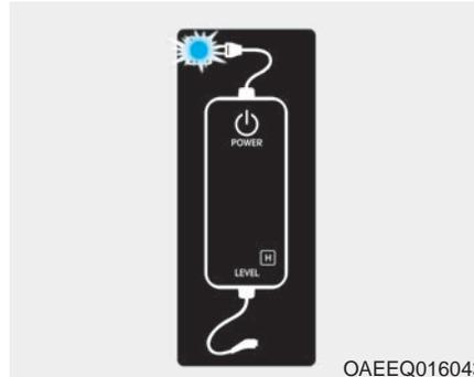
2. Check if the power lamp (green) illuminates on the control box.
