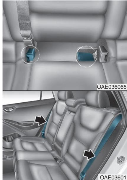
3. Insert the rear seat belt buckle in the pocket between the rear seatback and cushion.
