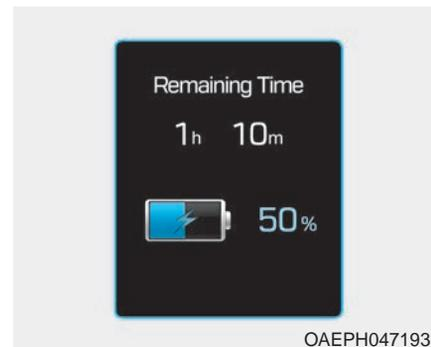
10. After charging has started, the estimated charging time is displayed on the instrument cluster for about 1 minute. If you open the driver seat door while charging, the estimated charging time is also displayed on the instrument cluster for about 1 minute.
