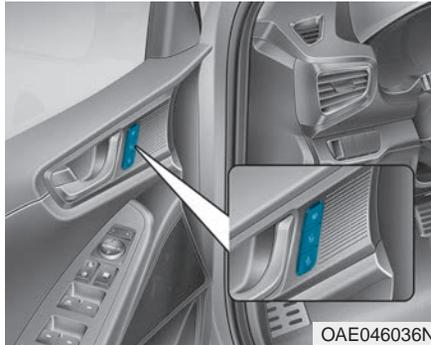
The Driver Position Memory System is provided to store and recall the following memory settings with a simple button operation.
