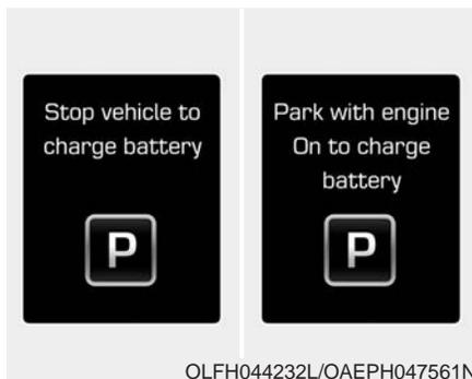
Either message is displayed when the hybrid battery power (SOC) level is low.
