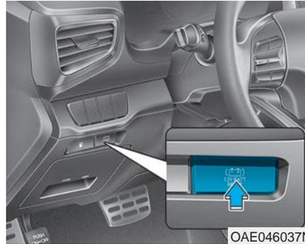
1. Press the 12V Battery Reset switch to reconnect the 12V battery.
