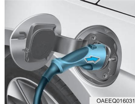
5. Hold the charging connector handle and connect it to the vehicle normal charging inlet. Push the connector until you hear a "clicking" sound. If the charging connector and charging terminal are not connected properly, this may cause a fire.
