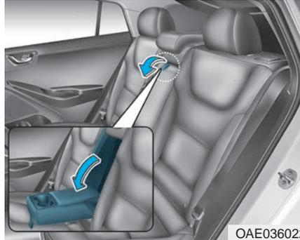
The armrest is located in the center of the rear seat. Use the strap in the center of the armrest to pull it down.
