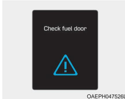
This message is displayed when the vehicle is driven with the fuel filler door opened. Close the fuel filler door and then start driving.
