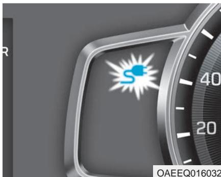
9. Check if the charging indicator light of the high voltage battery on the instrument cluster is turned ON. Charging is not done when the charging indicator lamp is OFF.
