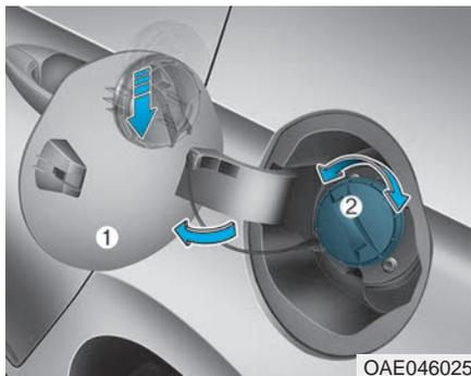
3. Pull the fuel filler door (1) out to fully open.
