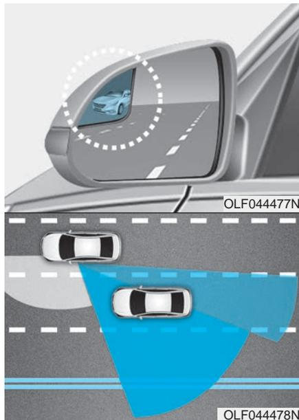
The Blind Spot Mirror (BSM) is a supplemental mirror that reduces the driver's blind spot by showing the rear side area of the vehicle. The blind spot mirror is equipped on the left-hand side view mirror.
