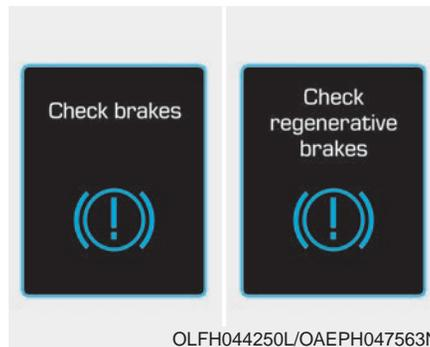
Either message is displayed when the brake performance is low or the regenerative brake does not work properly due to a failure in the brake system.
