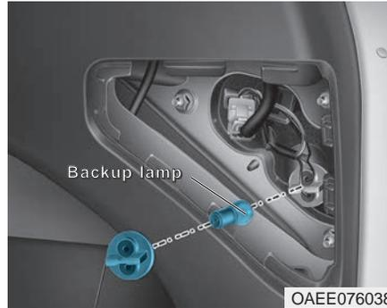
3. Remove the bulb by pulling it straight out.
