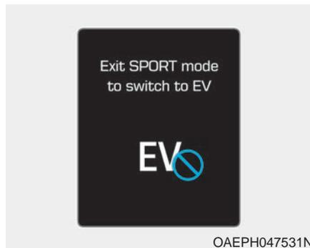
This message is displayed when [EV/HEV] button is pressed but it is impossible to switch from the HEV mode to EV mode because the SPORT mode is engaged.
