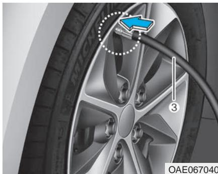
3. Connect the other end of the filling hose (3) directly into the tire valve.
