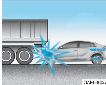
Just before impact, drivers often brake heavily. Such heavy braking lowers the front portion of the vehicle causing it to "ride" under a vehicle with a higher ground clearance. Air bags may not inflate in this "under-ride" situation because deceleration forces that are detected by sensors may be significantly reduced by such "override" collisions.
