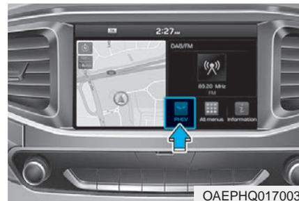
Press [PHEV] on the [Home] screen or the [All menus] screen and the menus related to plug-in hybrid ([ECO Driving], [Energy Information], [EV Range], [Charging Settings], [Charging Stations], [Gas Stations]) are displayed.
