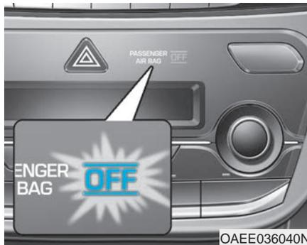
Your vehicle is equipped with an Occupant Classification System (OCS) in the front passenger's seat.
