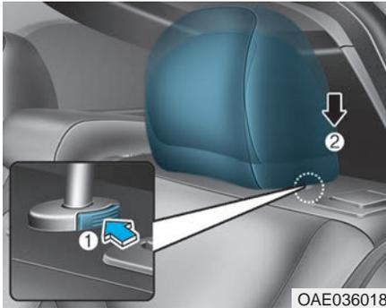
2. Lower the rear head restraints to the lowest position by pushing and holding the release button (1) and pushing down on the headrest (2).
