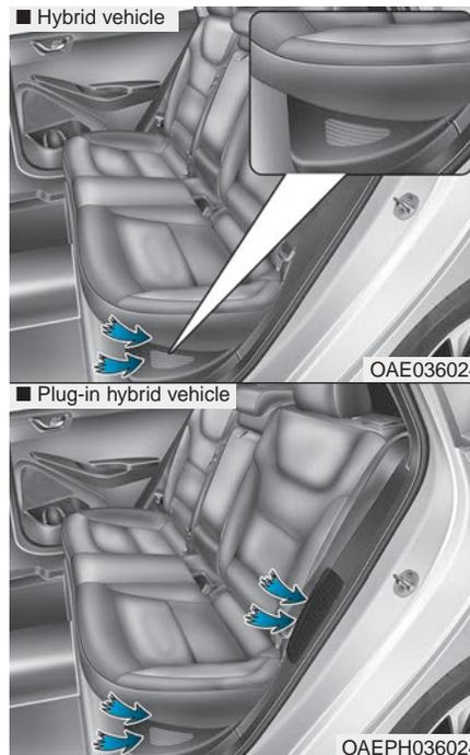
When the high voltage battery cooling duct is blocked, the high voltage battery may be overheated. Do not obstruct the cooling duct with any other objects.
