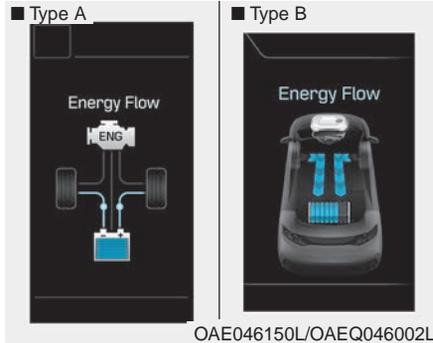
The high-voltage battery is charged up by the regenerative brake system.
