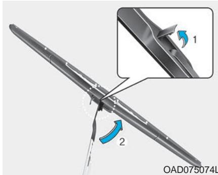
2. Lift up the wiper blade clip (1). Then lift up the wiper blade (2).
