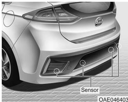
The Rear Parking Assist System assists the driver during reverse movement of the vehicle by chiming if any object is sensed within approximately 50 in (120 cm) behind the vehicle.
