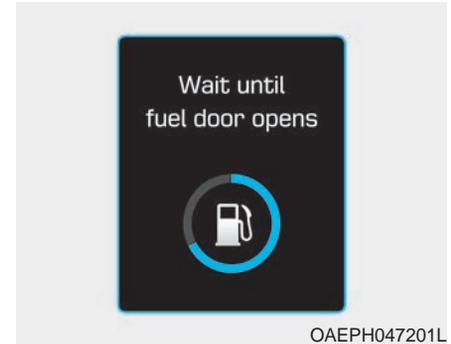
This message is displayed when you attempt to open the fuel filler door with the fuel tank pressurized. Wait until the fuel tank is depressurized.
