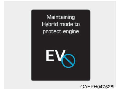
This message is displayed when the [EV/HEV] button is pressed but it is impossible to switch from the HEV mode to EV mode due to engine lubrication.
