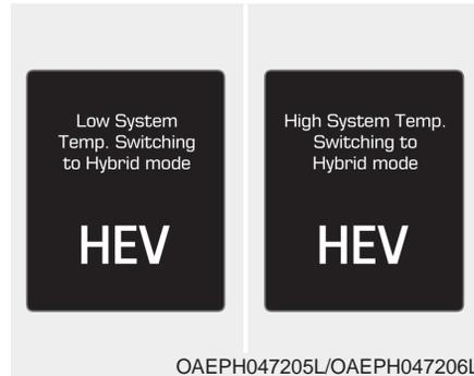
This message is displayed when the temperature of the high-voltage (hybrid) battery is too low or high. This warning message is to protect the battery and the hybrid system.
