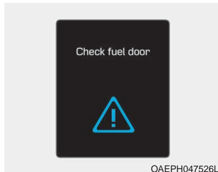
This message is displayed when there is a problem with the fuel filler door. Such as, when the fuel filler door does not open after 20 seconds at freezing temperature.
