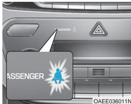
As a reminder to the front passenger, the front passenger's seat belt warning lights will illuminate for approximately 6 seconds each time you place the Engine Start/Stop button to the ON position regardless of belt fastening.
