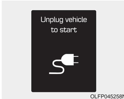
This message is displayed when you start the engine without unplugging the charging cable. Unplug the charging cable, and then start the vehicle.
