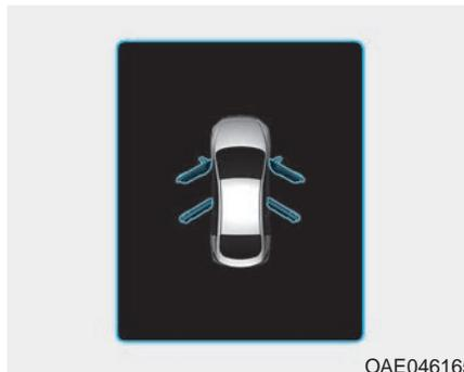
This warning is displayed indicating which door, or hood, or liftgate is open.
