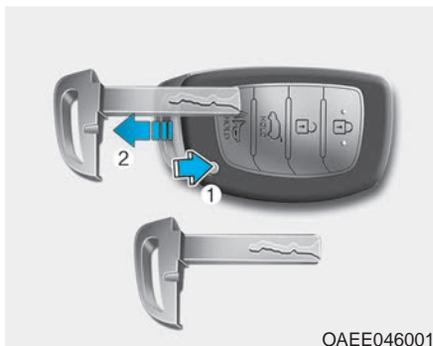
Press and hold the release button (1) and remove the mechanical key (2). Insert the mechanical key into the key hole on the door.
