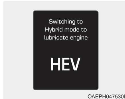
This message is displayed when the vehicle is automatically switched to the HEV mode to lubricate engine while the Engine Start/Stop button is in the ON position.
