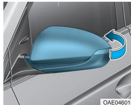
To fold the side view mirrors, grasp the housing of the mirror and then fold it toward the rear of the vehicle.
