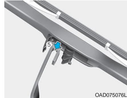
4. Remove the wiper blade from the wiper arm (5).
