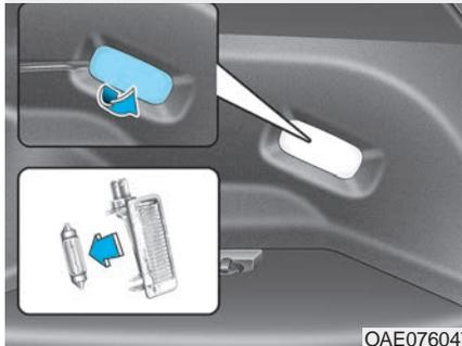
1. Using a flat-blade screwdriver, gently pry the lens from the interior lamp housing.
