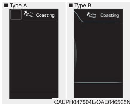
The coasting guide function informs the driver when to take the foot off from the accelerator by anticipating a decelerating event\* based on the analysis of driving routes and road conditions of the navigation. It encourages the driver to remove foot from the pedal and allow coasting down the road with EV motor only. This helps prevent unnecessary fuel consumption and increases fuel efficiency.
