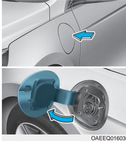
3. Press center edge of the charging door to open the charging door.
