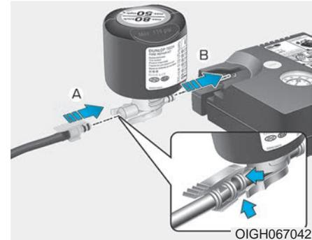
2. Connect the filling hose (3) to the sealant bottle (2) in the direction of (A) and connect the sealant bottle (2) to the compressor (5) in the direction of (B).
