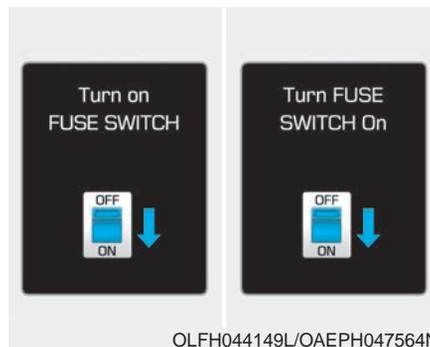
Either message is displayed if the fuse switch located on the fuse box under the steering wheel is OFF.
