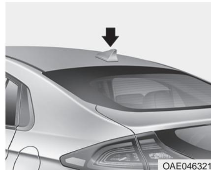
The shark fin antenna will receive the transmit data (example: AM/FM, SXM signal, GPS, LTE).
