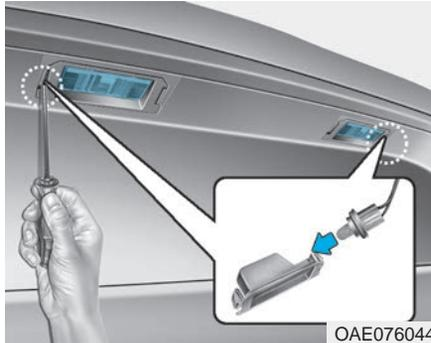
1. Using a flat-blade screwdriver, gently pry the lens cover from the lamp housing.
