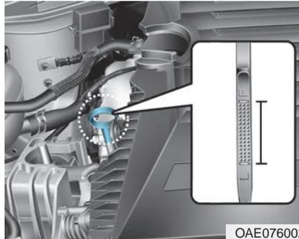
6. Pull the dipstick out again and check the level. The level should be between F (Full) and L (Low).
