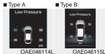
When the tire pressure monitoring system warning indicators are illuminated and the warning message is displayed on the cluster LCD display, one or more of your tires is significantly under-inflated. The LCD position indicator will indicate which tire is significantly under-inflated by illuminating the corresponding position light.
