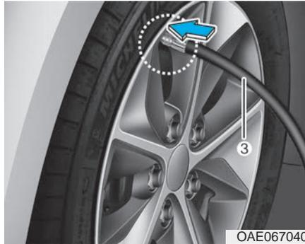
5. Unscrew the valve cap from the valve of the defective wheel and screw the filling hose (3) of the sealant bottle onto the valve.
