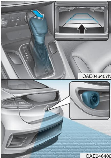
The Rear View Camera will activate when the vehicle is in the ready (🚗) mode and when you shift to the R (Reverse) position.
