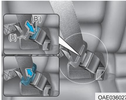
2. Pull the tongue plate (B) and insert it into the buckle (B') until an audible "click" is heard, indicating the latch is locked. Make sure the belt is not twisted.
