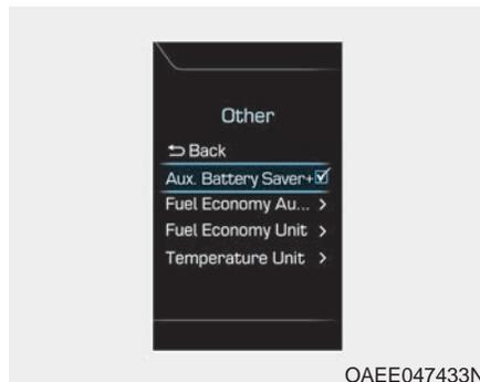
The driver can activate the Aux. Battery Saver+ function by placing the Engine Start/Stop button to the ON position and by selecting:
