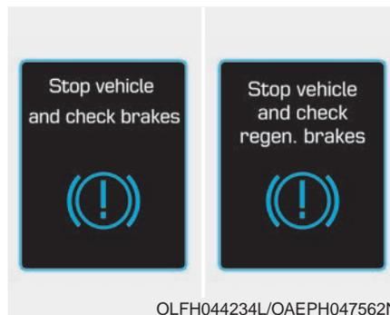
Either message is displayed when a failure occurs in the brake system.
