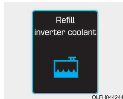
This message is displayed when the inverter coolant is nearly empty.
