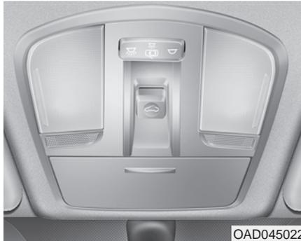
If your vehicle is equipped with a sunroof, you can slide or tilt your sunroof with the sunroof control switch located on the overhead console.
