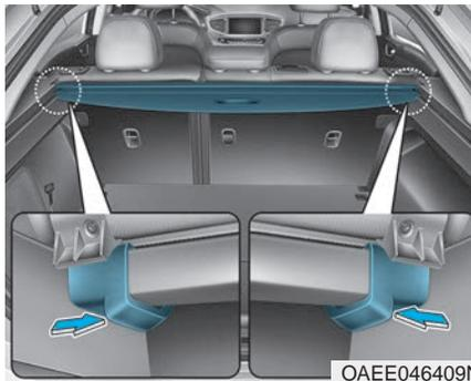
1. Push out the lower part of guide pins in both sides.
