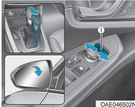
When you move the shift lever to the R (Reverse) position, the side view mirror(s) will rotate downwards to aid with driving in reverse. The position of the side view mirror switch (1) determines whether or not the mirrors will move:
