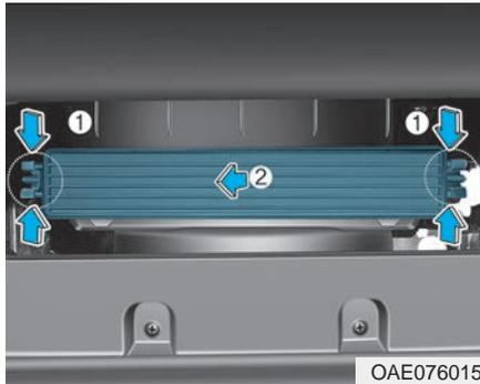
3. Press and hold the lock (1) on both sides of the cover.
