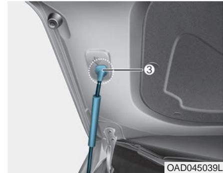
4. Pull out the support rod and hold the hood open with the support rod (3).
