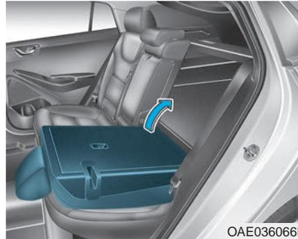
7. To use the rear seat, lift and unfold the seatback to the upright position. Push the seatback firmly until it clicks into place. Make sure the seatback is locked in place.
