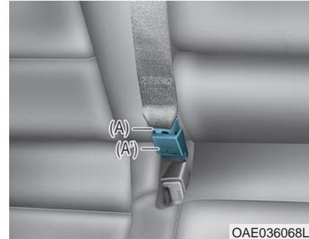
1. Insert the tongue plate (A) into the buckle (A') until an audible "click" is heard, indicating the latch is locked. Make sure the belt is not twisted.
