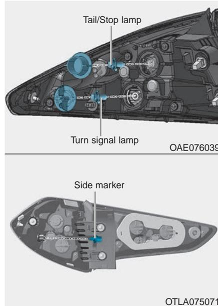
5. Remove the socket from the assembly by turning the socket counterclockwise until the tabs on the socket align with the slots on the assembly.
