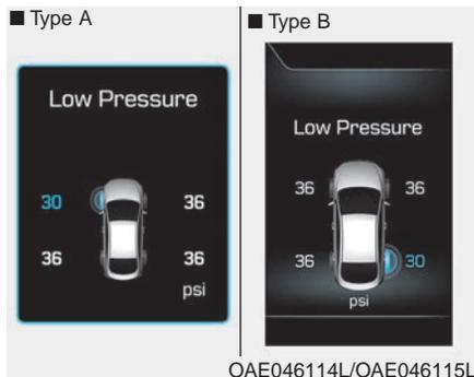
This message is displayed if the tire pressure is low. The corresponding tire on the vehicle will be illuminated.
