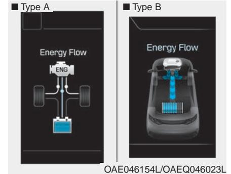
The engine is simultaneously used to drive the vehicle and to charge up the high-voltage battery.
