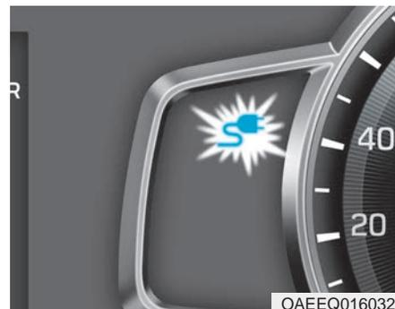
7. Check if the charging indicator light of the high voltage battery on the instrument cluster is turned ON. Charging is not done when the charging indicator lamp is OFF.
