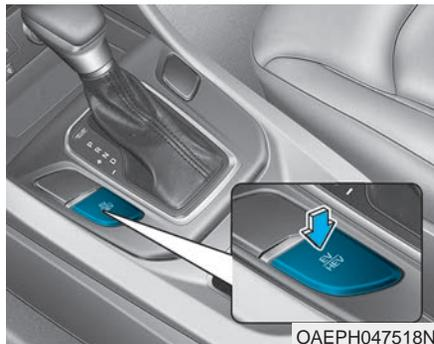
Pressing the [EV/HEV] button changes the plug-in hybrid system modes, between Electric (CD) mode and Hybrid (CS) mode.
