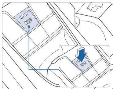
You can select the drive mode according to your preference or the road condition. The system initializes to the NORMAL mode (except ECO mode) after the vehicle is restarted. Each time you press the button, the drive mode is changed as follows:
