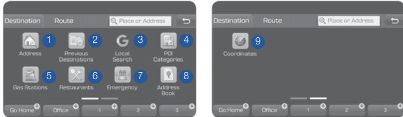
Press **[NAV]** button in the navigation head unit, and finds a destination by using the **[Destination]** menu.
