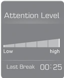
The Driver Attention Alert (DAA) system displays the condition of the driver's fatigue level and inattentive driving practices. The DAA system monitors the lane markers and driver's inputs to the steering wheel, accelerator pedal and brake pedal.
