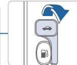
Pull the trunk release lever in the vehicle.
