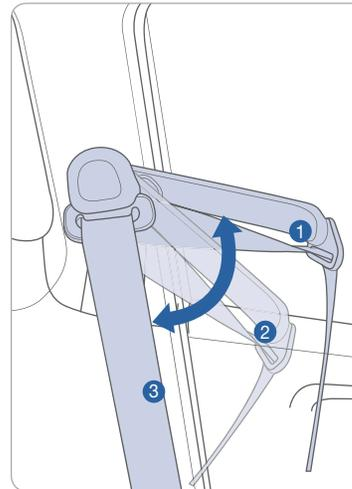
Set the belt extension guide to one of the 3 positions when using the seat belt.
