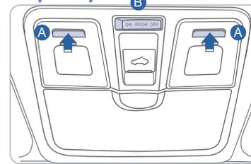
Push the lens **A** to turn the map lamp on or off.
