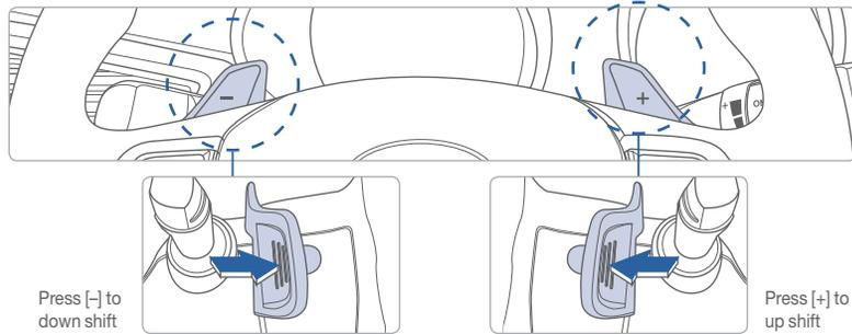
The paddle shifters operate when the shift lever is in the D position or the Sport Mode.
