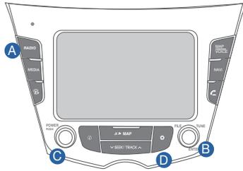
Press POWER button **C** to turn radio on.
