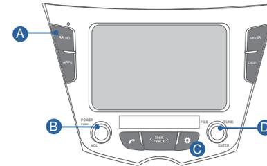
Press POWER button **B** to turn radio on.
