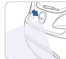
When the gear shift lever is shifted into reverse (R), the rearview camera displays the area behind the vehicle.
