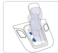
Shift the lever from D into the manual gate to activate manual shift mode. Manual shift mode is a recalibrated automatic mode that will hold gears longer and downshift at higher RPM for a more dynamic driving style.
