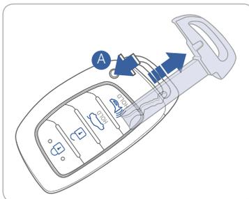
**Removing the mechanical key**
