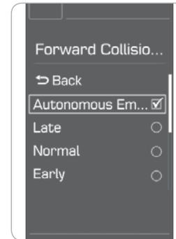
The Autonomous Emergency Braking (AEB) system is designed to detect and monitor the vehicle ahead or detect a pedestrian in the roadway through radar signals and camera recognition to warn the driver that a collision is imminent, and if necessary, apply emergency braking.
