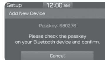
3. Confirm the 6-digit passkey displayed on the audio screen and the Bluetooth device are identical.
