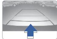
When the shift lever is moved to R(Reverse), the rear view camera displays the area behind the vehicle.
