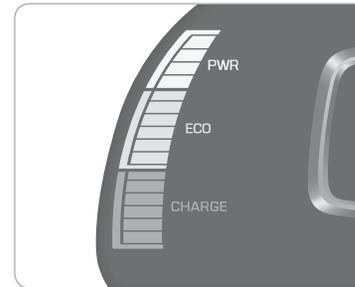
The power gauge indicates whether the current driving condition is fuel efficient or not.
