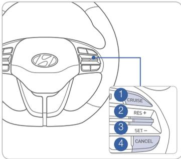
The Cruise Control system allows you to program the vehicle to maintain a constant speed without depressing the accelerator pedal.
