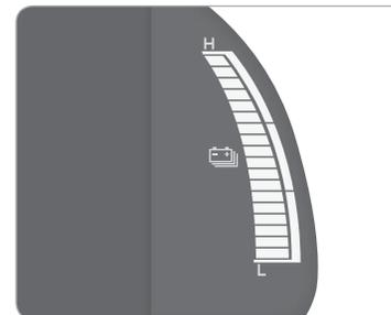
This gauge indicates the remaining hybrid battery power. If the SOC is near the "L (Low)" level, the vehicle automatically operates the engine to charge the battery.
