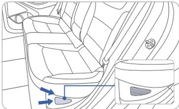
The high voltage battery cooling duct is located on the left side of the rear seats.
