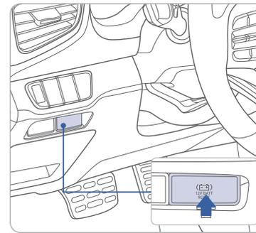
This vehicle does not have a replaceable 12V flooded lead acid battery. The 12V battery is integrated into the lithium high voltage battery assembly. It is automatically protected against vehicle current draw when a minimum level of 12.8V 10% SOC level is reached. The 12V Battery Reset Switch has to be activated in order to start the vehicle. This should negate the need to jump start the car.
