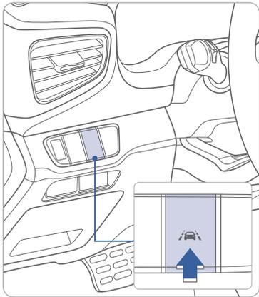
The Lane Departure Warning System detects the lane on the road and warns the driver if the vehicle leaves the lane. The system operates when the vehicle speed is over 40 mph.
