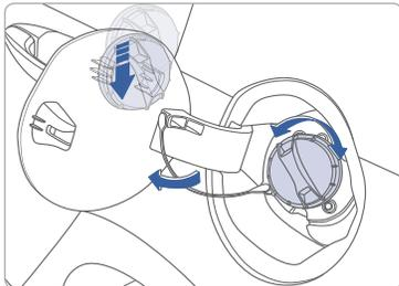
2. Remove the fuel tank cap.
