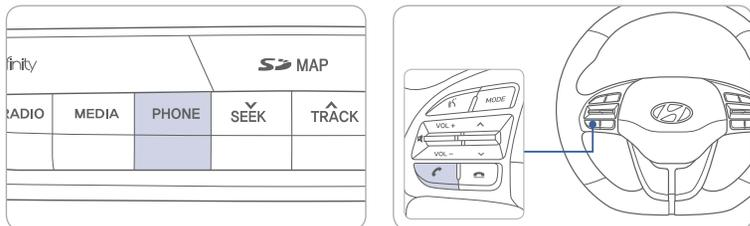
1. Press the PHONE button in the head unit or CALL button in the steering wheel remote control.
