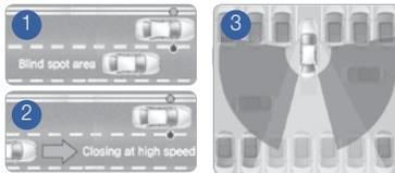
The BSD (Blind Spot Detection) system uses a radar sensor to alert the driver while driving. It monitors the rear area of the vehicle and provides information to the driver.
