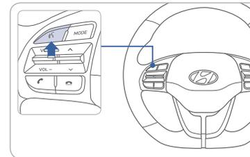
Press 🗣️ button on the steering wheel control to activate voice recognition.
