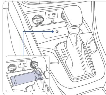
There is a wireless cellular phone charging system inside the front console. The system operates with all doors closed, and the Engine Start/Stop button in the ACC/ON/START position.
