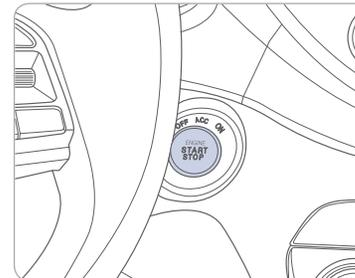
With the ignition OFF and foot OFF of the brake pedal, press the Engine Start / Stop button.
