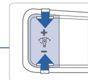
Press + or - to adjust the illumination brightness of the instrument cluster.
