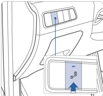
The BSD and LCA systems will activate once the vehicle speed exceeds 20 mph. The RCTA system activates in reverse gear under 6 mph.
