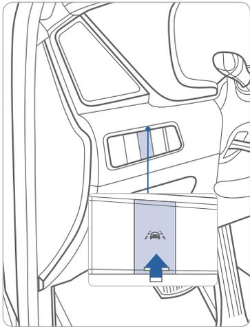
The Lane Departure Warning System detects the lane on the road and warns the driver if the vehicle leaves the lane when the vehicle speed is over 40mph.
