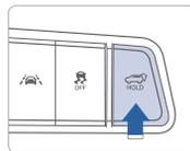
Press the power liftgate button in the vehicle.
