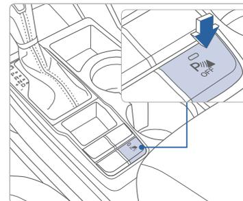
The rear parking assist system assists the driver during the reverse movement of the vehicle by chiming if any object is sensed within a distance of 47 inches behind the vehicle.
