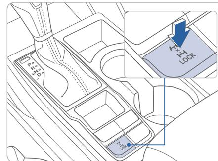
During off-road or inclement weather conditions, press the AWD LOCK switch to drive in full-time AWD. This will divide the power between the front and rear wheels (only when the vehicle speed is under 19 mph). The AWD LOCK indicator light on the instrument cluster will illuminate.
