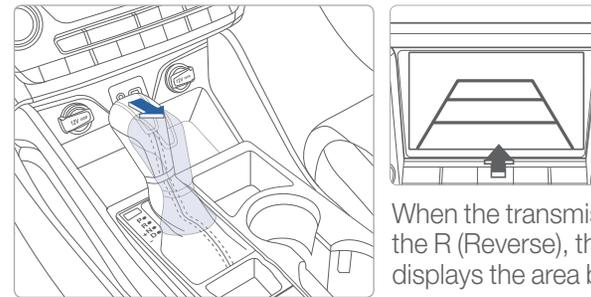
When the transmission is shifted into the R (Reverse), the rearview camera displays the area behind the vehicle.
