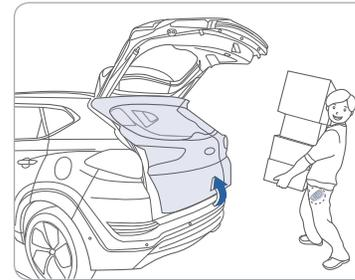
Approach the vehicle 15 seconds after all the doors are closed and locked with the smart key. The liftgate will open automatically.
