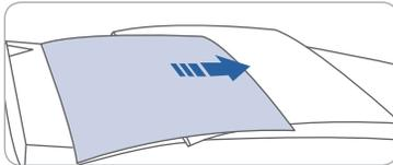
Pull the sunroof control lever backward to the second detent position. First the sunshade will open and then the sunroof will open automatically.
