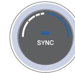
Press the SYNC button ON to operate the driver and passenger temperature equally. Press the SYNC button OFF to operate the driver and passenger side temperature individually. The button indicator will turn off.
