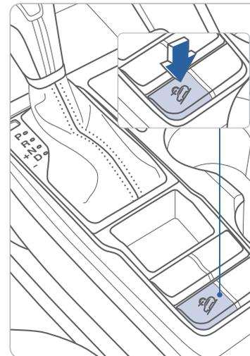
The Downhill Brake Control (DBC) helps the driver maintain a slow speed on a steep downhill without depressing the brake pedal. The system automatically applies the brakes to keep the vehicle speed under 5 mph.
