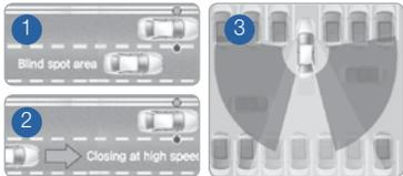
The BSD (Blind Spot Detection) system uses a radar sensor to alert the driver while driving. The system monitors the rear area of the vehicle and provides information to the driver. The system incorporates the following functions:
