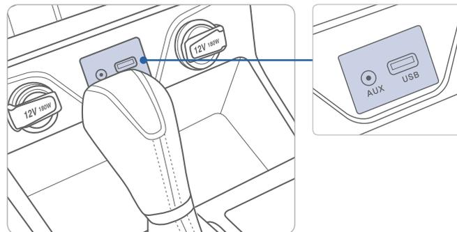
Use the input jack to connect an external audio device and listen to it through the audio system in your vehicle.
