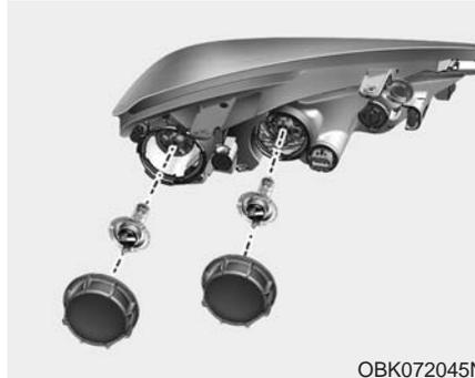
8. Remove the headlight bulb cover by turning it counter clockwise.
