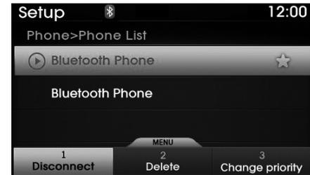
From the paired phone list, select the currently connected device and select the **Disconnect** button.
