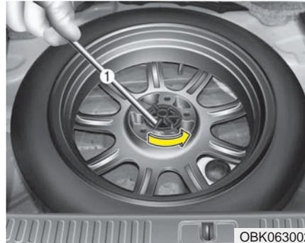
※ If it is hard to loosen the tire hold-down wing bolt by a hand, you can loosen it easily using the Jack handle.
