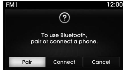
If *Bluetooth*<sup>®</sup> Wireless Technology devices are paired but none are currently connected, pressing the **PHONE** key or the
