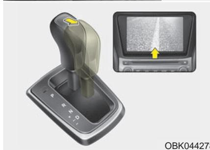
The rear camera display will activate when the back-up light is ON with the ignition switch ON and the shift lever in the R (Reverse) position.
