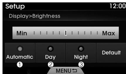
Use the **TUNE** knob to adjust the screen brightness or set the Brightness on Automatic, Daylight, or Night mode.
