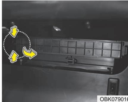
3. Remove the climate control air filter case pulling out both sides of the cover.
