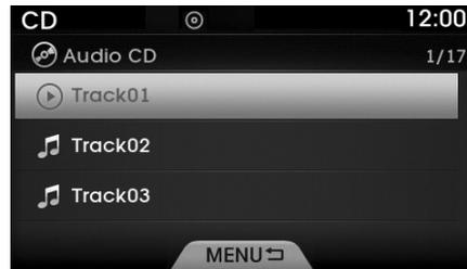
Turn the **TUNE** knob to search for the desired track and press the **TUNE** knob to select.
