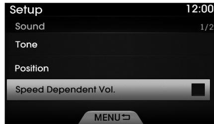
The volume level is controlled automatically according to the vehicle speed.
