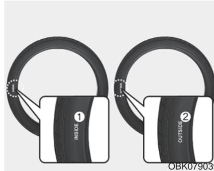
Your vehicle is equipped with asymmetric tires, when you replace the tires, check the inside and outside of the tire.
