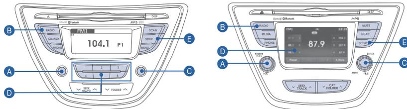
Press POWER button **A** to turn radio on.
