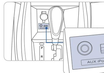
Use the jack to connect an external audio device and listen to it through the audio system speakers in your vehicle.
