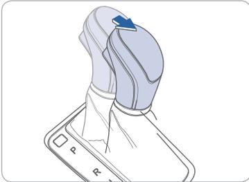
The rearview camera will activate when the ignition switch is turned ON and the shift lever is in the R (Reverse) position.
