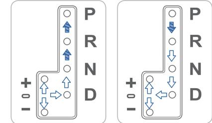
(➔) : Depress the brake pedal when shifting.
