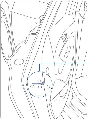
Insert a key into the hole and turn it to the following positions:
