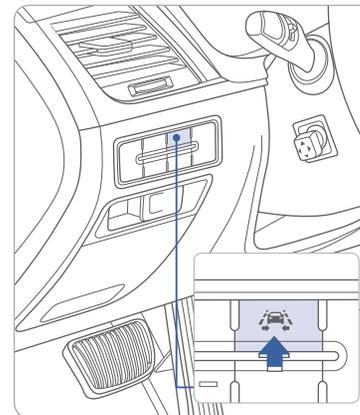
The Lane Keeping Assist System detects lane markers on the road, and assists the driver's steering to help keep the vehicle between lanes.
