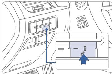
The BSD (Blind spot detection) system uses a radar sensor to alert the driver while driving. It senses the rear side territory of the vehicle and provides information to the driver.
