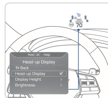
The head up display is a transparent display which projects a shadow of selected information of the instrument cluster and navigation on the windshield glass.
