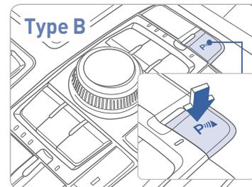
If you move the shift lever to R with the engine start/stop button in ON and the parking assist system in OFF, the parking assist system will turn ON automatically. The system will automatically turn off when vehicle is driven forward at a speed above 6 mph.
