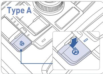
Pressing the heated steering wheel button warms the steering wheel. The indicator on the button is illuminated.
