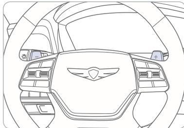
The Paddle shifter is available when the shift lever is in the D position or the sport mode.
