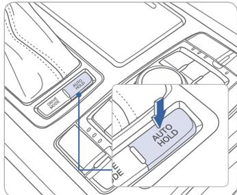
The Auto Hold feature assists in steep hill areas. It holds the brake until the accelerator pedal is pressed.
