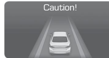
The Automatic Emergency Braking (AEB) helps avoid accidents by identifying critical situations early and warning the driver.
