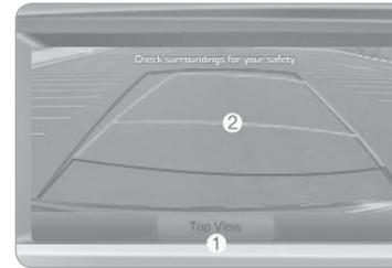
The parking guide system will activate when the back-up light is ON and the shift lever in the R (Reverse) position.
