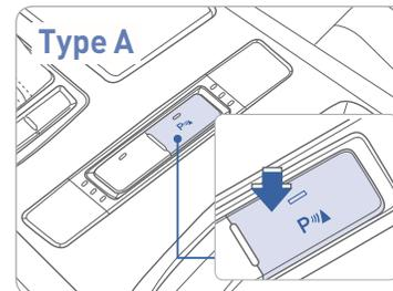
The parking assist system assists the driver during movement of the vehicle by chiming if any object is sensed within the distance of 39.5 inches in front and 47.2 inches in behind the vehicle.
