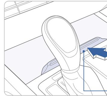
Use the input jack to connect an external audio device and listen to it through the audio system in your vehicle.
