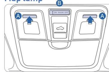
Push the lens **A** to turn the map lamp on or off.
