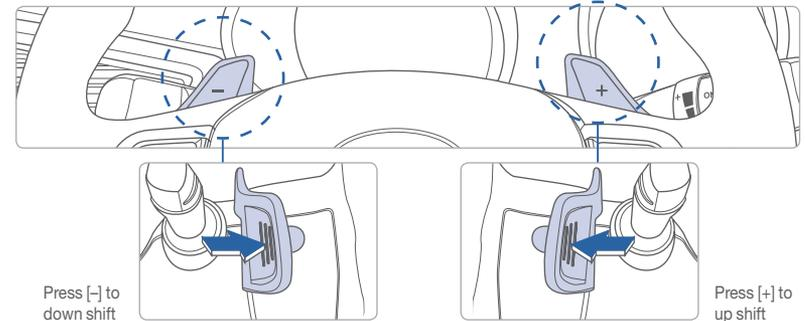
The paddle shifters operate when the shift lever is in the D position or the Sport Mode.
