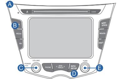
Press POWER button **C** to turn radio on.
