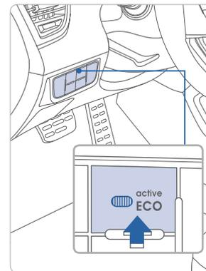
Active ECO System helps improve fuel efficiency by controlling the engine and transmission.
