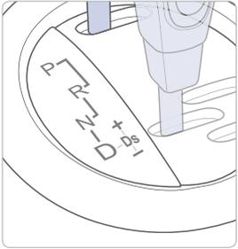
Shift lever from D to DS to activate Sport mode. Sport mode is a recalibrated automatic mode that will hold gears longer and downshift at higher RPM for a more dynamic driving style. If you use the paddle shifters (or [+] or [-]) to enter the Sport Mode, you will stay in Sport Mode until the shift lever is returned to Drive, giving you full manual control.
