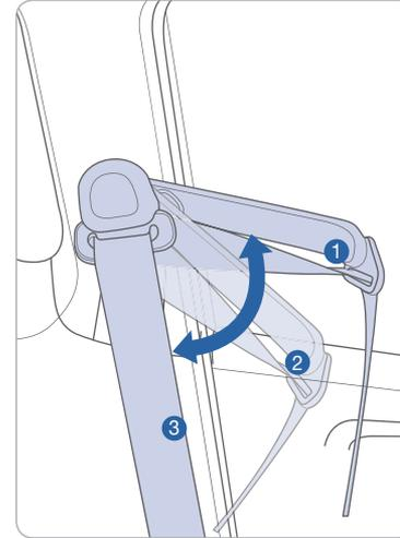
Set the belt extension guide to one of the 3 positions when using the seat belt.
