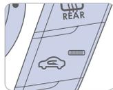
This is used to select outside (fresh) air position or recirculated air position.
