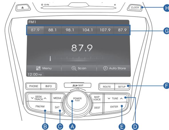
Press POWER button **A** to turn radio on.
