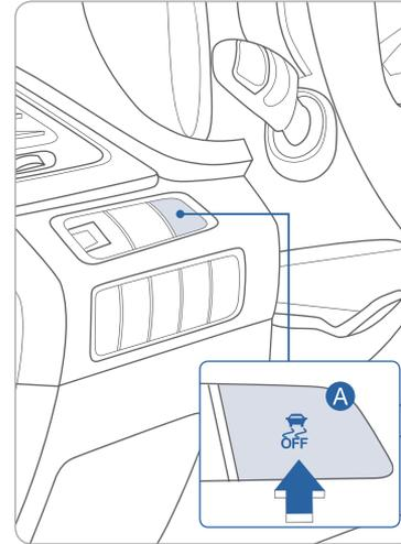
The ESC system is an electronic system designed to help the driver maintain vehicle control under adverse conditions.
