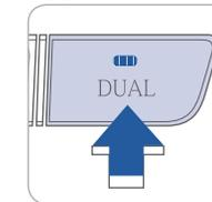
Press the DUAL button to operate the driver and passenger side temperature individually.
