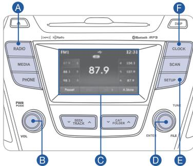
Press POWER button **B** to turn radio on.
