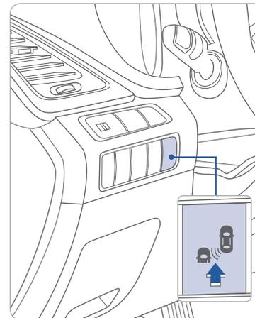
The BSD system sensor senses the rear side territory of the vehicle and provides information to the driver. Press the BSD switch. If vehicle speed exceeds 9.3mph the system will activate. Press the switch again to deactivate the system.
