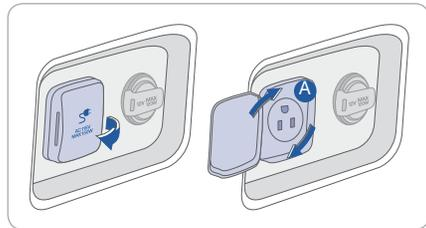
1. Dashboard button must be switched on to use cargo area AC115V plug. Engine should be running when AC 115V plug is in use.
