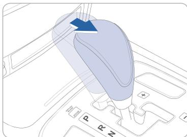
The rearview camera will activate when the ignition switch is ON and the shift lever is in the R (Reverse) position.
