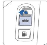
Pull trunk lid release to open trunk from inside of vehicle.
