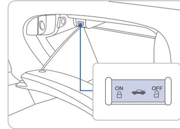
The trunk lock button is used to prevent unauthorized access to the trunk.
