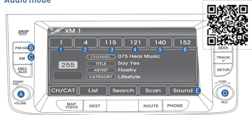
Press **POWER** button **A** to turn radio on.
