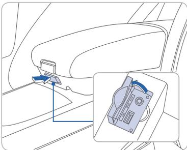
Use the jack to connect an external audio device and listen to it through the audio system in your vehicle.
