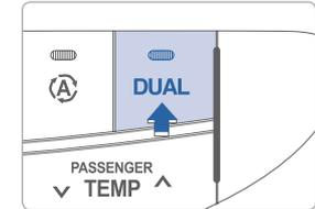
Press the DUAL button to operate the driver and passenger side temperature individually.
