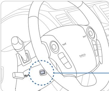
Pressing the heated steering wheel button warms the steering wheel. The indicator on the button is illuminated.
