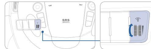
Rotate the illumination control knob to adjust the brightness.
